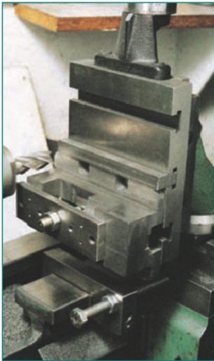
12. Machining the first side and vice fixing web.
