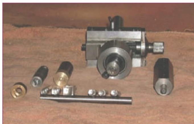
5. Method 2 Wobble tool fitted to boring head, also showing cutters and hexagon jig.
