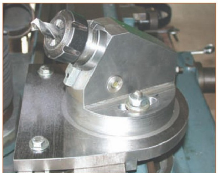
7. The baseplate now modified for the J & S 310. The jig is using the ER holder for a parallel drill. Note the base now fixes against the location strip underneath.
