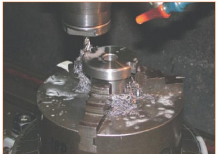
3. Milling slots in holder
