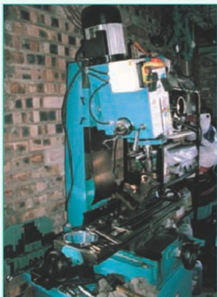
1. Compound angle set up for drilling steam passages.
