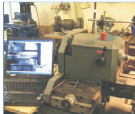
7. Webcam and laptop arranged for a turning application.
