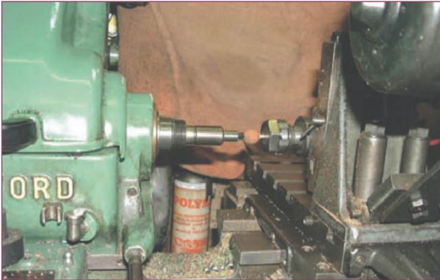
6. Grinding the end of the tool using a spherical stone.
