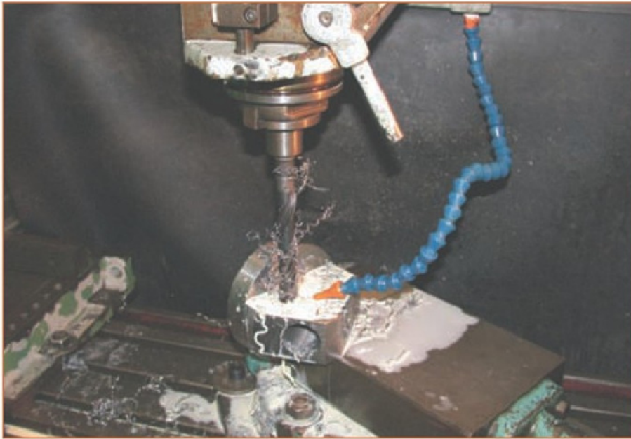
1. Cross drilling the main body for clamp location.
