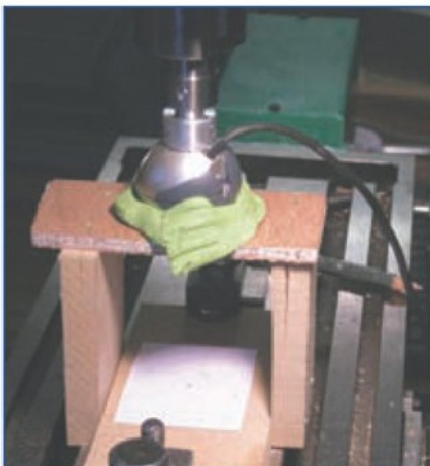
3. Set up to centre Trust camera.
