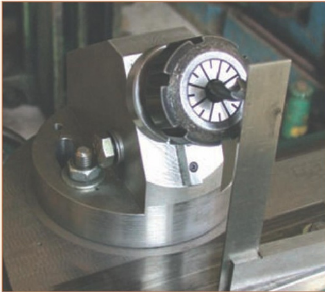
8. Setting a drill parallel to the holder with ER collets
