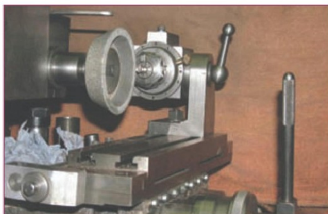
4. Grinding a cutter on the Stent.
