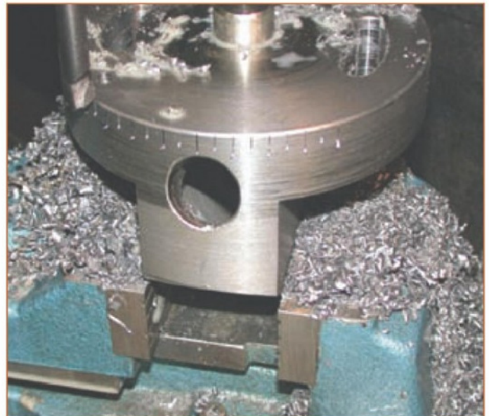
5. Milling the arc slots and Graduating the Main Body, the vice is mounted on a rotary table
