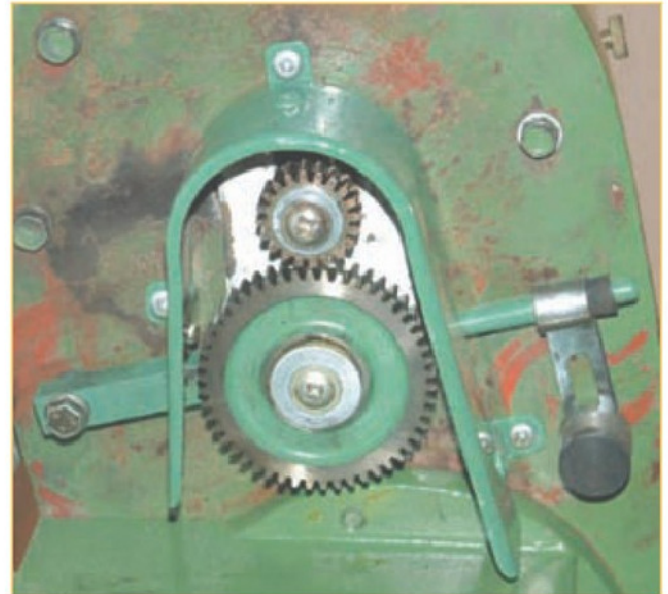
3. View of the back-gear from beneath, showing the lever which carries the bearing in which it runs, and the pivot-bolt at the end. The white plate serves to steady the assembly against the motor mounting plate. The black knob on the right clamps the gear in position, engaged or disengaged.
