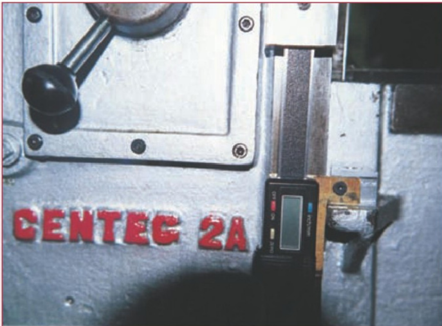
13. Scale fitted to Z axis of Centec mill.
