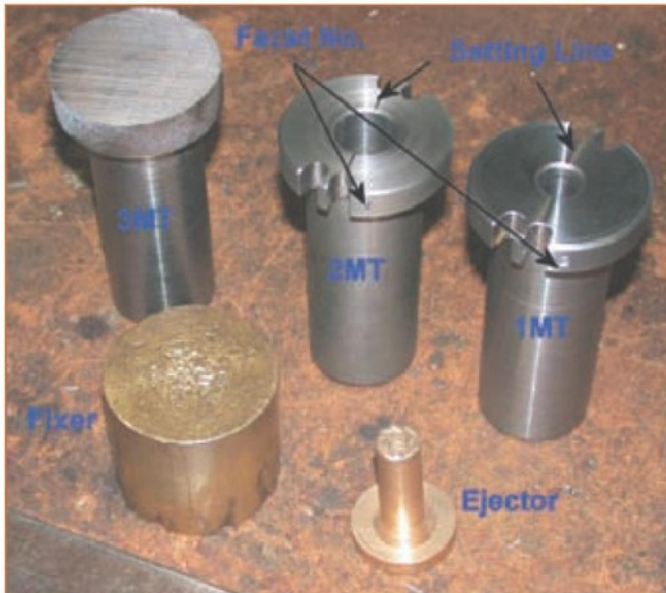
4. Morse taper holders, ejector, and fixer.
