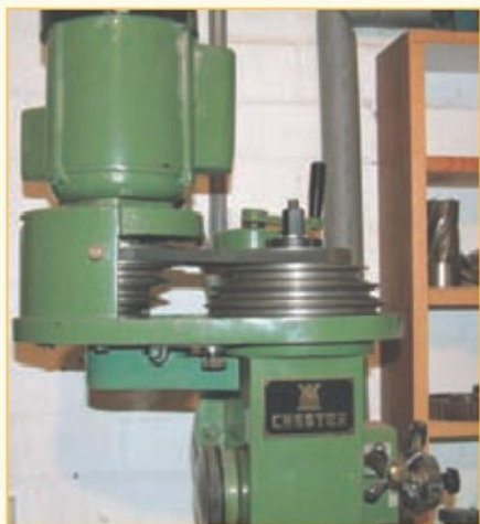
1. General view of the mill-drill, with the cover off to show the arrangement of the belt-drive. The cover of the back gear modification can be seen beneath the motor support plate.
