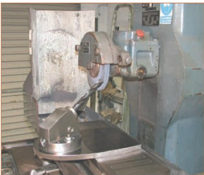
6. The jig in test use. Note the end face locates on the table fence for alignment.
