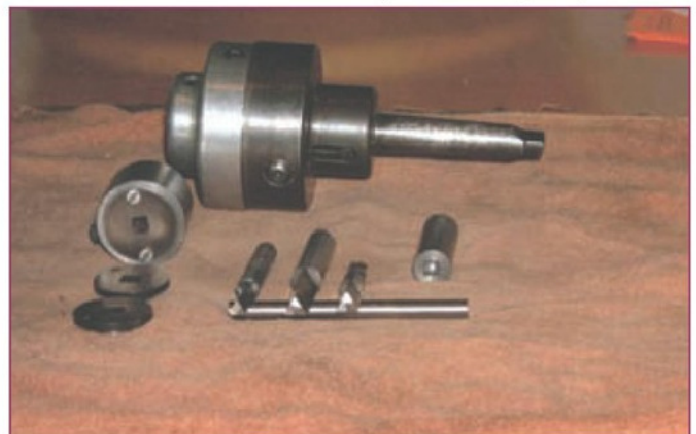
3. Floating chuck with drill bits, guide plate and holder.
