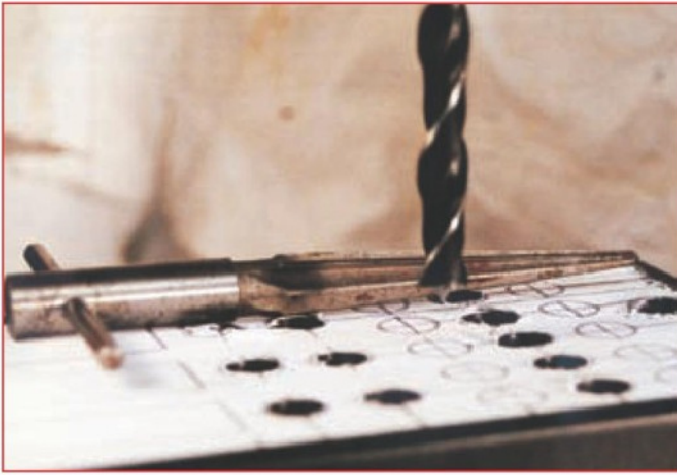
9. Drilling the case.
