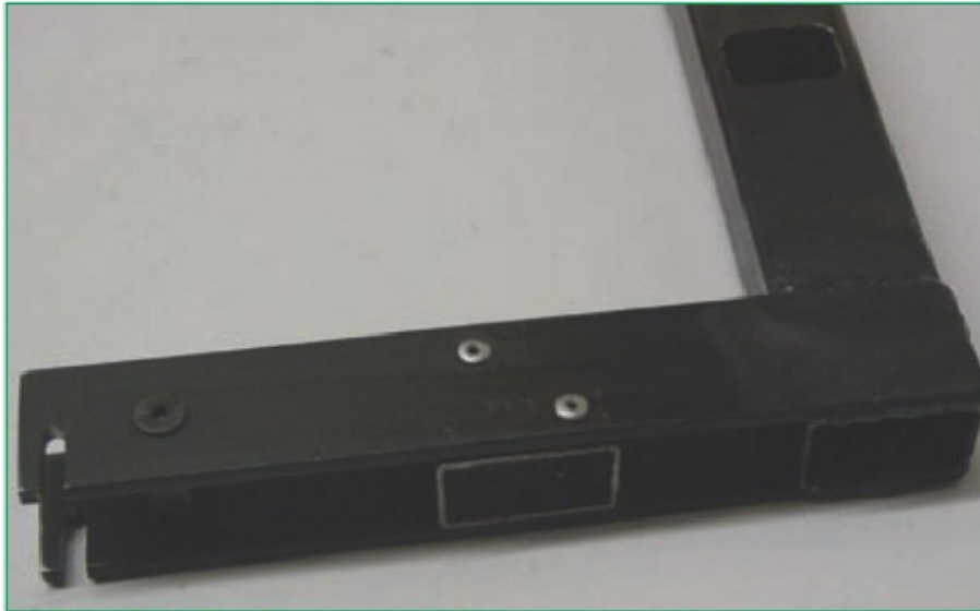
6. Guides are retained by pop rivets.
