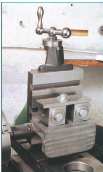
5. Machining the ends. Note the vertical slide has been set parallel to the lathe's axis. This set up is not unlike a mini horizontal mill. However, available traverse of the vertical slide is somewhat limited.
