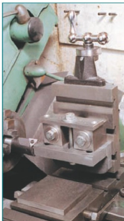
6. Machining the second end. Note the cover to prevent swarf entering saddle slideways.
