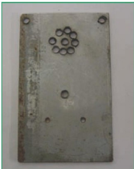
9. Motor mounting plate part drilled.
