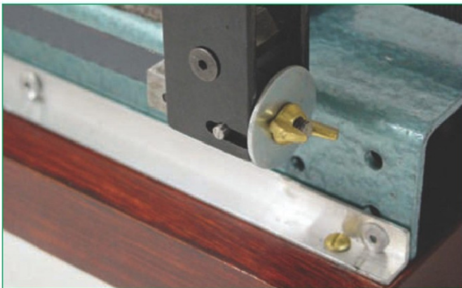
8. Blade mounting fitted to frame.
