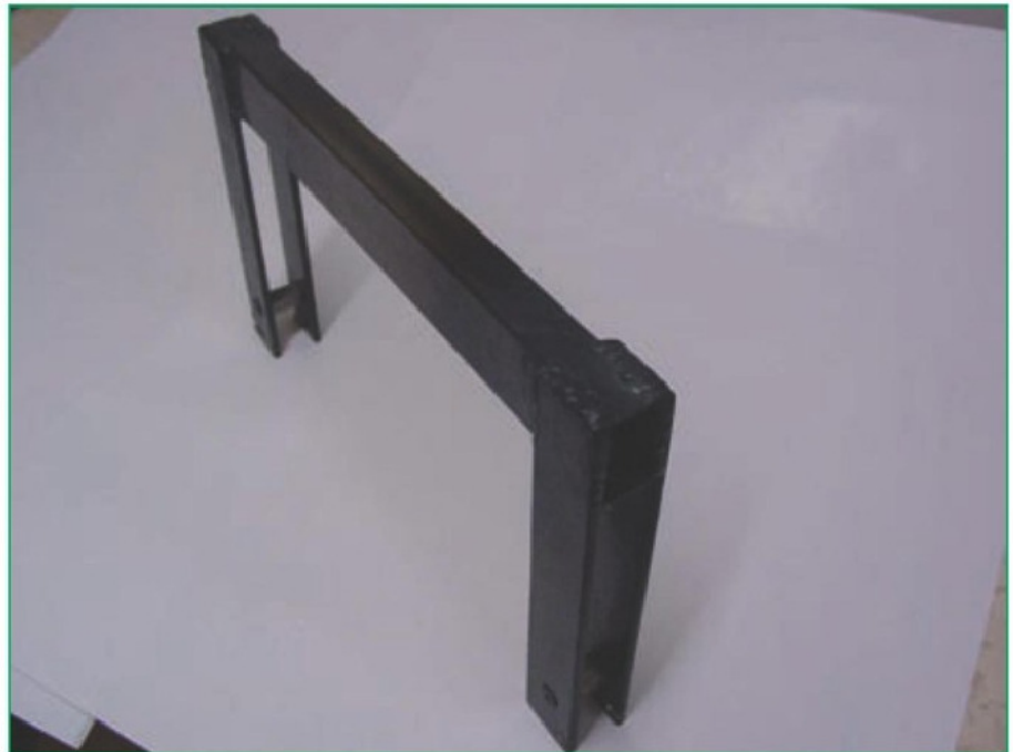
5. Frame welded, spacers in place.
