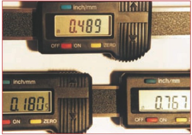
5. Yes two heads on one beam does work.
