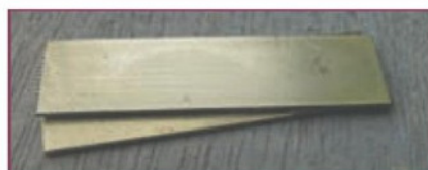
8. Soldered brass strips with only minor marking to the surface.
