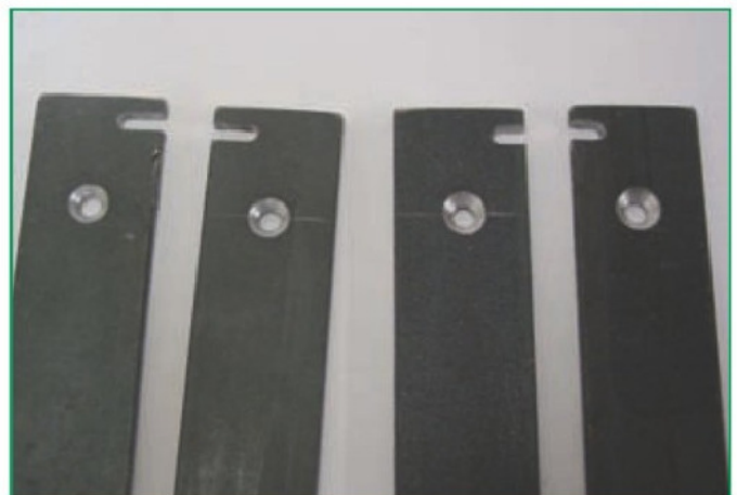
3. Parts of frame showing slots for blade holder.
