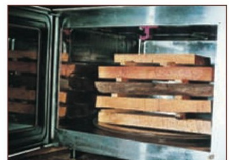
2. Wood stacked in microwave oven.
