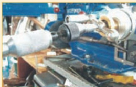
Flexible drive taken to cross slide.
