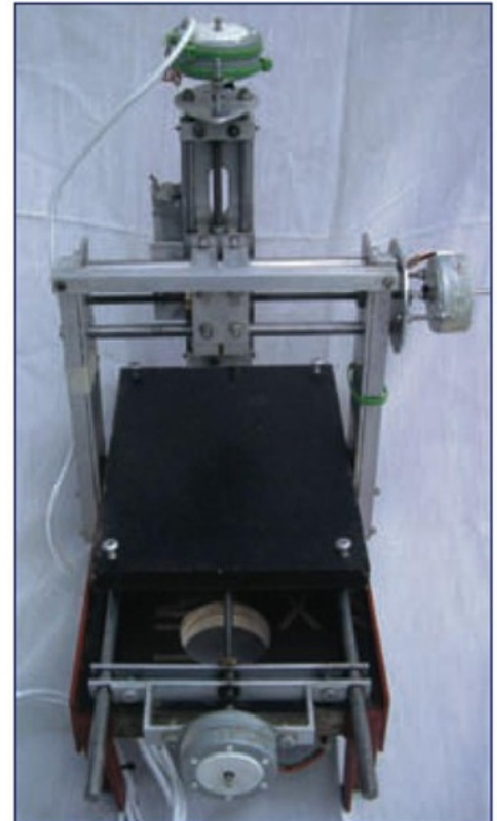
6. Front view of machine, clearly showing gantry arrangement.
