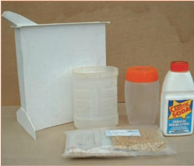
26. Tank made from 2mm polystyrene sheet shown with chemical packs.
