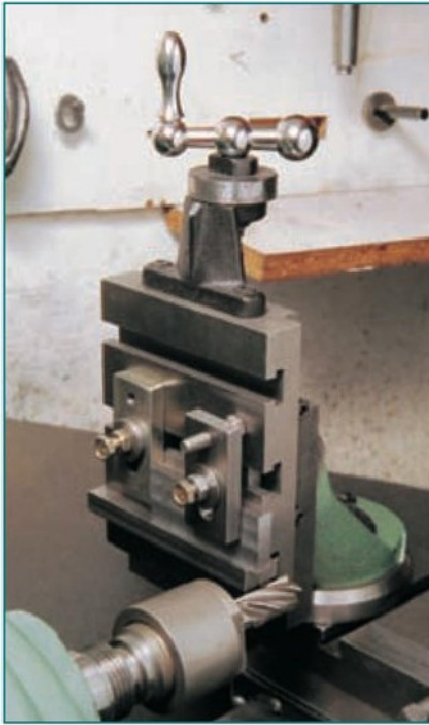
4. The method of finishing the ends of the various rectangular bars required.
