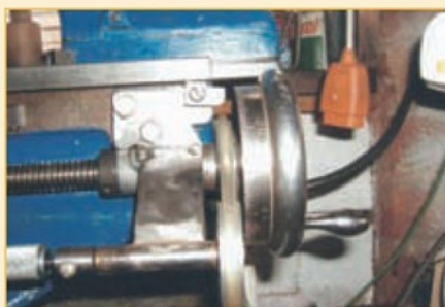
System driven from a pulley attached to the handwheel.
