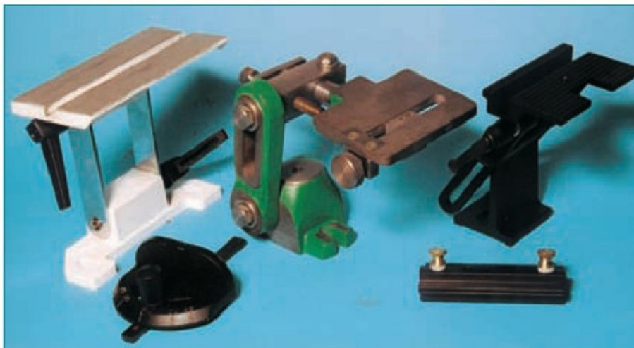
1. Three typical grinding rests, two commercial, one made in the workshop.
