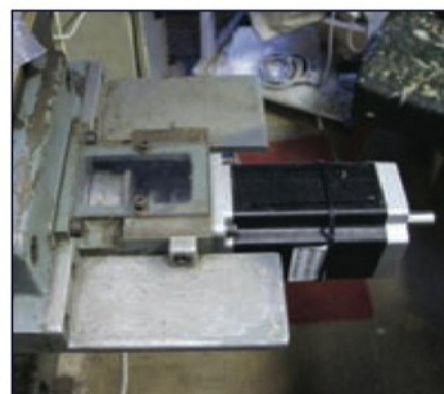
X axis directly driven by size 34 motor.
