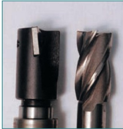
8. Helix angle of a tipped tool and conventional end mill compared.
