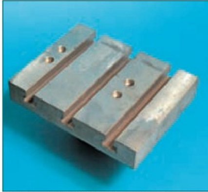
3. A tee slotted table for adding to a cross slide where tee slots are not provided.
