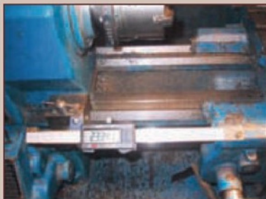
Cut down caliper used as saddle DRO.
