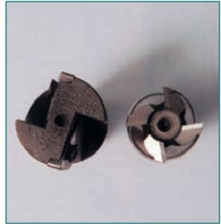
9. Rake of a tipped tool and conventional end mill compared.
