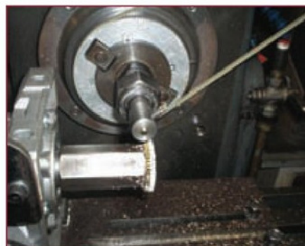
2. Hobbing a gear electronically, the encoder drive belt is visible.
