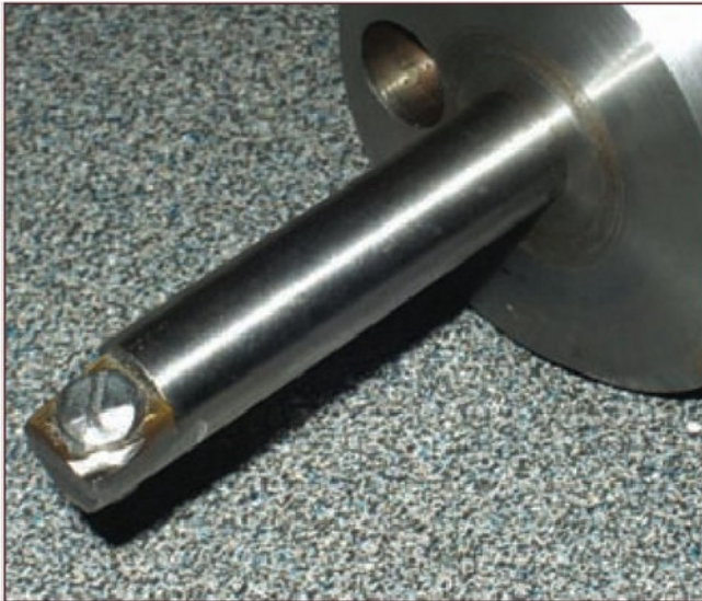
2. Home constructed bar using carbide tip.
