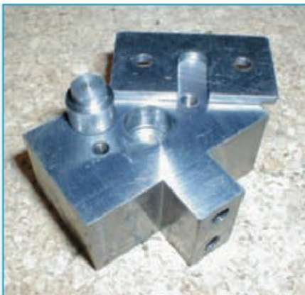
4. Screw retaining plate with moving jaw and shouldered plug.
