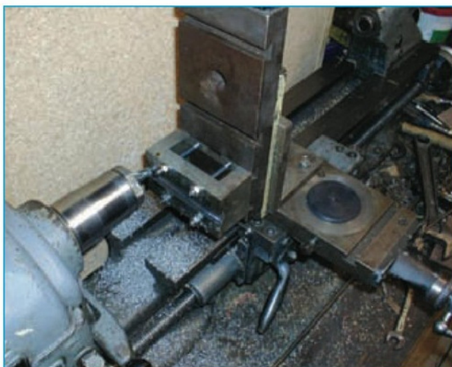
2. Machining the slot and tracks for the sliding jaw.
