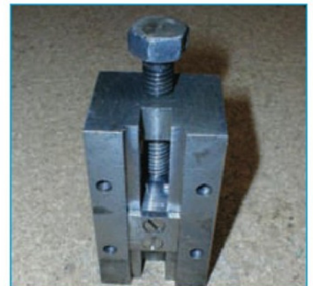
6. Underside view with jaw bottom plate clearly visible.
