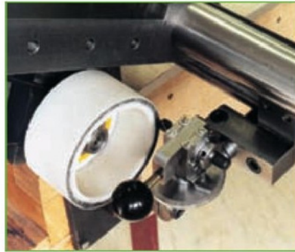
6a. Set up for sharpening an end mill.
