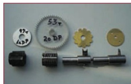
7. A selection of components and the cutters used to create them.
