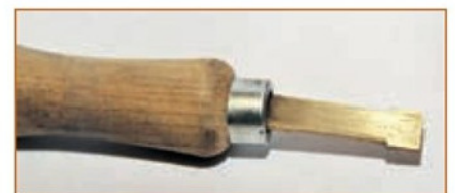
2. One of a set of 4 brass screwdrivers used for tightening and unscrewing blued screws. A steel screwdriver does tend to scratch the bluing.
