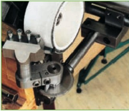
5. Set up for sharpening a lathe tool.
