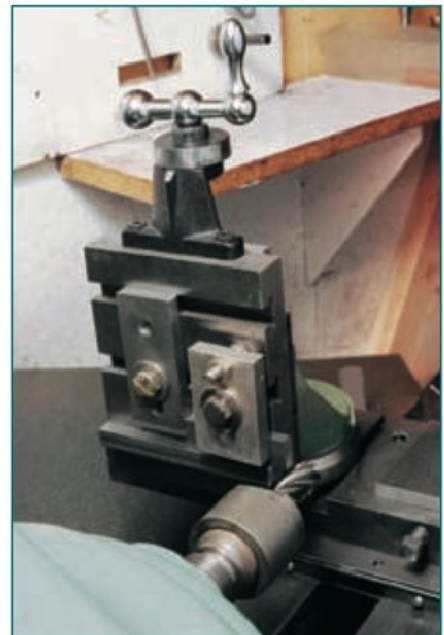
11. Similar to the set up in Photo 6 but the second support is mounted at the end of the workpiece for accurately machining a batch of parts to the same length.
