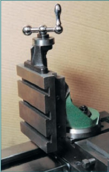
2. A vertical slide is essential for most milling on the lathe.
