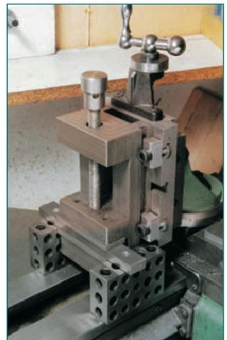
4. and 5. The method of clamping these two vices onto the slide allow their position on the slide to be easily adjusted.
