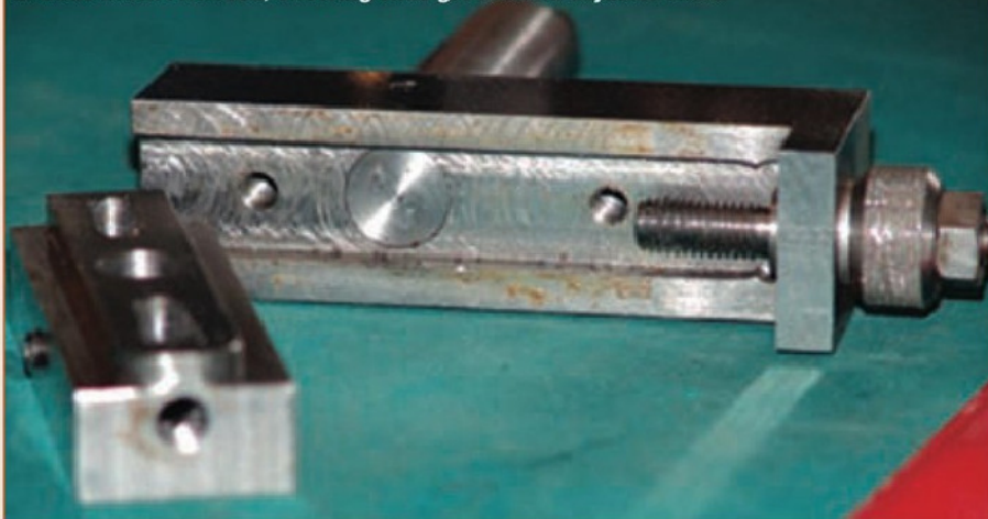
2. Slide block removed, showing slide groove and adjuster shaft.
