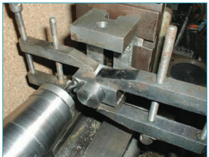
3. Milling the tenon on the moving jaw.
