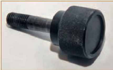
1. A free cutting mild steel thumb screw. This was oil blacked and has been in use on my door for about 10 years, the recess in the head is purely cosmetic; it makes the head look lighter, without actually reducing the strength of it.
