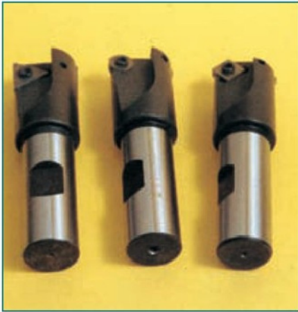
7. Three economy tipped tools that will be very useful for machining cast iron. However, the lack of a positive helix places more load on the lightweight cross slide/vertical slide set up. Rate of metal removal is therefore limited.
