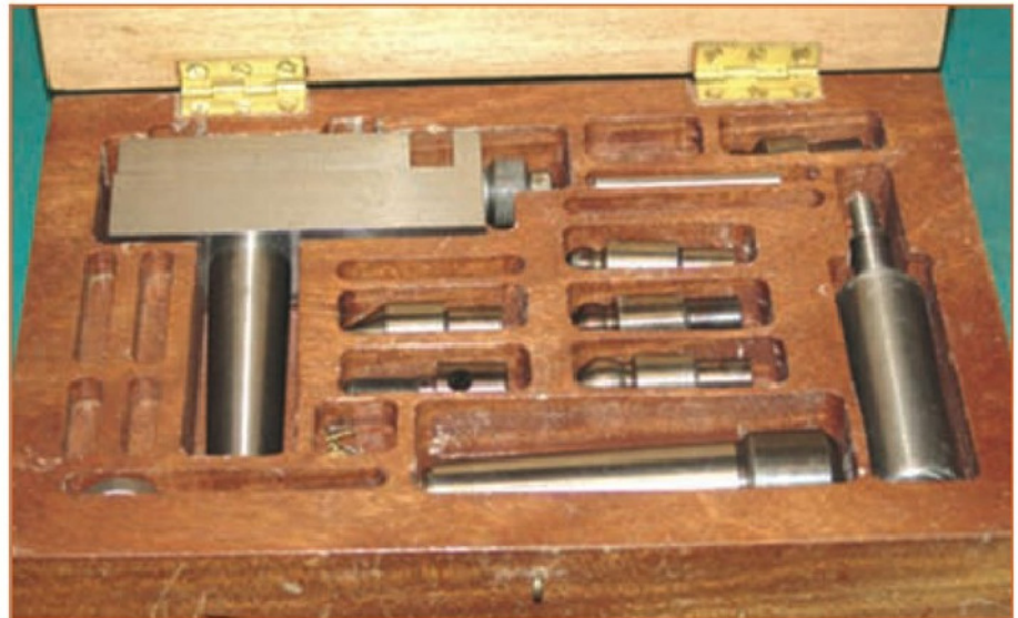
1. Completed off centre device with spherical centres and alternative arbors, in case.
