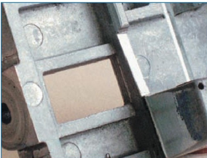
3. Material has been removed from the inner web of the saddle.
