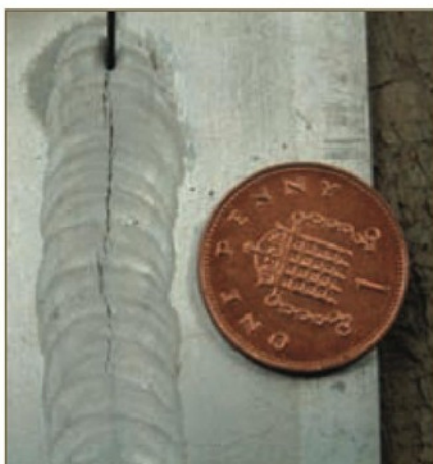
11. If you seek to weld aluminium alloys without adding filler, you will often get cracking like this. Silicon-rich filler alloys provide an almost total cure, but the associated need to "prep" the edges and feed the filler is tedious and unappealing.
