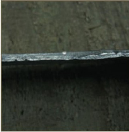
13. An autogenous (no filler) weld might look quite OK, but if you examine the reverse side you will often find that the penetration is poor or non-existent. Flexing in a manner to open the root gap will often cause the weldment to fail, allowing visual confirmation of how little penetration had been achieved.
