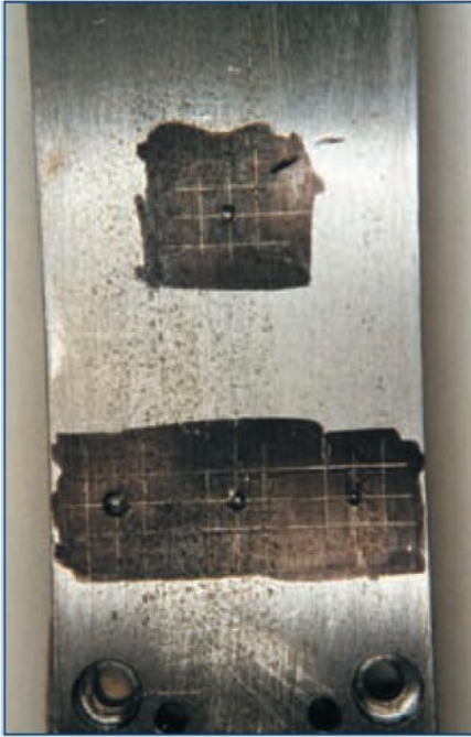
12. A component marked, boxed and centre punched ready for the drilling.
