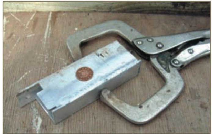
18. It is beneficial to use powerful clamps to facilitate assembly, but with those clamps being carefully adjusted so as to apply very little force. Then, the stiffness of the clamps prevents excessive creep during the period when the parent metals are at elevated temperatures, while at the same time the welds are not subject to the tensile forces which, if the clamp was absent, would cause cracking.
