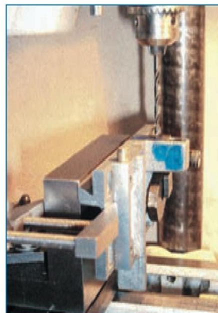
2. Using the drilling attachment.
