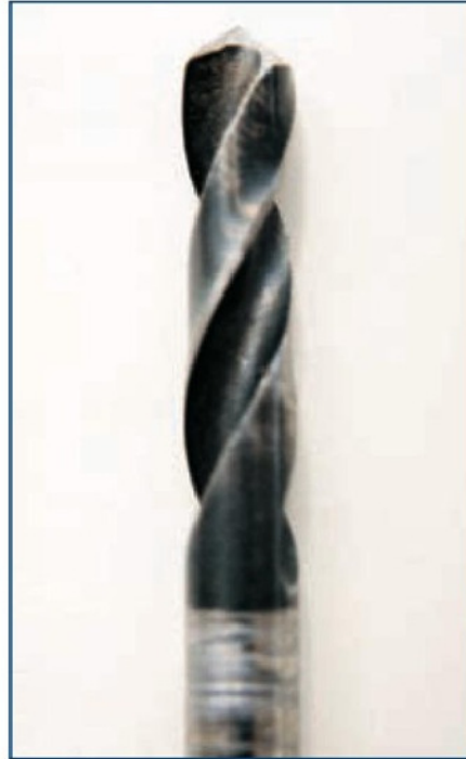
7. A short drill which has had the web thinned.
