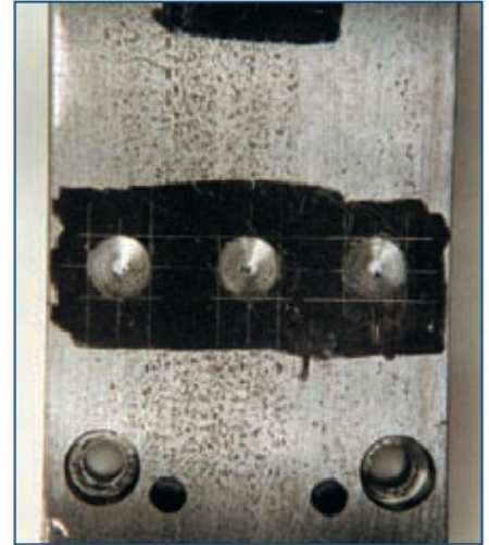
14. With the holes corrected, the drilling can be finished.
