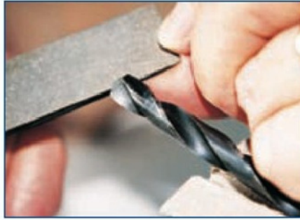
10. A smaller drill having its rake reduced. Photo-Pauline Loader.
