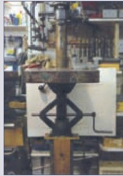
Use of a car scissor jack eases vertical movement of the drill table.
