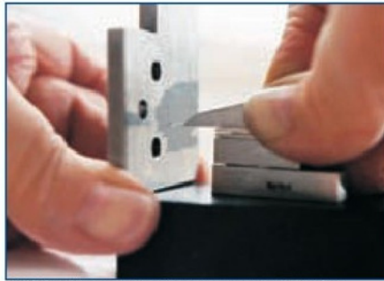
3. Marking out using accurate blocks. Photo by Pauline Loader.
