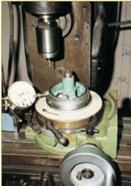
4. Clocking up the handwheel.
