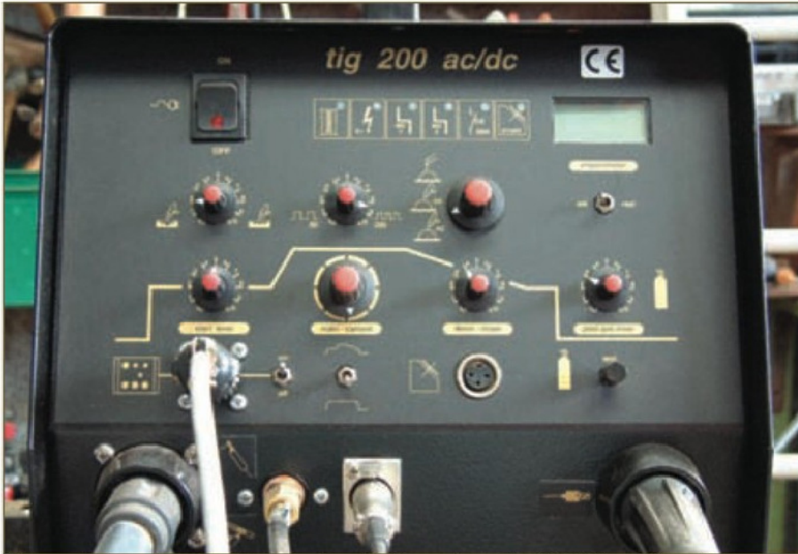
The controls and connections panel on the front of a typical AC/DC set. You will soon figure out what the glyphs mean, but figuring out the optimum settings for different procedures, different thickness of material and different weld types takes far longer.
