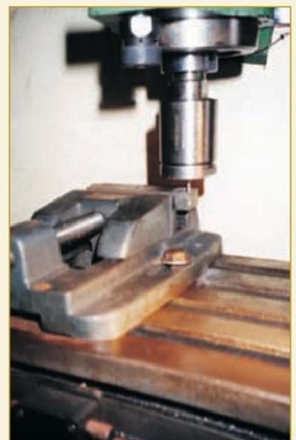
2. A trial run at groove milling.
