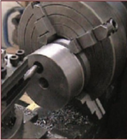
3. Boring location holes for bars
