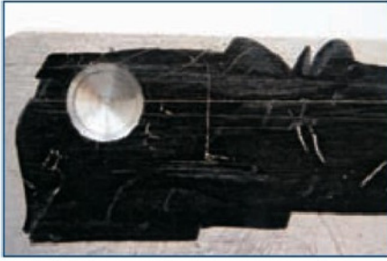
6. A drill just starting to cut, note the small shiny flat where the chisel edge does not cut.
