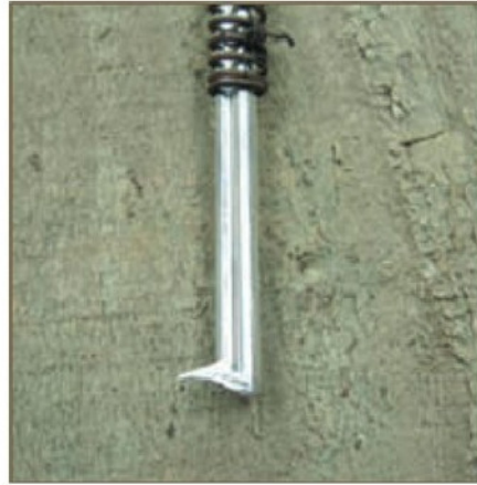
14. If you do not have the correct thickness of filler wire for the thicker jobs, your attempts to provide sufficient filler will be rather like trying to fill a bath with a teaspoon. Worse, you will experience problems with the thin filler rod getting too hot too quickly, making it difficult to add material to the weld pool. A partial remedy, useful only until you can get the proper filler rods, is to assemble three rods into a triangular cluster. You hold that cluster together at the far end with a bit of sticky tape, and hold it together elsewhere by a sliding spring, or whatever else is handy and suitable. You then get something like three times the filler feed rate and, more importantly, you can provide that filler into the weld pool.
