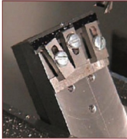
4. Milling the angle on the gib strip
