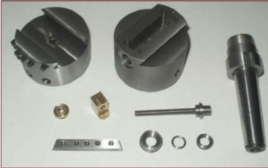
7. Key components of heavy duty head.
