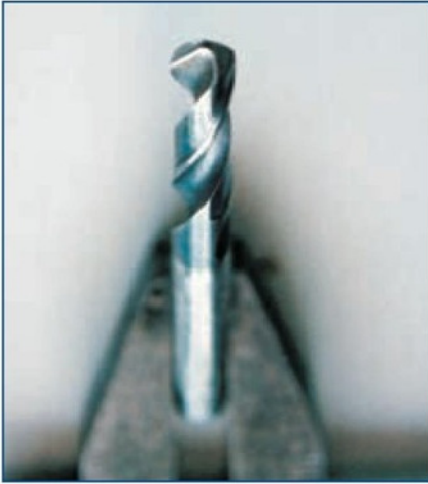
9. A drill which has had the rake backed off to stop it jumping.
