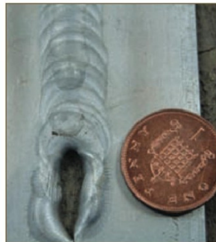
12. Here, surface tension has been coaxing the two pools to merge into one, but then disaster has struck, caused either by too wide a gap or by locally oxidised surfaces. From whatever cause, the surface tension causing the edges to pull apart has overcome the surface tension tending to cause one pool. Sometimes the situation is recoverable if in the early stages (when you first notice that the weld has stopped advancing) you provide a deft dab of filler. If it gets to this stage however, your best bet is to start again ... tomorrow!
