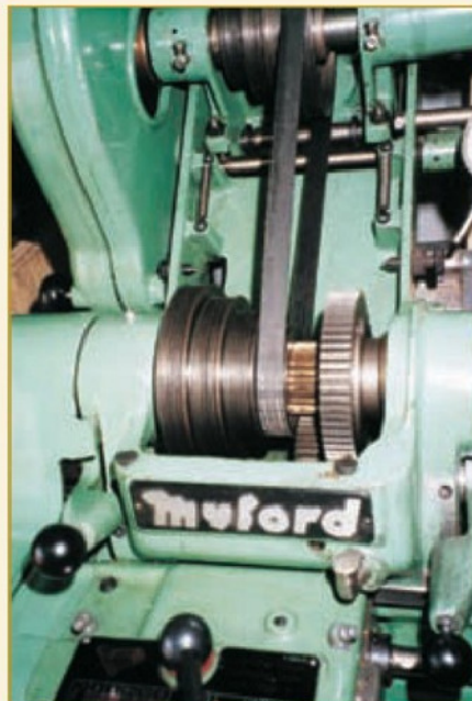
1. Home made poly vee pulley drive arrangement.
