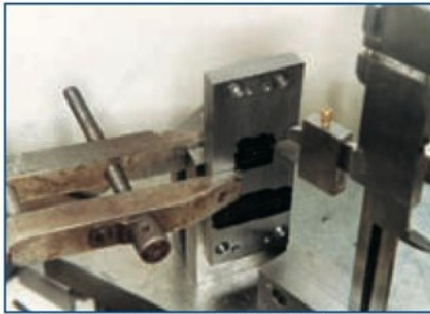
2. A component marked out using a marker pen.
