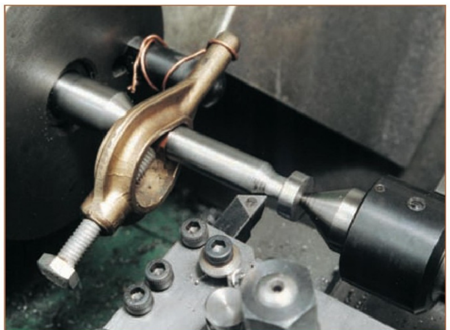
2. Turning the waist and head using left and right hand knife tools.
