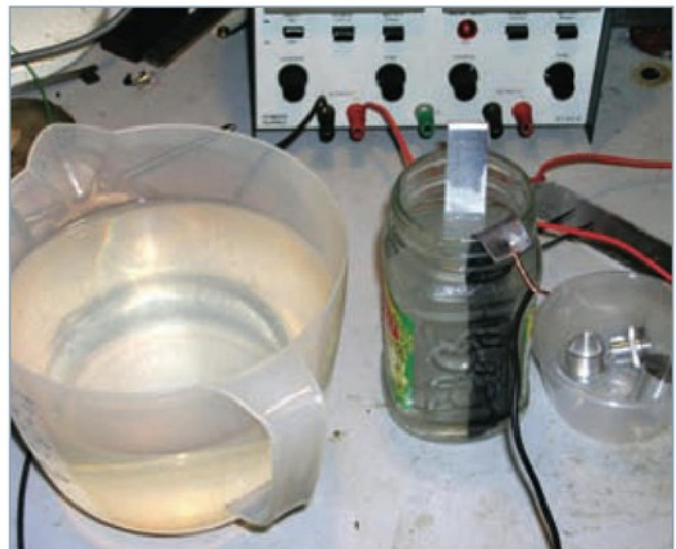
5. Arrangement for anodising.
