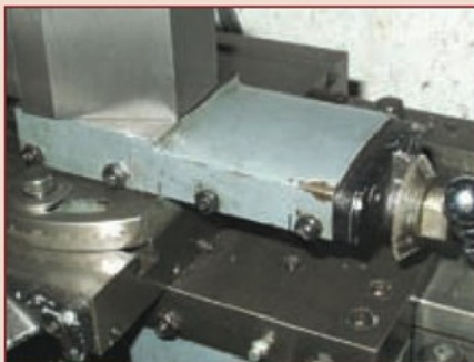
3. Reference marks used in measuring top slide angle.
