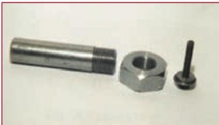
2. Lantern chuck with screw, disassembled.
