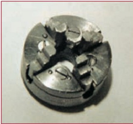
1. Model chuck on Stewart model lathe to show the screw heads in chuck body all lined up with the circumference of the chuck.
