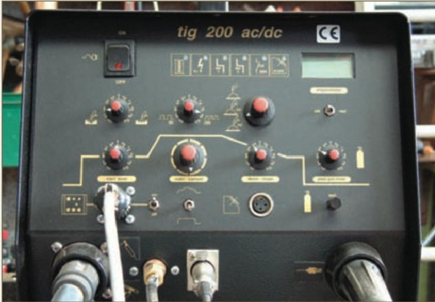
1. The controls and connections panel on the front of a typical AC/DC set. You will soon figure out what the glyphs mean, but figuring out the optimum settings for different procedures, different thickness of material and different weld types takes far longer.
