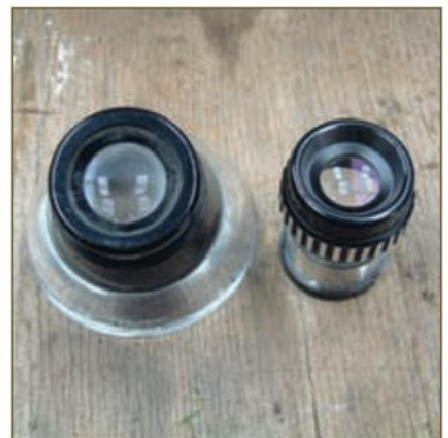
10. If you bother to investigate the extent of weakening of parent metals due to thermal cycles, you will need a way to measure the diameter of the indentations made by the ball bearing. Both of these magnifiers, having calibrated reticules, will serve that purpose.
