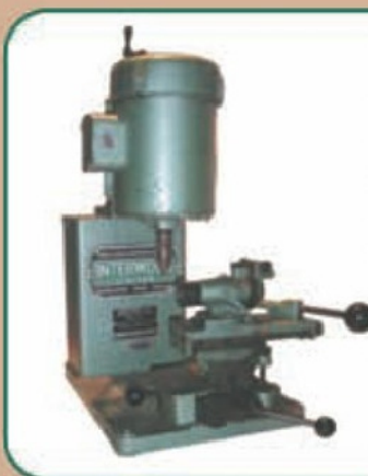
Cutter Grinder made by Interwood Essex. Originally for sharpening router cutters. Would easily adapt to tool and cutter grinder.
