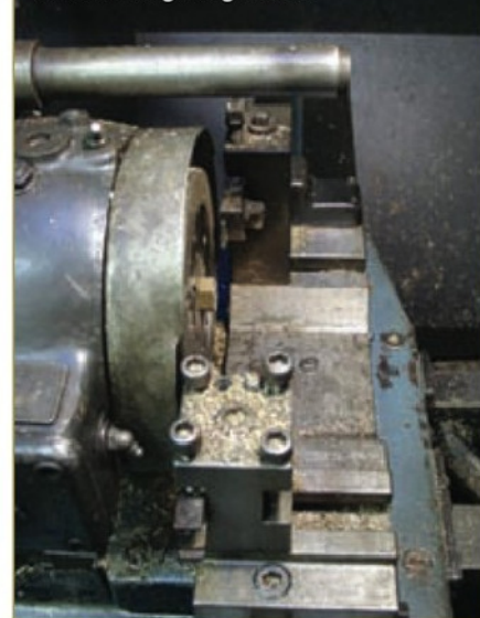
1. Tools on Herbert Capstan lathe in rough alignment
