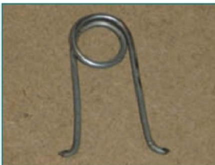
2. Simple mandrel thread cleaning tool made from old coat hanger.
