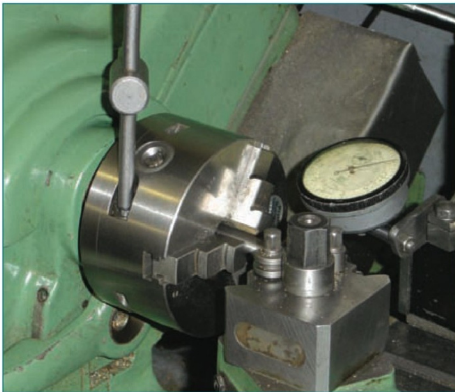
3. Alignment for concentricity: tightening the fine adjusting screw in the position shown throws the chuck body away from the dial gauge.
