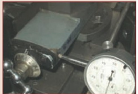
4. Using dial gauge for checking topslide angle. Note this topslide has machined sides.
