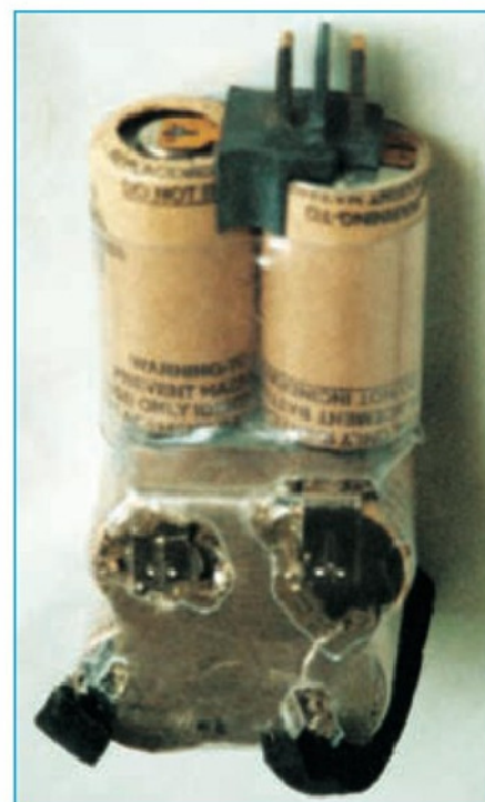
1. Battery pack opened up, revealing individual cells.
