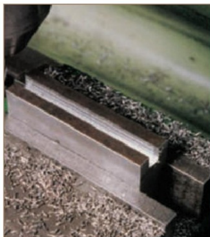
4. Milling the slot to take the head centre piece.
