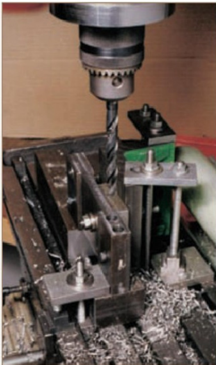
8. Drilling the two 10mm holes in the head assembly.
