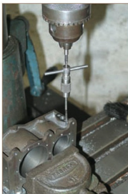
13. A tap wrench and tap have now been inserted to tap the hole.
