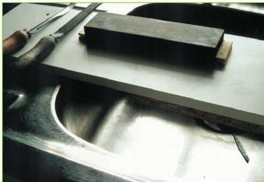
2. An oilstone fixed to the 'Bench' (photograph by Pauline Loader).
