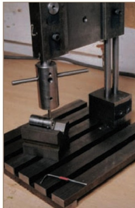
11. Putting the stand to the test before final completion by tapping the holes in the tap holders, again using only a plug tap.
