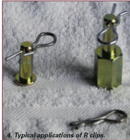
4. Typical applications of R clips.
