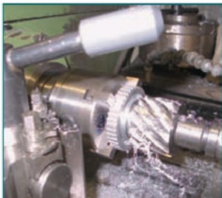
2. Boring the pulley using a Rotabroach.
