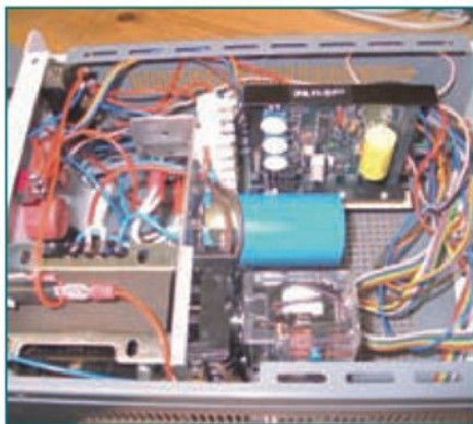
8. Power Supply and driver board.
