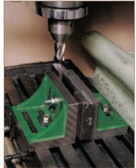
7. Levelling the bottom and top of the head assembly. See how two angle plates can in some cases be used in the absence of a large vice.
