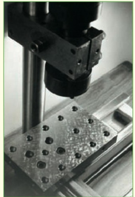
9. A nice finish for a milling/drilling table for a small lathe, the pattern is a result of random scraping in different directions.
