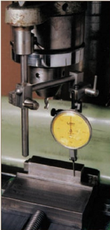
3. Setting the vice accurately in line with the axis of the table.
