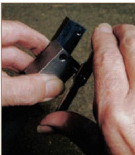
2. Hand tapping using a plug tap and a guide block.
