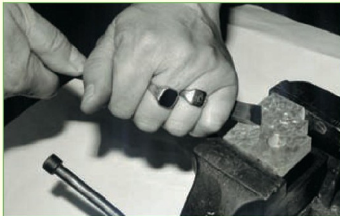
5. The small flat scraper being used.
