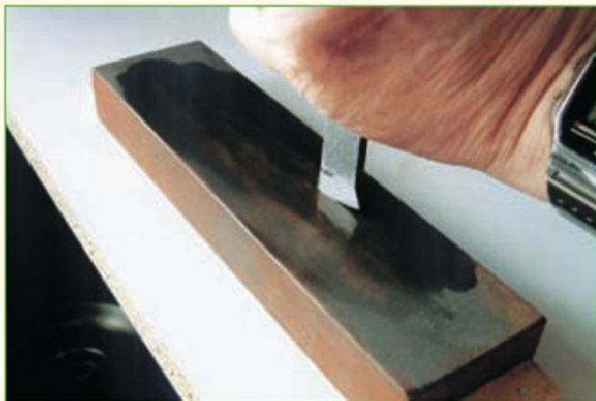
4. Stoning the scraper edge (photograph by Pauline Loader).
