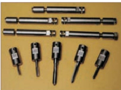
10. The spindle assembly parts for 5 sizes of threads.
