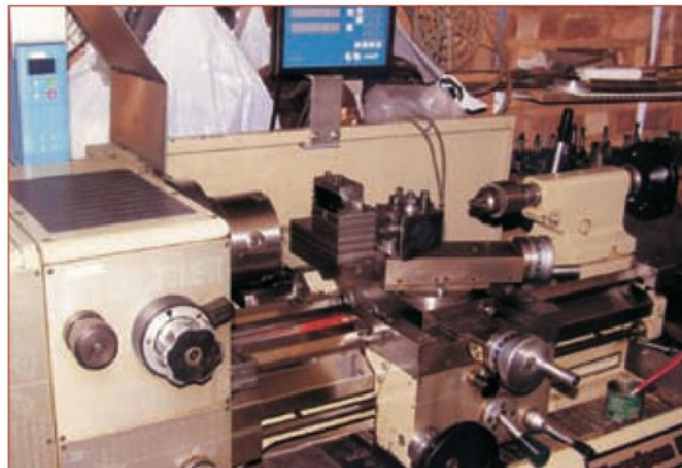
3 A general view of the front of the lathe also shows the Eurotherm inverter drive, and the Newall DRO system, definitely one of the better life enhancing benefits brought to us by modern technology.
