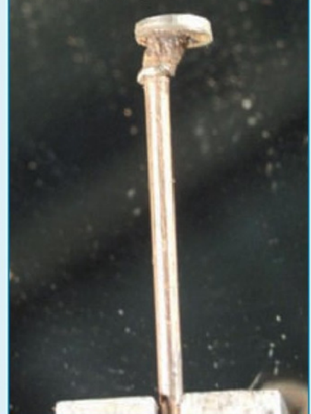
4. Spot welded assembly has deformed sideways.
