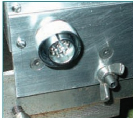
7. Detail of multi-way socket.
