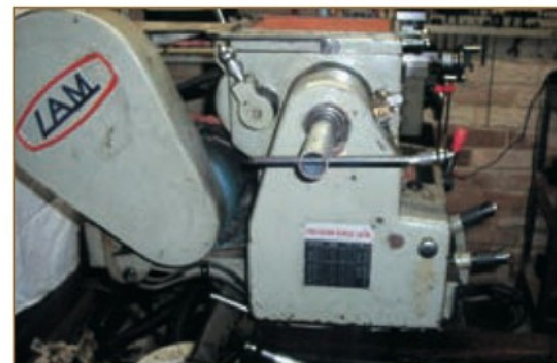
4. Tommy bar to apply locking torque.
