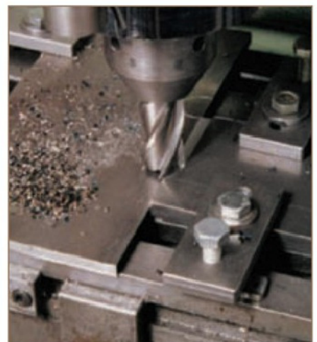
5. Commencing to machine the webs on the end of the centre piece.
