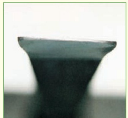
10. The cutting edge of the small scraper.
