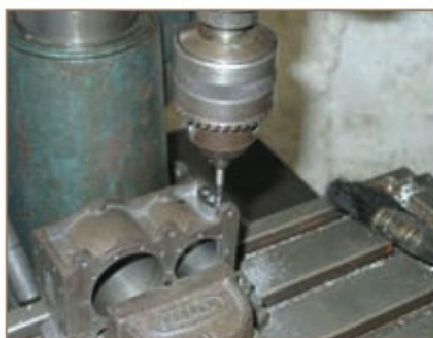
12. As an alternative to the tapping stand in this article a drilling machine can be used, in this photograph the hole and spindle are being aligned.
