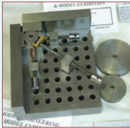
7. Also by P. Bowler, the design for this aid to jig boring was found in Guy Lautard's 'Bedside Reader'
