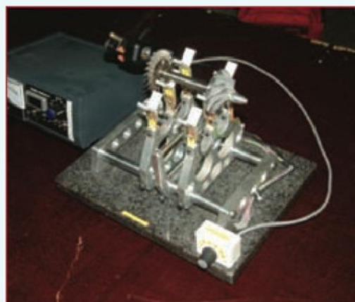
24. Used in the manufacture of miniature gas turbine engines, this dynamic balancing machine was to be seen on the Gas Turbine Builders' stand.
