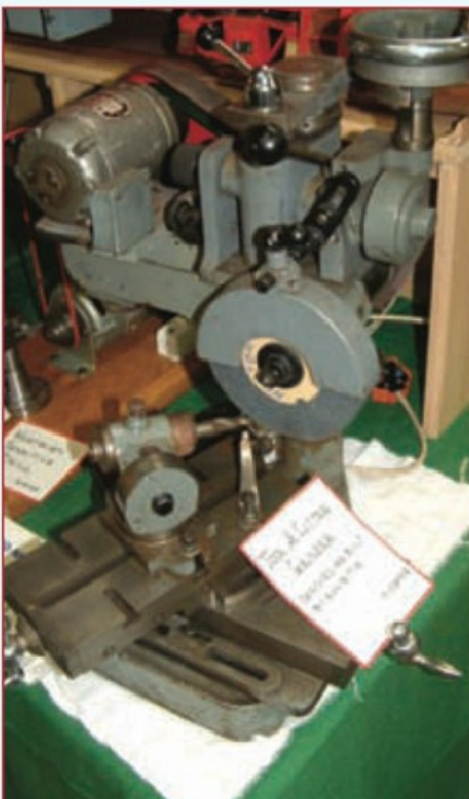
11. Mike O'Dwyer of the Keighley and District Society designed and built this tool grinder.
