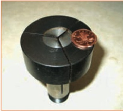
9. Large diameter "emergency" 5C.
