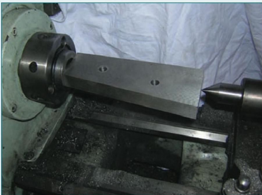
7. Using the taper gauge to set the topslide angle.
