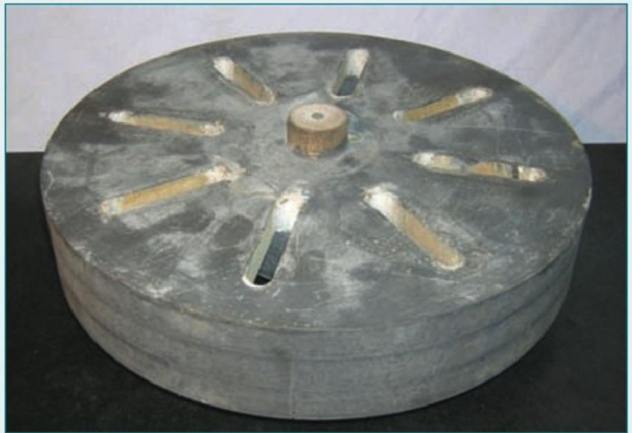
1. Pattern made from MDF used to cast backplate.
