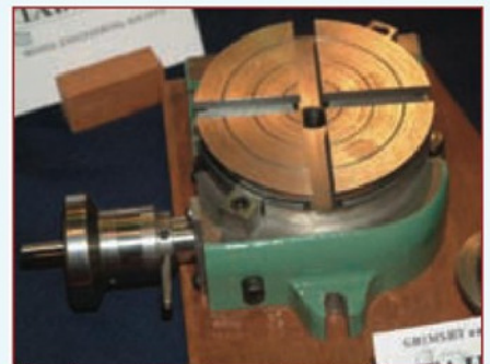
12. A neat 4in. rotary table by John Rhea of the Grimsby and Cleethorpes Society
