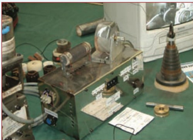
23. Mike Sayers of Pickering is building a 1/8th scale version of the engine of his 3 litre Bentley. This form relieving tool was used in the manufacture of cutters for the helical gears in the turret of the engine. The design is based on one published in Model Engineer in June 1949.
