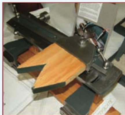
4. Also Highly Commended was Malcolm Leafe's taper turning attachment for a Smart & Brown lathe.
