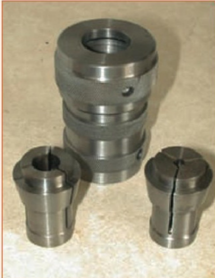
1. Home made collet chuck for Myford seven.
