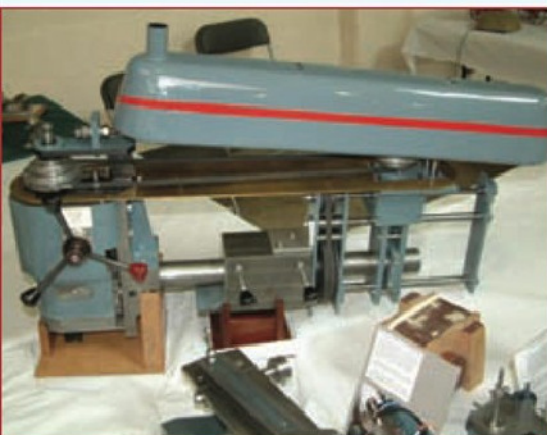
3. Designed to fit a Centec 2B milling machine, Gordon May's vertical head was awarded a Highly Commended certificate.
