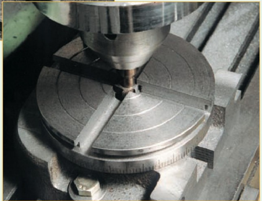
19. Milling the arms of the tee slot using a home made tee slot cutter.
