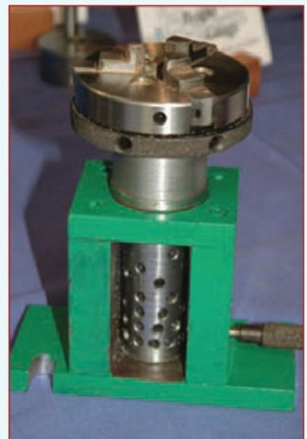
17. A neat direct dividing device by John Matthews of Grimsby and Cleethorpes.
