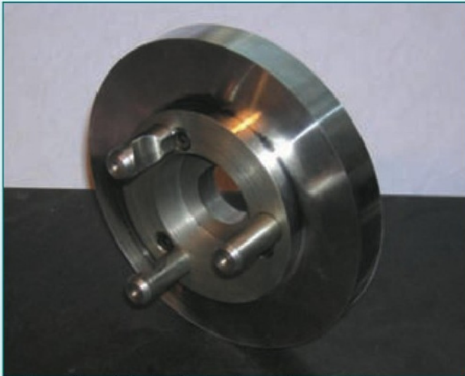
4. Rear of faceplate clearly showing studs and retaining capscrews.
