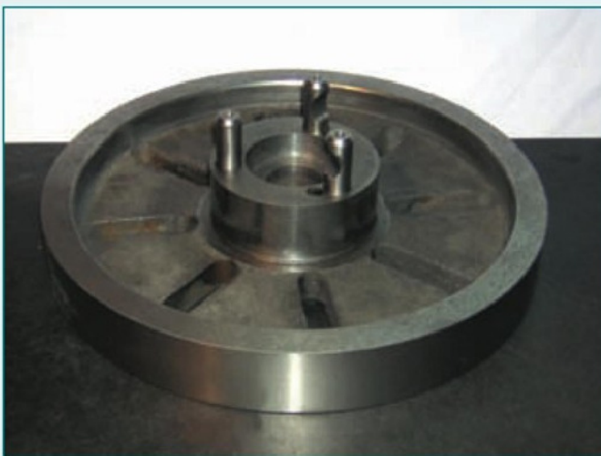
2. Completed backplate showing D1-3 studs.
