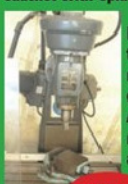
Myford Super 7B long Bed in almost immaculate condition with power cross feed, gearbox and hardened bedways on industrial cabinet with splash back
