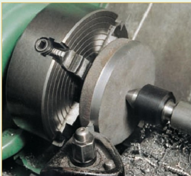
14. Rough machining the outer diameter of the table.
