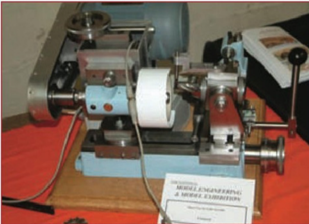
9. The Stent design is also popular, this version being by Peter Fedorof of the Tyneside Society.
