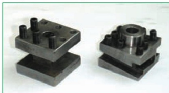
1. The two toolposts, angled slots (and milling error) visible on right.
