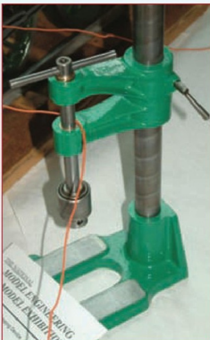
18. A simple tapping device by Edwin Hughes of Leeds
