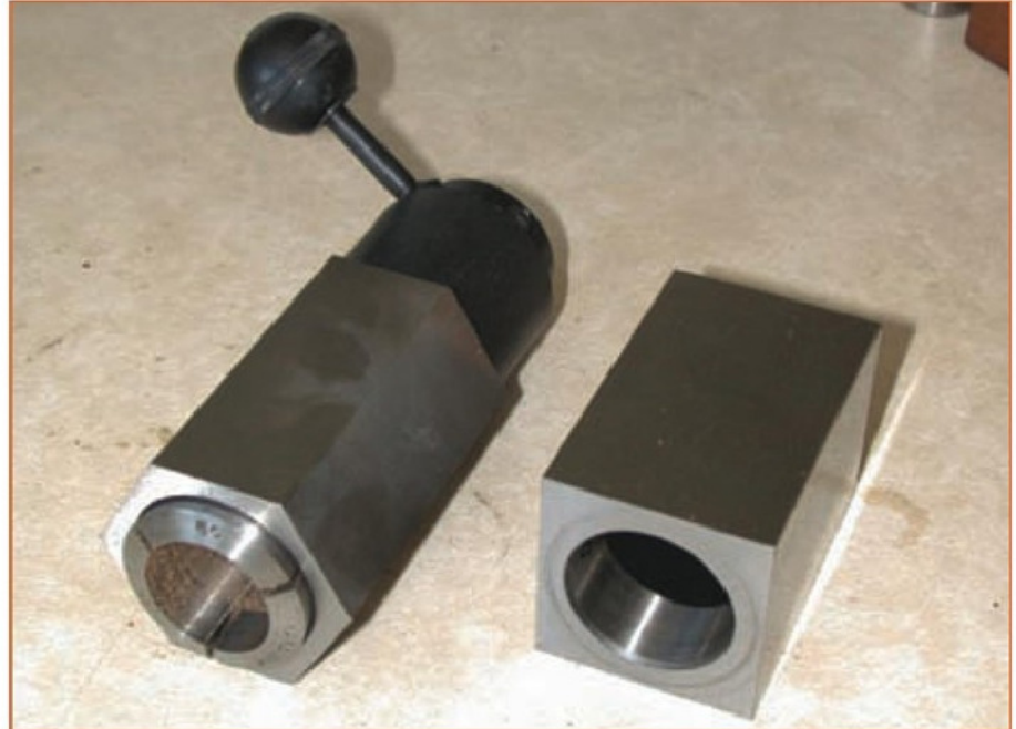
6. These collet holders aid machining squares and hexagons, are also a boon for cutter grinding.
