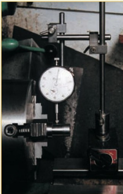
22. Using a dial indicator to set the eccentric spindle to give the required offset.
