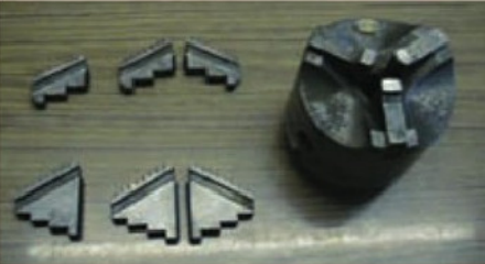
The component parts, note the angle of the thread on the jaws.
