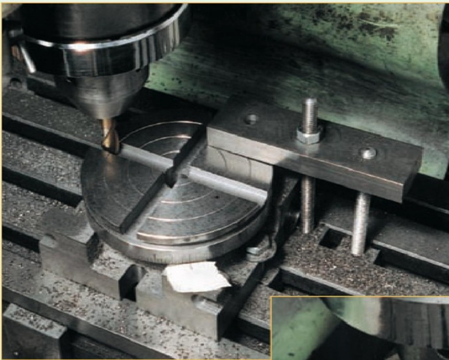
18. Milling the centre portion of the tee slot using a slot drill.
