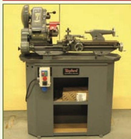
26. Back on its repainted cabinet stand, with new switchgear fitted, our reconditioned lathe awaits a new owner
