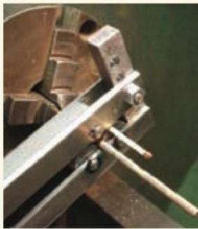
1. Knurling a slim component with the knurling pliers
