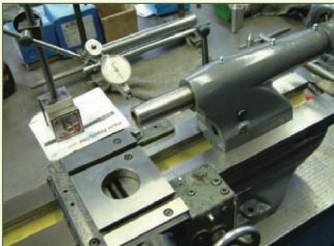
23. Operation of the tailstock barrel clamp must cause the barrel to lift no more than 0.001in. at a distance of 3in. from the body. Further checks are carried out with a test bar located in the Morse taper socket
