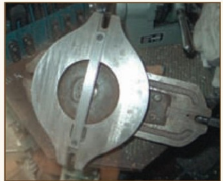
3. Underside of vice showing key
