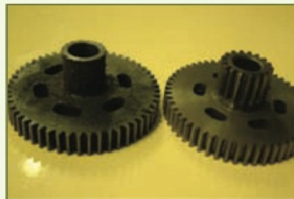
16. The old with the new. The back gear cluster had suffered badly, with no teeth left on the small pinion. The bull wheel was also short of its full complement, as can be seen in Photo. 2
