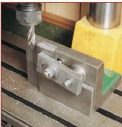
2. With the down feed set and fixed, the parallel will ensure that all parts are the same length
