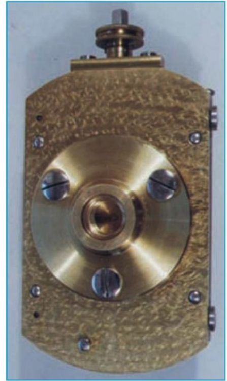
11. Holtzapffel chuck features detachable backplate.
