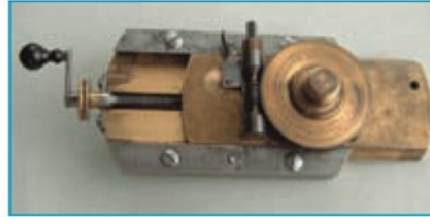
7. Eccentric chuck – with slide extended.
