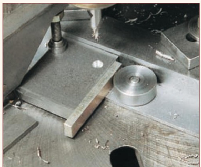
6. Drilling the first hole in one of the side plates, the disc plus 5mm packing achieves the 7.5mm dimension.
