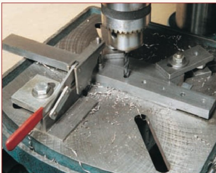
5. Using the pin to locate the bar, holes can be drilled at the required 20mm centres.
