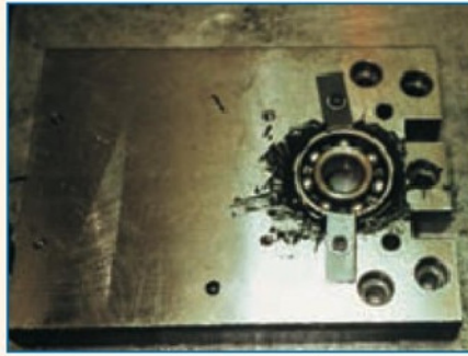
11. Gap around ball race filled with locating resin.
