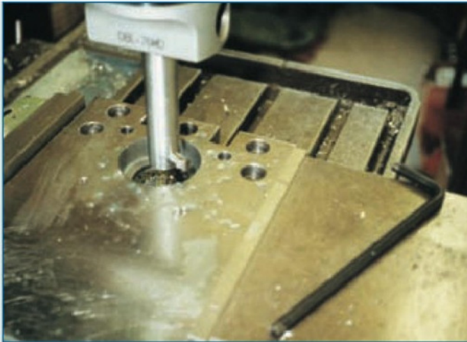
8. Boring the end bearing brackets for feedscrew bearings on CNC milling machine table.
