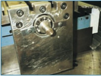
10. Ball race "centralised" by the feedscrew, then clamped.
