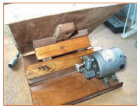
4. Mechanism for "Rocking table"
