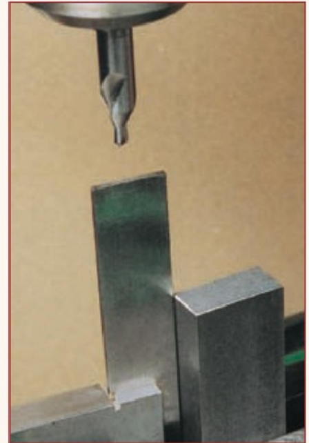
11. Removal of the 18mm packing enables the second hole to be positioned easily. The vice is of course clamped to the machine table.
