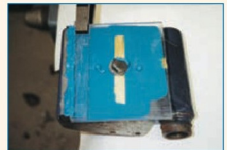
4. As photo 3 with low friction resin injected. Note two "blobs" of resin showing position of holes used to inject the resin.
