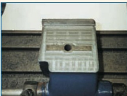
2. Finished machined tailstock.
