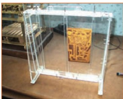
5. Purpose built etch tank – later version with PCB.
