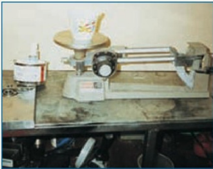
5. Balance for weighing out small quantities of resin and hardener.
