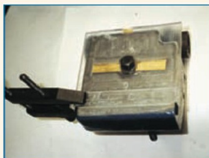
3. Tailstock with Perspex cover plate.
