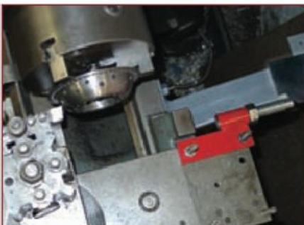
2a. Posed photo of workpiece and device from above fitted to lathe.
