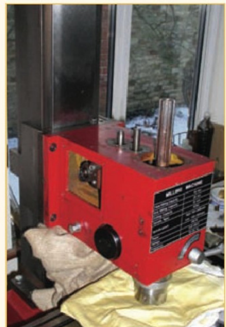
4. The weight of the head casting augers well for the general rigidity of the machine.
