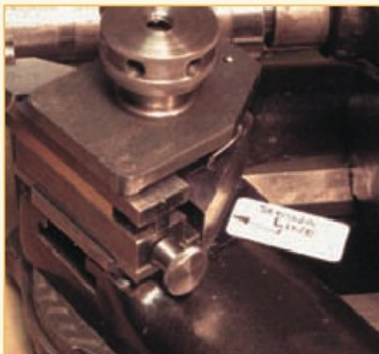
17. Setup for marking datum lines on compound slide.
