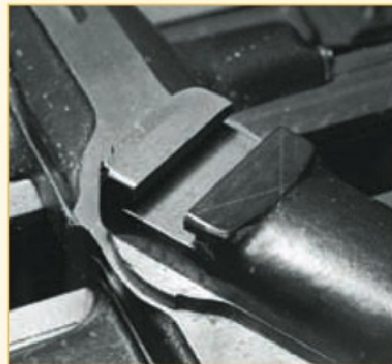
16. Screwcutting datum lines on compound slide face.
