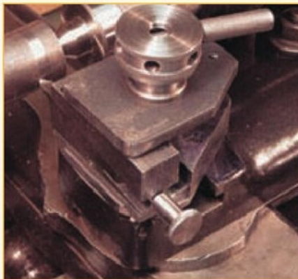
15. Setup for cylindrical turning.
