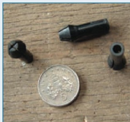
4. Three of the four standard collets. Made in a waxy black plastic, the range allows holding drill bits from the smallest (0.3 mm?) up to about 3.3mm.
