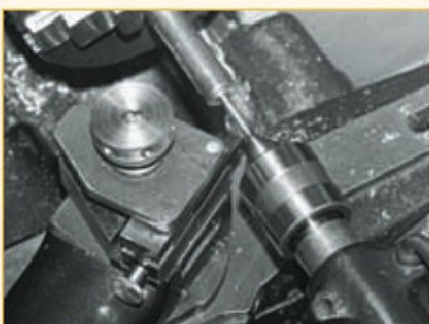
2. Cutting screw thread of elevating screw
