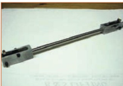
9. Limit switch bar complete.
