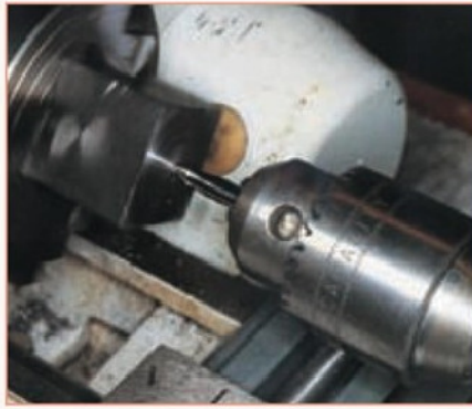
4. Centre drilling a block.
