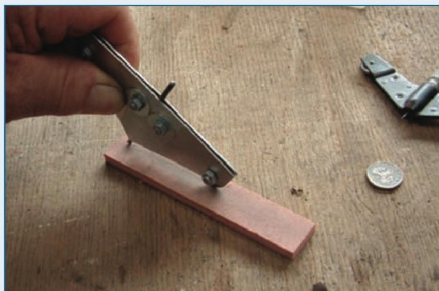
10. The "Son of Wishbone" in use, at the start of a sharpening stroke. The degree of tilt (to the left) is progressively increased during the stroke.
