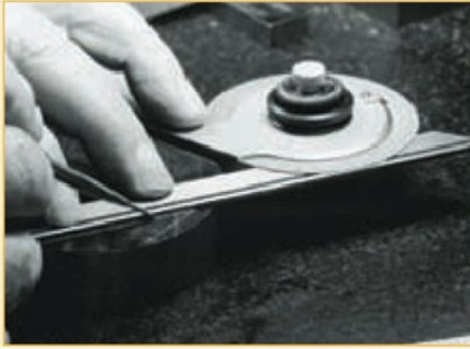
5. Marking out 60 degree datum faces.
