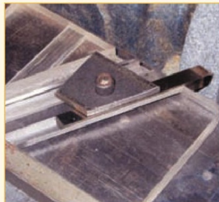
18. Jig used to generate 60 degree toolpoint on screwcutting toolbit.
