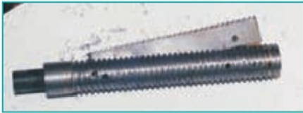
2. Making a broach by screwcutting. The blade is shown partially inserted in the machining arbor.
