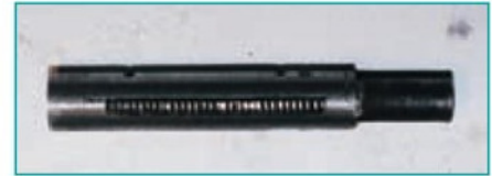
4. Although the incremental cut per tooth is only 0.05mm, it may be seen that some gullets are blinded by swarf.
