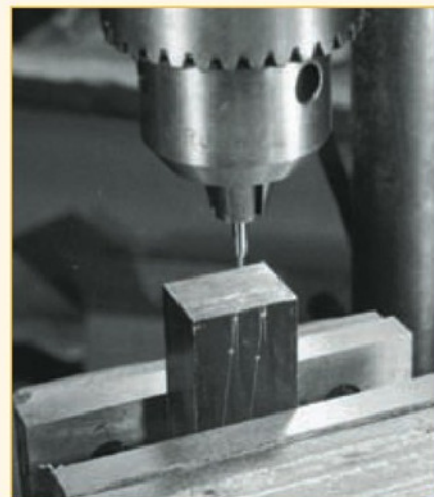
8. Centre drilling in preparation for through drilling of tool slot.
