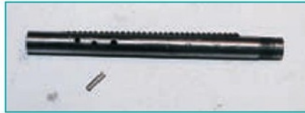
3. The broach blade located in the operating arbor. The depth of cut can be seen increasing from left to right, and the inclination is maintained by the dowels.
