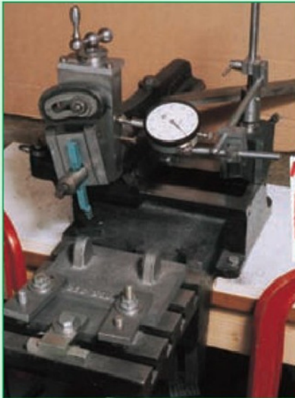
8. In the absence of a calibrated cross feed the dial indicator enables precise adjustments to be made.
