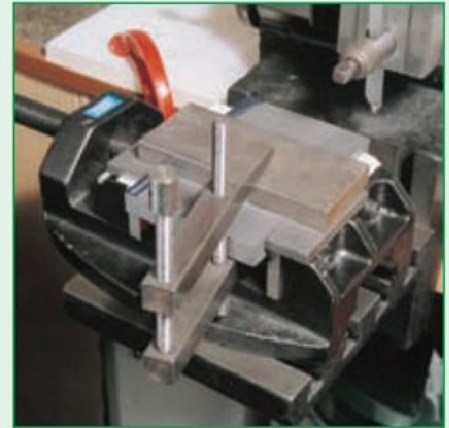
9. A plate clamped to the rough machined plate, together with spacers between it and the vice jaws enables the part to be accurately set up for taking a shallow cut for final finishing.
