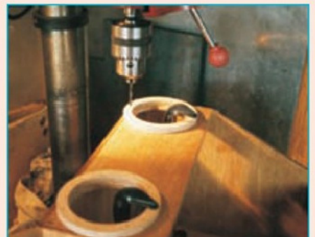
3. Drilling four holes through each ring
