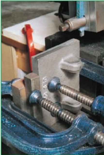
5. An extra support has been added to give added security to the mounting for machining the short edge.
