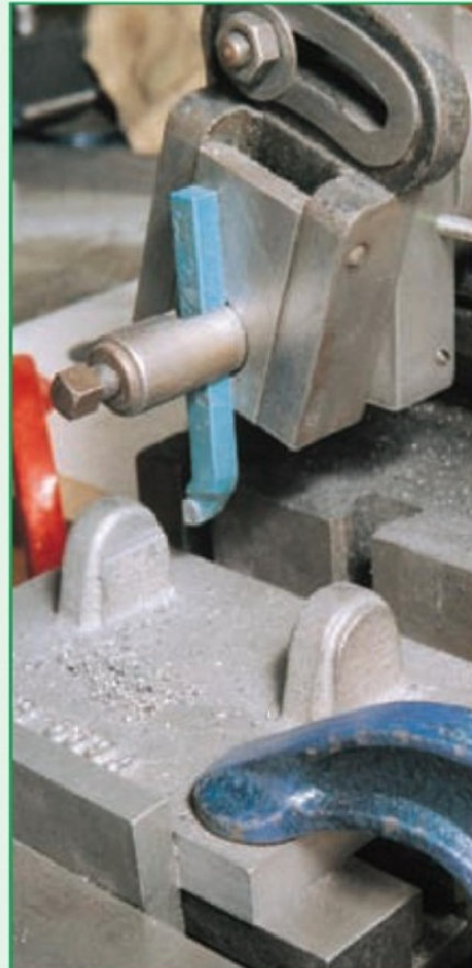
6. Rough machining one of the boss faces. Note the setting of the clapper box.
