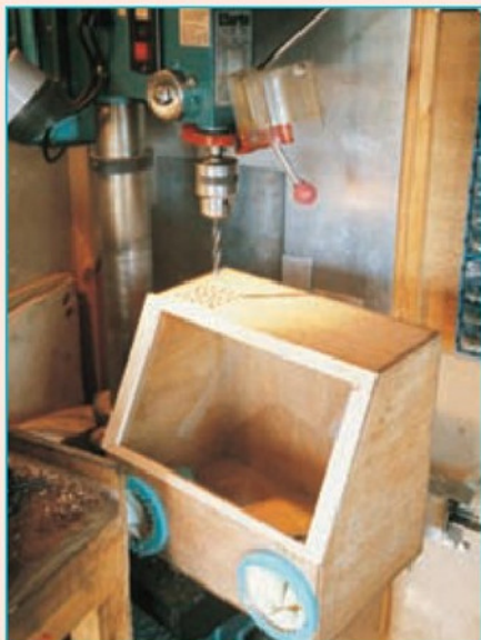
7. Matching holes are drilled in the cabinet
