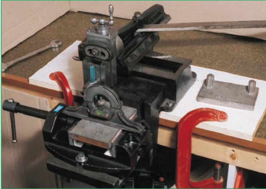
1. Setting up the first casting for rough machining its main face.
