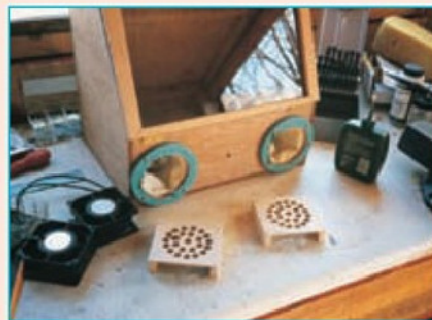
6. Air filter holders showing vent holes
