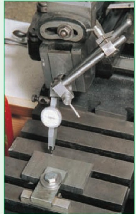
7. Positioning a fence for accurately locating each part for final finishing of the boss faces.
