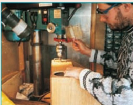
1. Trepanning the hand access holes
