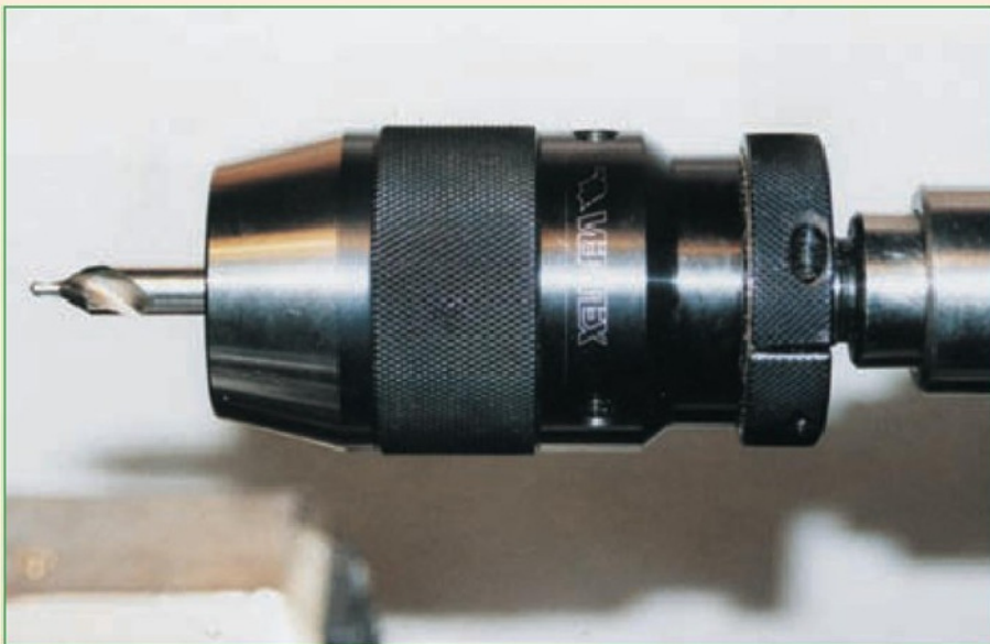
12. The keyless chuck is a great timesaver, but not so good for tapping.
