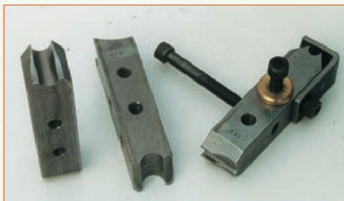
8. Three large support pads, one fitted with the protection angle piece.
