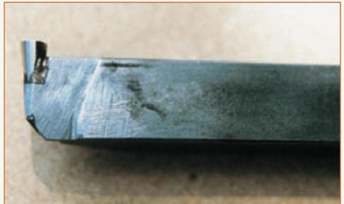
12. A form tool made by silver soldering a silver steel tip to a MS shank.
