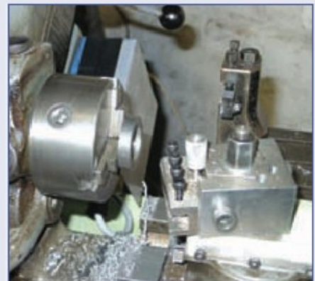
3. Preparing to take a 0.180in. cut. The new motor can just be seen (blue) together with the makeshift swarf guard.
