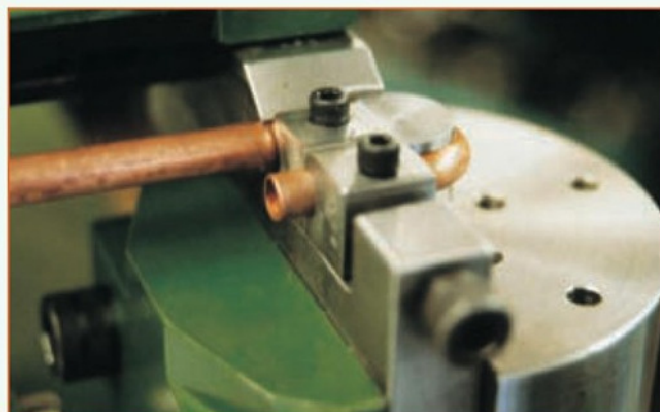
9. The fixed jaw has been cut away to clear the pipe on a 180deg bend.
