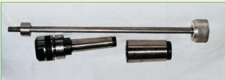
13. The 3MT milling chuck, with 5MT/3MT reducer, and draw bar.
