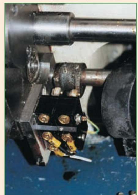
6. Motor control microswitches with as cast cams and plastic roller followers.
