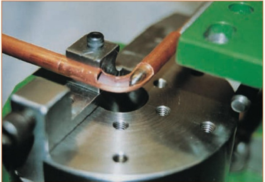
10. Sectioned pipe reassembled with bullet head to show positioning.
