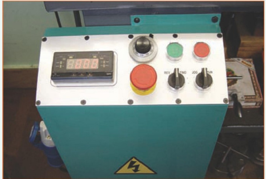
6. Control panel, note E-stop and tachometer.
