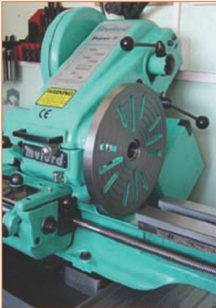
2. Chuckguard removed and large face plate fitted.
