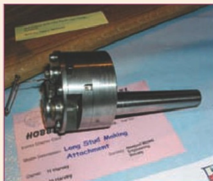
2. Howard Harvey's stud making attachment for 6 to 10 BA.
