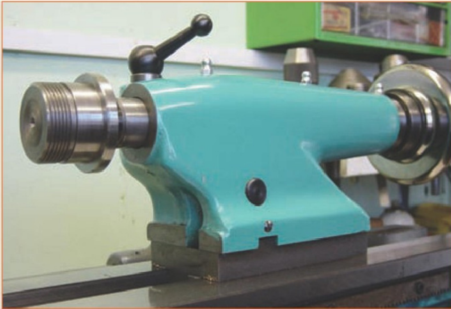
13. Tailstock attachment to accept older style chucks etc.
