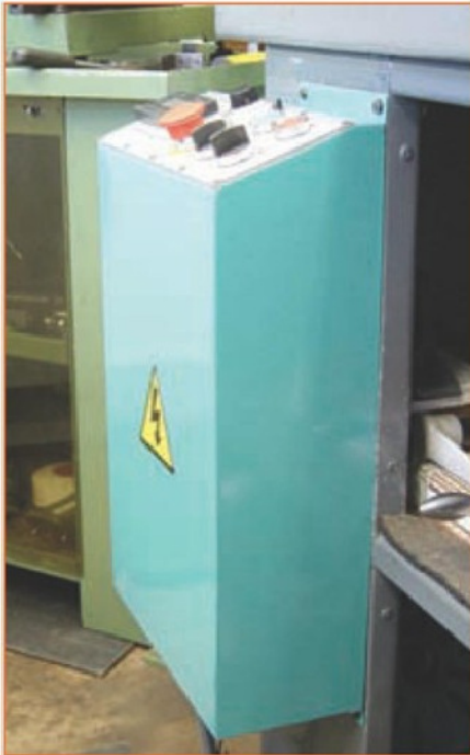
5. Inverter housing mounted at front of lathe.
