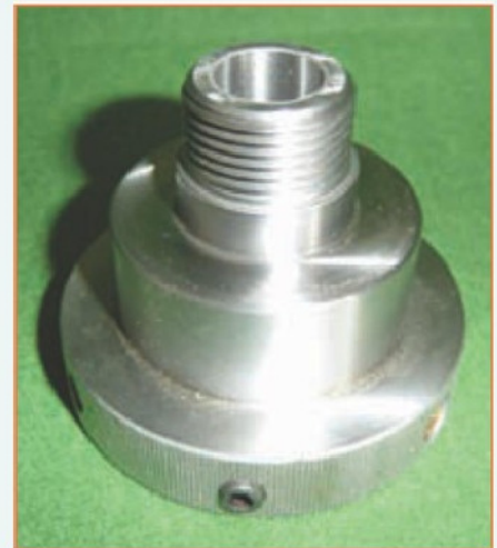
3. Spindle nose adapter enables use of older pattern chucks etc.
