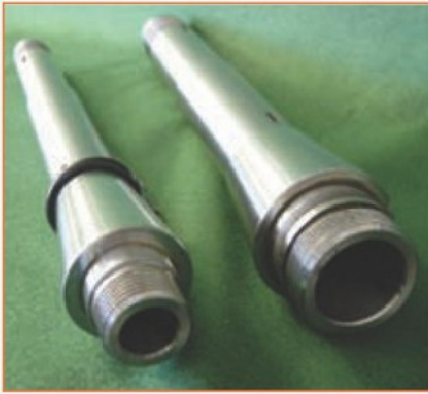
8. Showing the size difference between the old (left), and new (right) headstock spindles.
