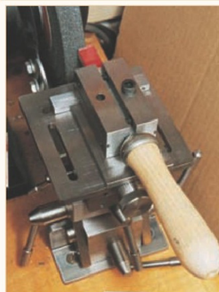
6. The same accessory used for the screw driver is also used to hold the wheel dresser.
