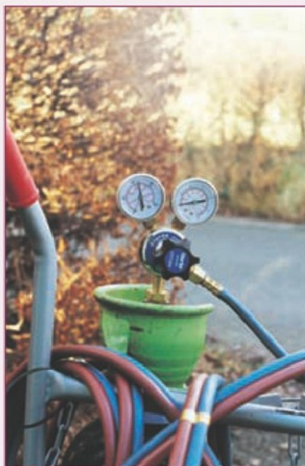
2. The ability to know feedline pressure, and to be able to accurately adjust the value, is critical to successful gas welding.
