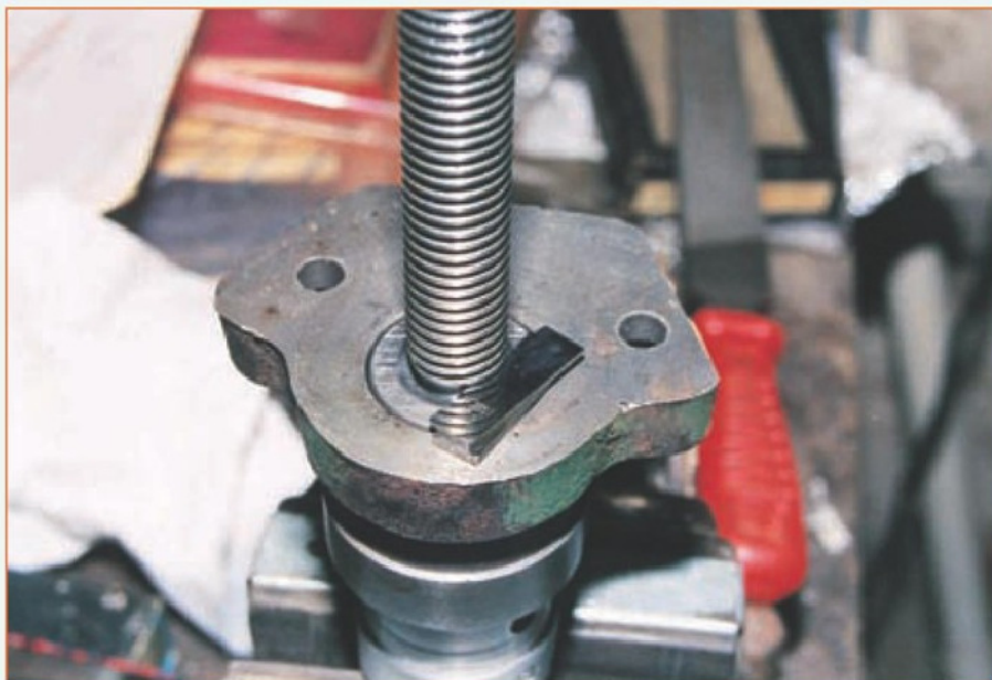
4. Measuring axial gap for stop collar.
