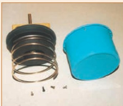
2. Top removed showing plunger / magnet assemble resting on spring.
