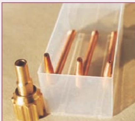
6. One welding tip screws in to replace another.
