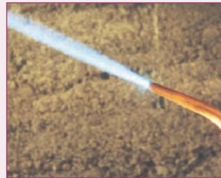
15. Early stage of moving from neutral to oxidising conditions. The intense white cone is hard-edged.
