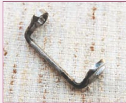
12. Tools can be modified in a trice to reach into those near-impossible locations. (This one was for the nuts joining the carb to the manifold on a 2CV!).
