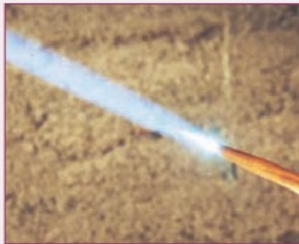
14. The transition between carburising and neutral conditions. An occasional and transient hint of excess acetylene seen beyond the intense white cone.
