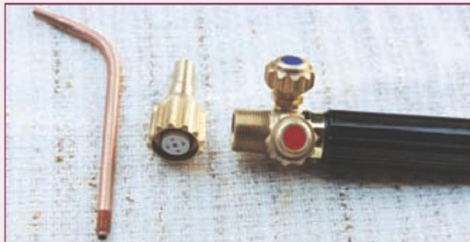
5. The torch is made up of valves, mixer unit, and tip.
