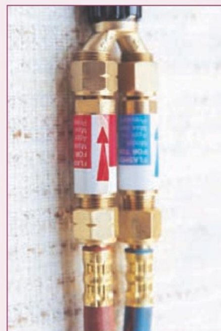
3. Absolutely, totally necessary. Flashback arrestors in each supply line.
