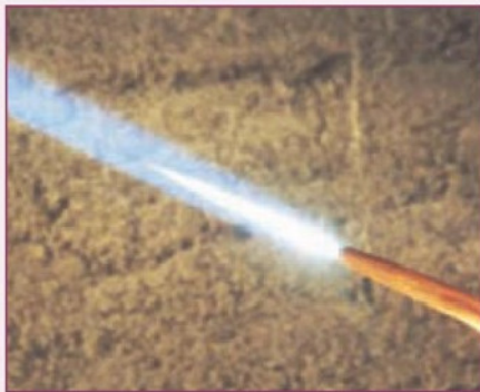
13. The starting point for fine adjustments to the flame. A long white cone of excess acetylene.
