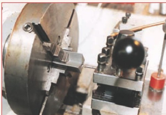
15. Re-boring plugged hole
