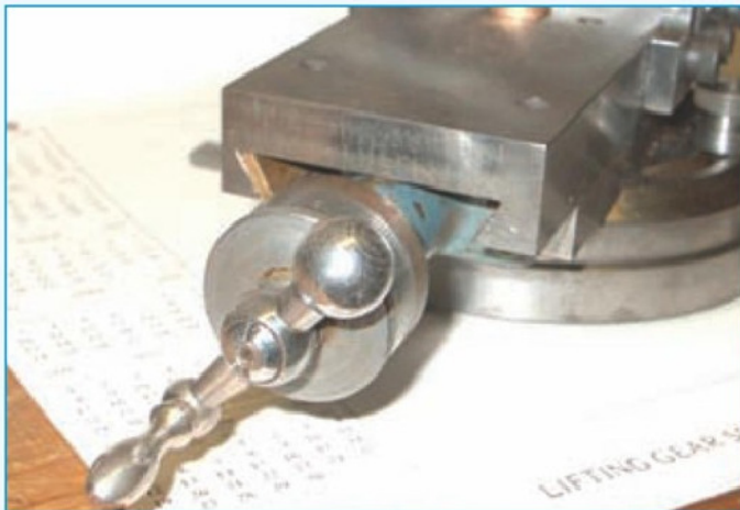
14. The slide adjustment handle was salvaged from a Boxford lathe.
