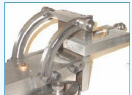
13. Tenon guide showing angular adjustment features.
