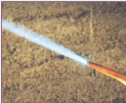
16. Distinctly oxidising. The intense white cone is now very small and the secondary blue flame has shortened to about two-thirds of its previous length. A far noisier flame than previously.
