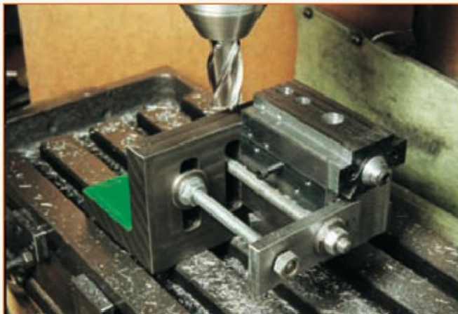
13. Machining the cutter carrier for weight reduction and better visibility when in use.
