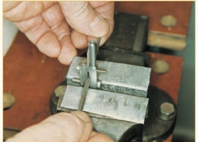
40. A square Swiss file used to finish the square in a small tap wrench. (Photo by Pauline Loader)
