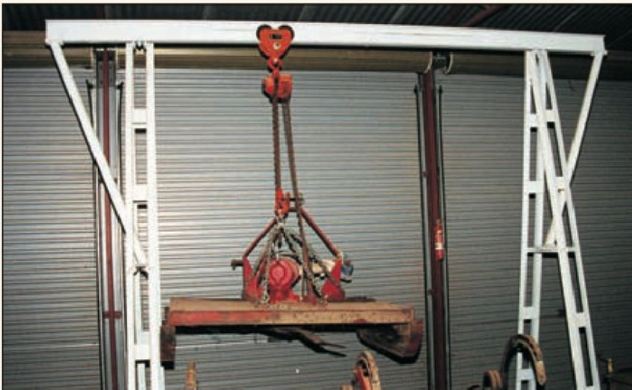
2. Crane lifting slasher implement.
