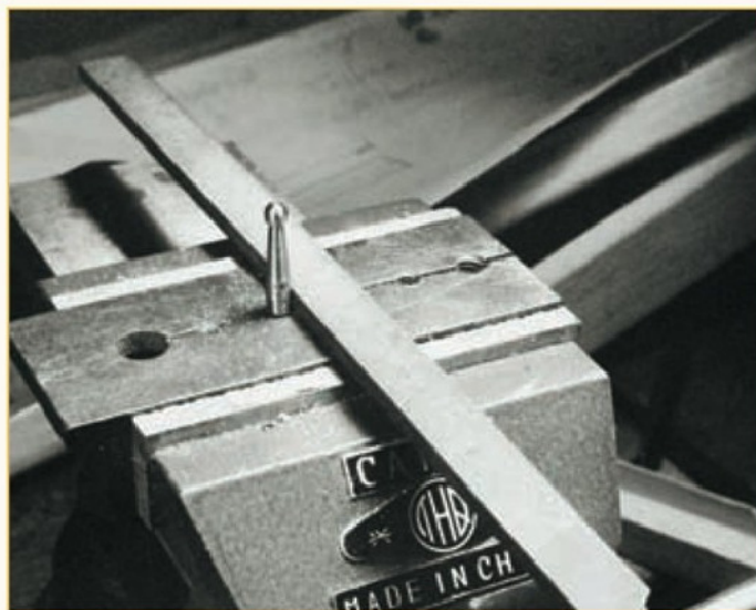
22. The pillar file used edge-on to file a small flat.
