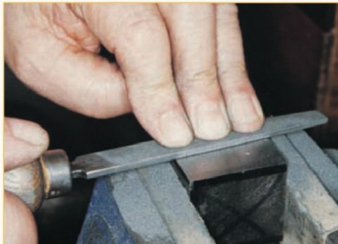
30. Precision filing to remove irregularities.
