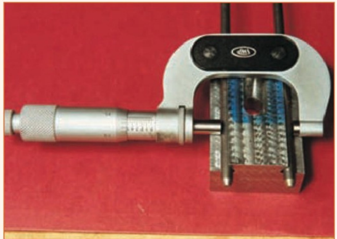
11. Using a micrometer and two rods to check if the dovetail sides are parallel.
