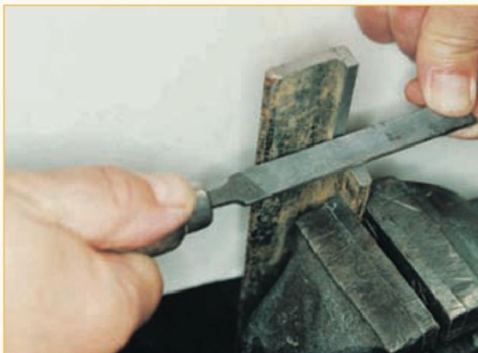
25. Using the safe edge of a file. (Photo by Pauline Loader)
