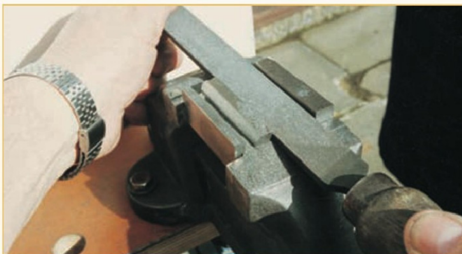
27. The correct grip for heavy filing. (Photo by Pauline Loader)
