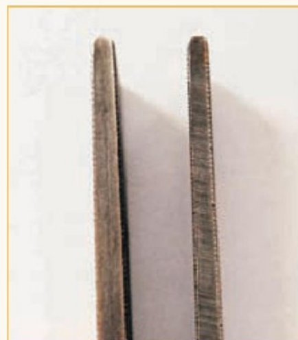
28. Safe edges, one is and one isn't. See text.
