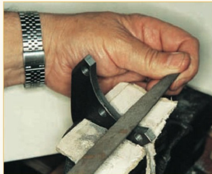
24. Filing a curve with a half-round file. (Photo by Pauline Loader)
