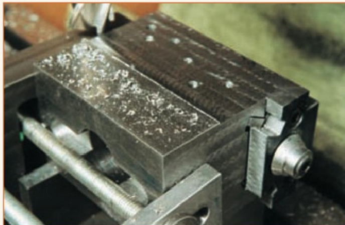
14. Skimming the sides to level up the two parts and improve appearance.
