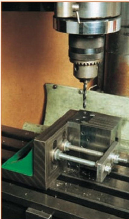
12. With the unit partially assembled, the lead screw nut is drilled with a tapping size hole using the assembled parts as a guide to ensure alignment.
