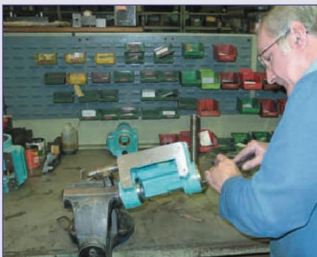
8. Hand scraping a headstock bearing.
