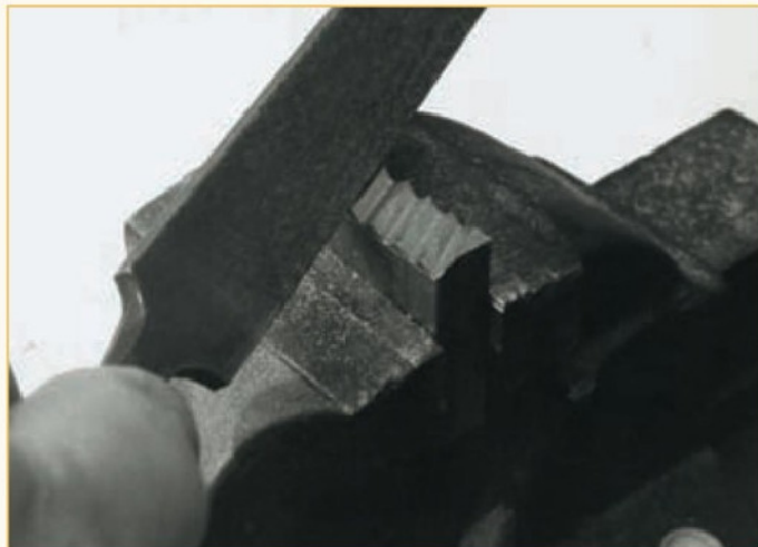
32. Roughing up a surface to make filing easier.
