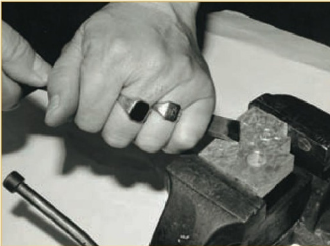
39. A small scraper made from an old file. (Photo by Pauline Loader)
