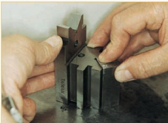
31. A way of checking a filed surface for accuracy.
