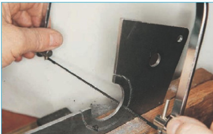
11. The thinnest material a coping saw will manage because of the tooth pitch.
