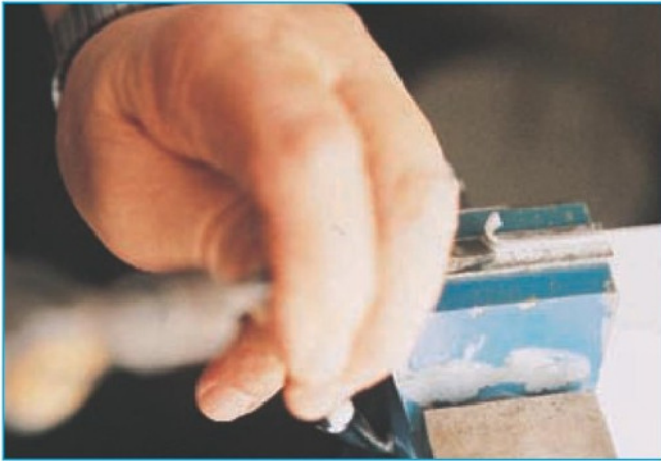
4. Using a chisel against the vice jaw to cut a thin metal. Photo by Pauline Loader.
