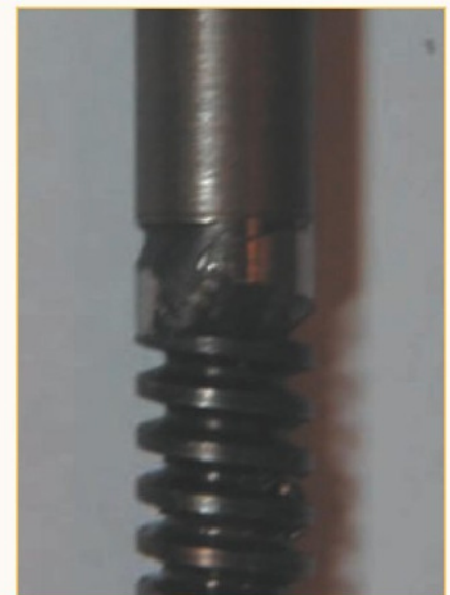
4. The welded joint of the original Acme screw and extension shaft.
