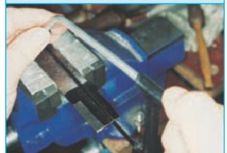
13. Sawing along a line instead of vertically is best for thin work.
