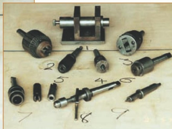
2. The smaller chucks with heavy drilling fitment to rear, and sensitive drilling attachment in foreground.
