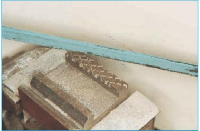
5. Preparing the job in photo.3. by hacksawing grooves ready for chiselling.
