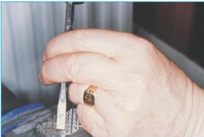
2. Chiselling the waste off a broad surface
