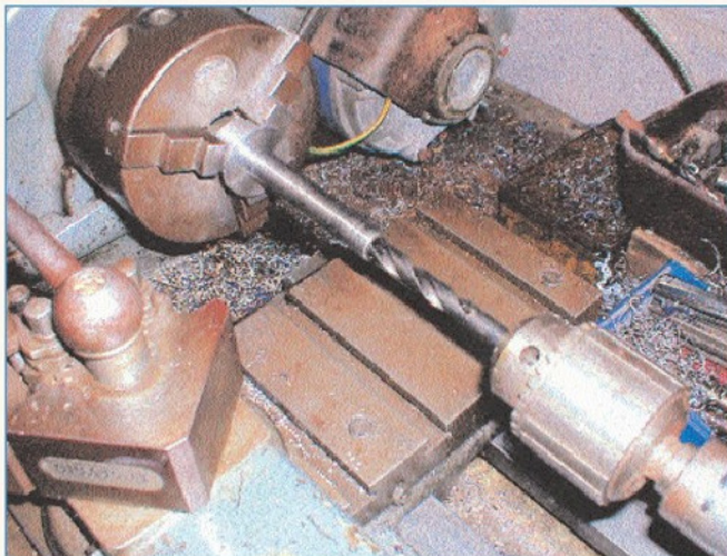
6. Drilling through the sliding tube.
