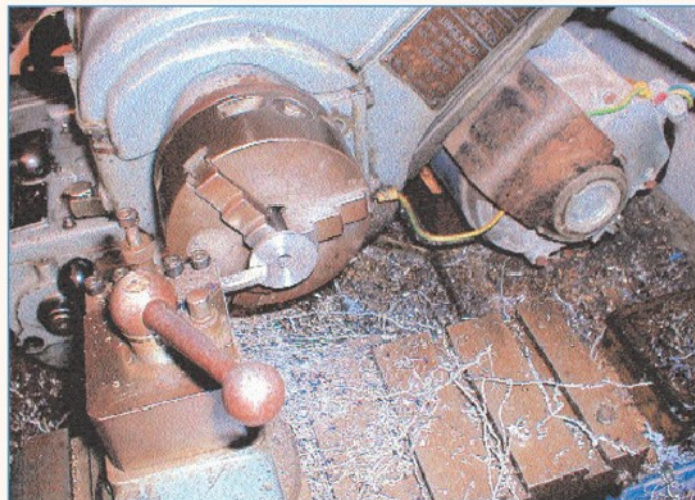
7. Facing the flange on the sliding tube.
