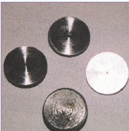
18. Trial result, showing improved surface finish.
