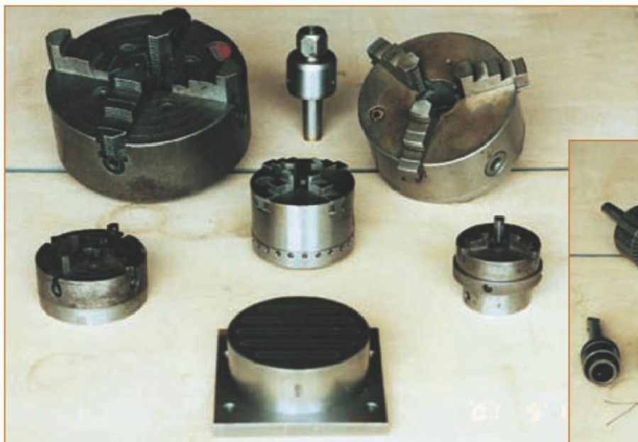
1. The larger commercial chucks and one self built collet chuck.
