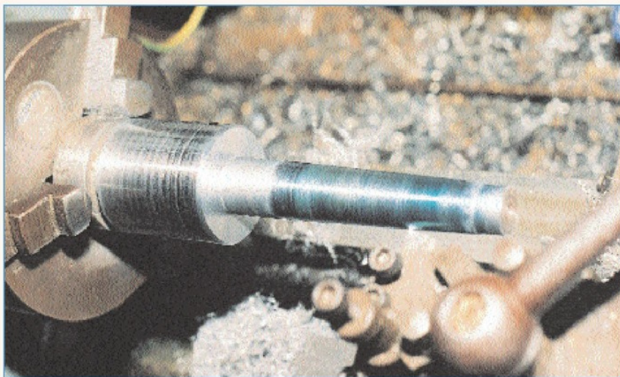
5. Turning the No.2 Morse taper. Note for finishing cuts, the tailstock support was not found necessary.
