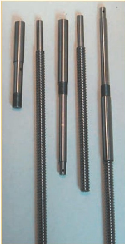
5. The machined ends of the screw shafts and the extension shafts.
