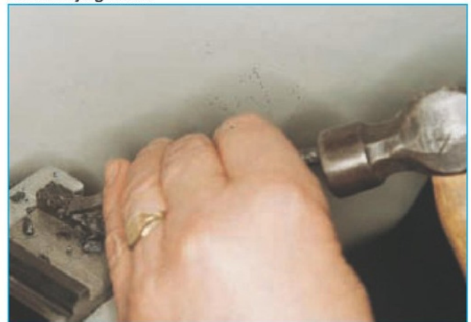
3. Chiselling off a narrow surface, a smear of Vaseline helps stop the bits flying about.
