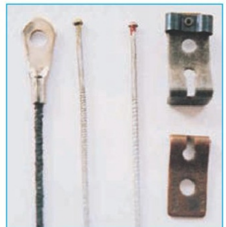
7. A rod saw and two tension files with the clips used in the hacksaw frame.
