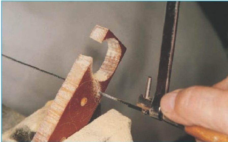
10. A typical use for a coping saw. Photo by Pauline Loader.
