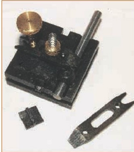
1. Finger plate arranged for cross drilling \frac{1}{8} inch diameter hole in \frac{1}{8} inch diameter rod. Alternative finger and Tee piece also shown.
