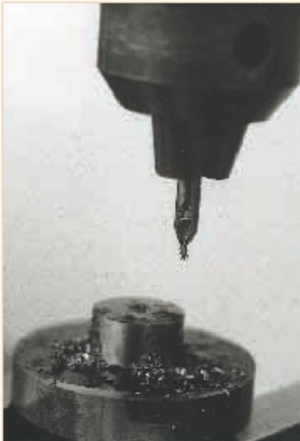
3. The drill guiding spigot set into the planet carrier to ensure that the planet axles are located on the 24mm PCD.
