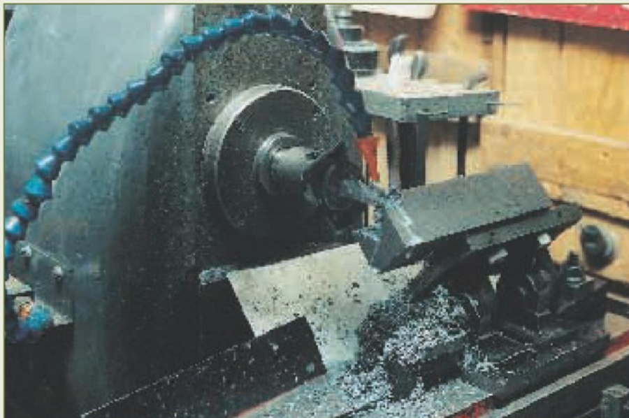
8. Machining the V feature in the guide block
