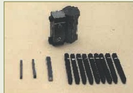
11. Punch holding jig, punches and spacers. Note the ground mark on each punch to help ensure it is used right side up.
