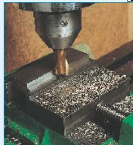
20. Taking a heavy cut (6mm. x 4mm.) using a 16 mm. plain shank cutter fitted in a holder rather than a collet. The chuck performed perfectly.
