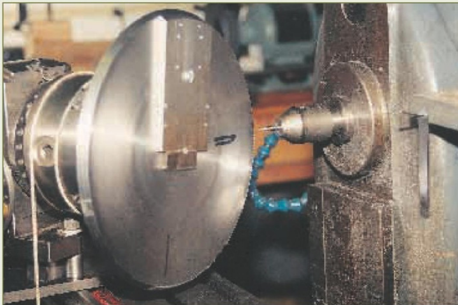
10. Engraving the angle marks
