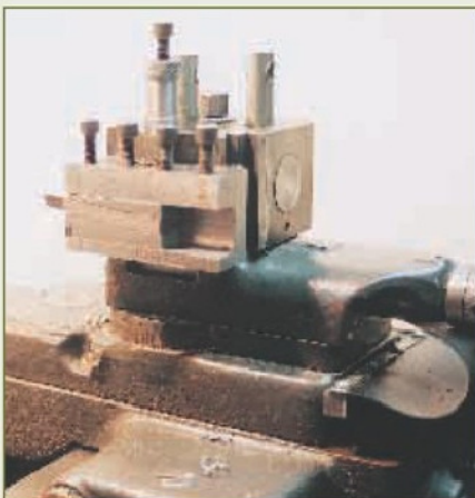
1. Toolholder fitted with rectangular toolbit holder which presents the bit at the specified angle
