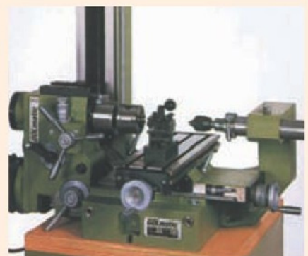
Possibly another near equivalent to the elevating head machines described is the German Golmatic universal machine shown here in Lathe and Vertical Mill configuration. Other setups including Horizontal Mill are possible. The Golmatic is marketed in the UK by Pro Machine Tools Ltd. (tel 01780 740 956)
