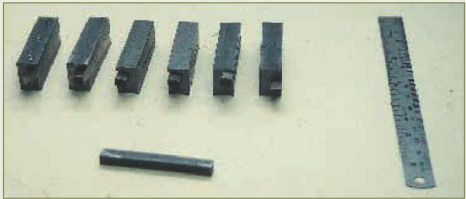
3. Six toolholder inserts for \frac{1}{4} "x \frac{1}{4} " toolbits, covering left and right hand and various rake angles
