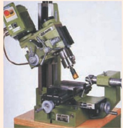
Possibly another near equivalent to the elevating head machines described is the German Golmatic universal machine shown here in Lathe and Vertical Mill configuration. Other setups including Horizontal Mill are possible. The Golmatic is marketed in the UK by Pro Machine Tools Ltd. (tel 01780 740 956)
