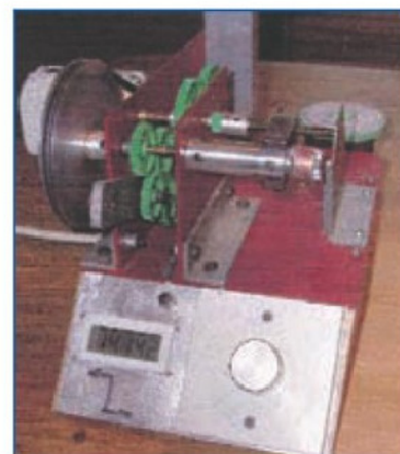
Paul Boothby has redesigned the Myford Quadrant Arm to permit easy swapping of changewheels (see page 38)
