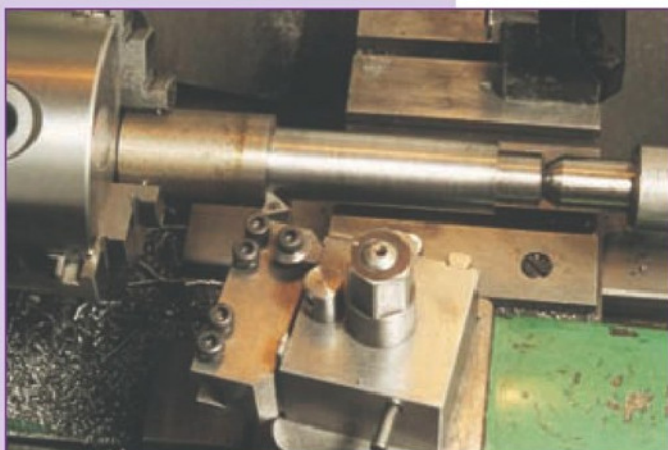
2. Preliminary turning the Morse taper part of collet body.
