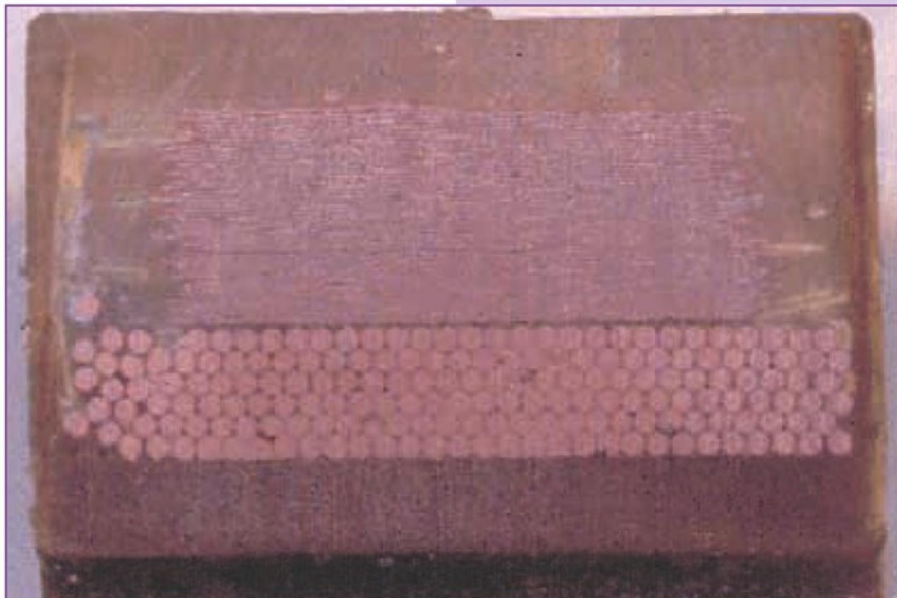
5. A later attempt, still on a Tufnol bobbin but with a greater degree of insulation.
