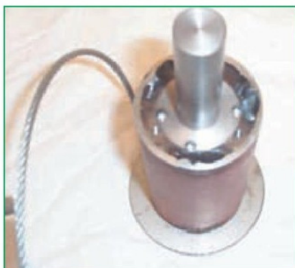
3. Close up of partly assembled drum.
