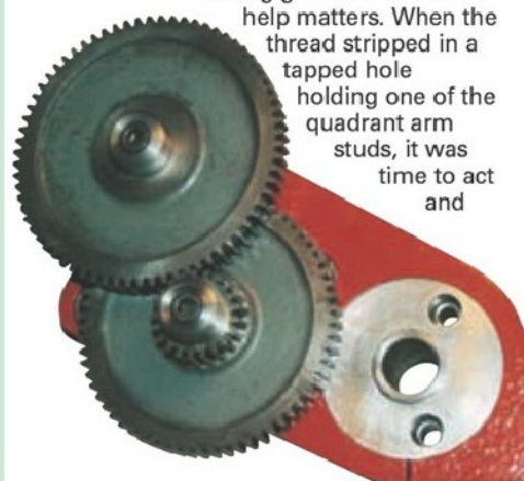
3. The Easychange fitted with changewheels
