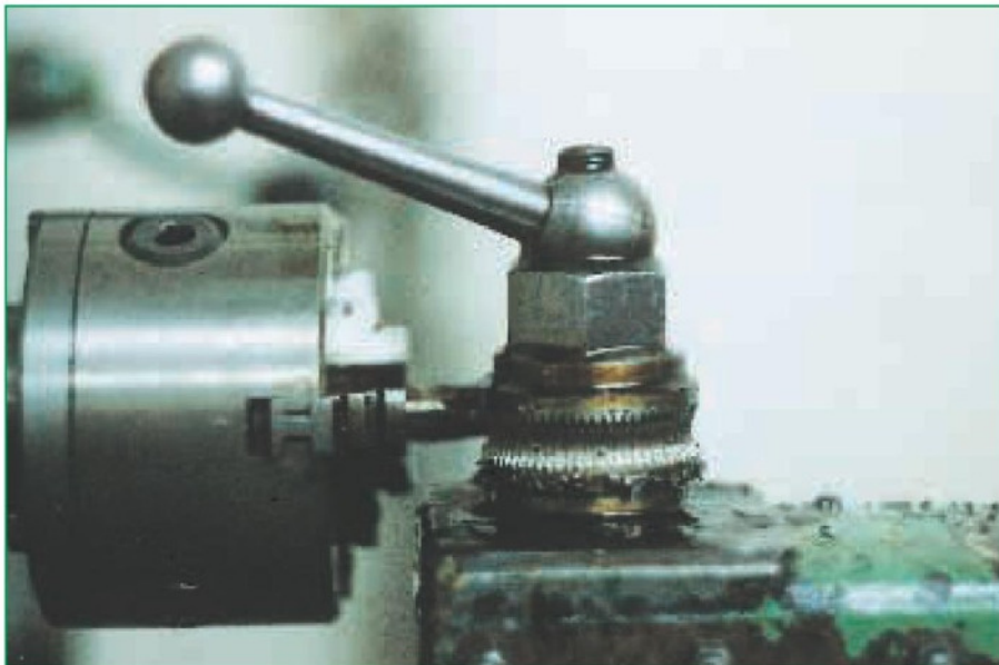
M. Hobbing a Wormwheel in the Lathe
