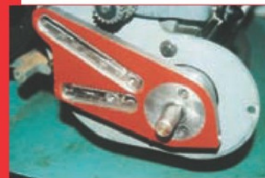
Paul Boothby has redesigned the Myford Quadrant Arm to permit easy swapping of changewheels (see page 38)
