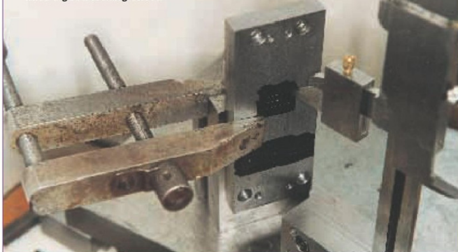
7. Fine threads in the parallel clamp have a good locking effect.
