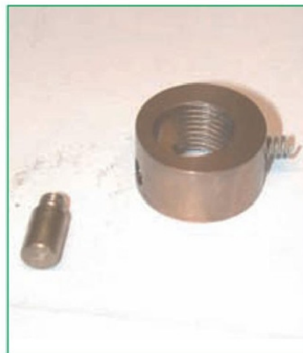
3. Inner nut showing spring and knob and actuator
