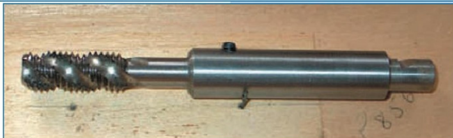
8. An M10 tap needs a slightly shorter holder
