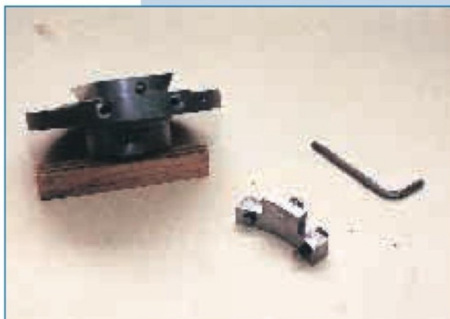
12. The adjuster piece used to take up the leadscrew end play
