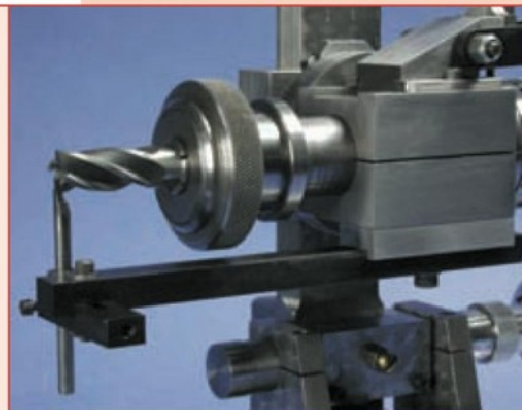
4. The cutter support assembly is a simple arrangement which can be adapted to accommodate a number of forms of tool rest (Photo. Mike Chrisp)
