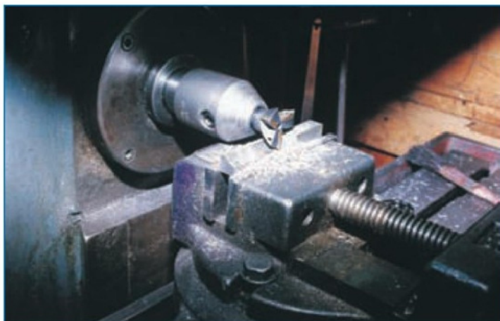
11. Making the angled support piece used to support the gib, as shown in Fig. 10. Again the same dovetail cutter is used
