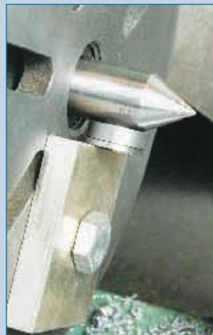
9. Using the width gauges (see Issue 73), to set the position of the arm supporting block seen in Photo. 8
