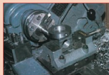
3. Boring the spindle hole on the collet head
