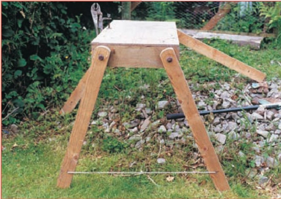
2. A portable bench with all four legs independently adjustable, here set up on a pile of rubble to illustrate why it can be used almost anywhere. Notice the locking pliers clamped to the worktop, as might be used for lighter jobs. The removable cords seen near the bottom of the front legs have been found to be a valuable asset when deploying the legs on fairly level ground.
