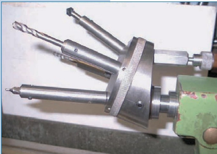
6. The varying tool stand-outs are equalised by means of purpose-made tool holders
