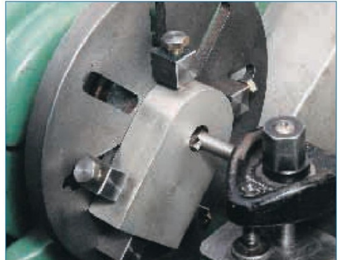
3. Faceplate dogs being used to clamp a large bearing block
