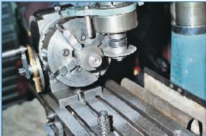
4. Gashing the worm wheel prior to hobbing
