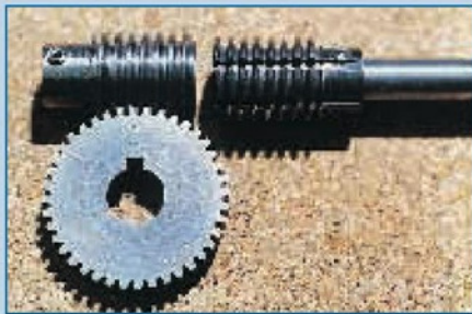
1. A finished worm and wormwheel and the hob used to form the teeth on the wheel
