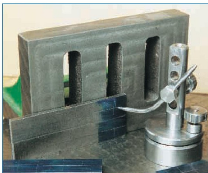
7. The mini surface gauge described in Issue 68 being used to mark out some of the parts for the knurling tool
