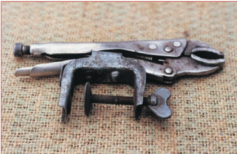
4. Worth its weight in gold, this table edge clamp allows you to mount any appropriately sized set of locking pliers on to any handy solid structure. Occasionally found for sale in the better hardware stores.
