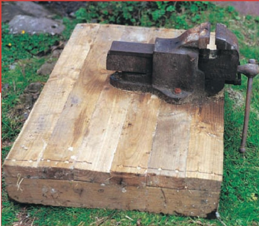
1. Deliberately made to be near the limits of portability, a 'vice on solid four by two base' assembly that can be used flat on the ground, as seen here, on fold-away legs, or on a free-standing base. While it is really a two-man job to carry it about (make sure you get the light end!!), it can be 'walked' on its corners
