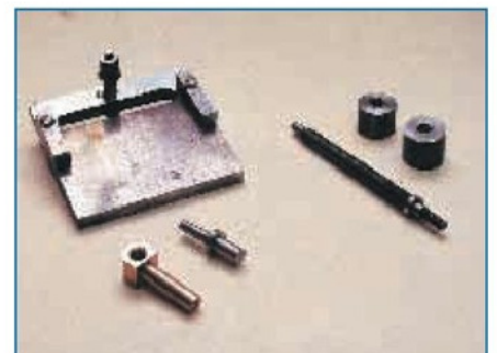
18. The completed nut with its gauge and jig, beside the leadscrew
