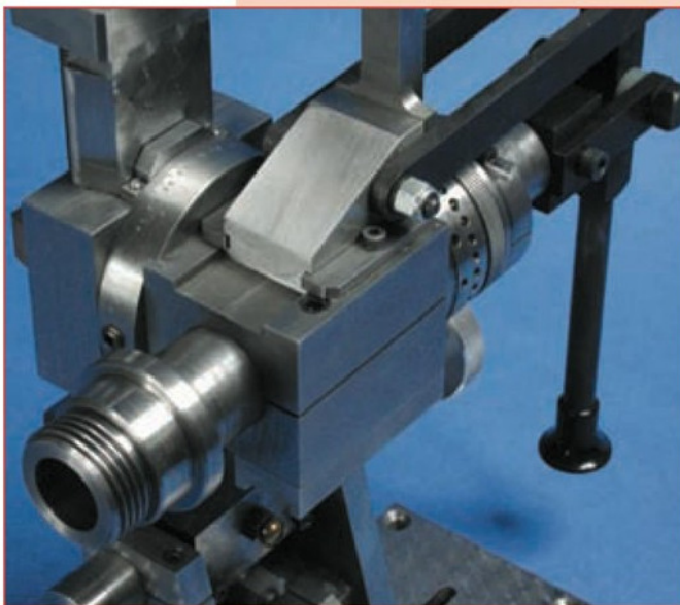
2. The head houses the spindle collet holder which features a 2MT socket capable of housing Myford collets. Other methods of holding the cutter to be ground could be incorporated to suit the builder's needs (Photo. Mike Chrisp)
