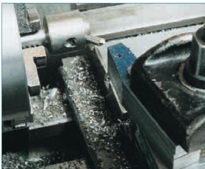
10. Fly cutting the arms whilst held as a pack on the top slide
