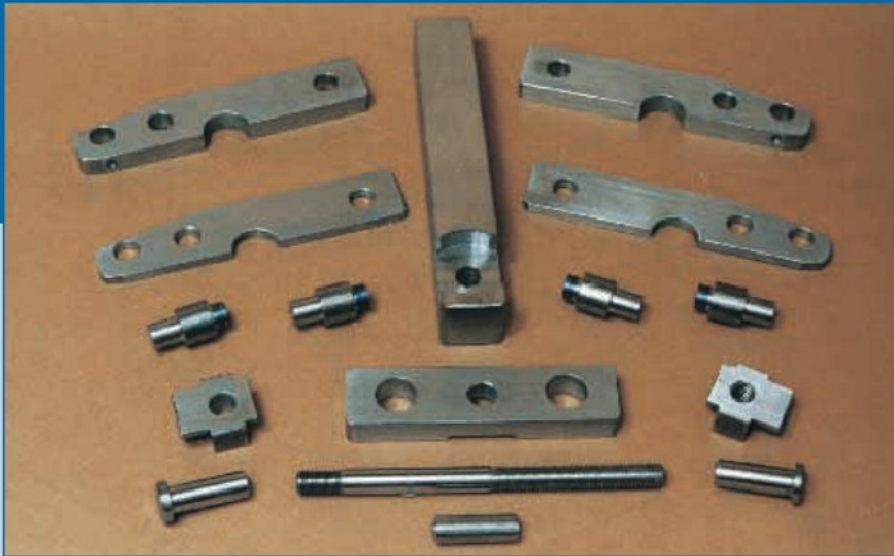
1. The parts that make up the knurling tool with some features being incorporated with the use of the faceplate particularly in mind. Typically the recess in the mounting bar, centre top of the picture
