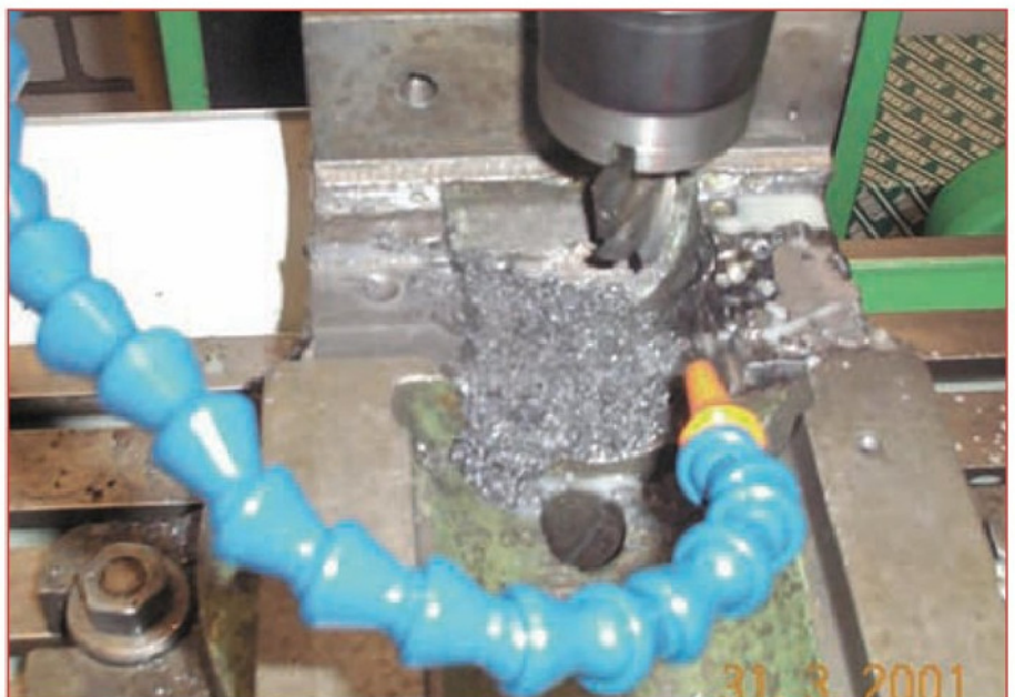
3. Machining the recess for the insert
