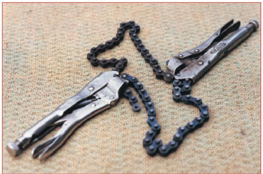
3. Chain clamps can be assembled in series to get a powerful 'high modulus' grip on almost anything. A recent application was to hold substantial flanges onto a dead tree trunk while the whole was jacked out of the ground. For some jobs, lots of tight turns using luggage ('bungee') bands can be even better.
