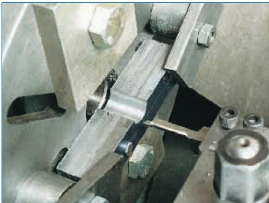
8. Making the half-round recesses in the arms; note the supporting block just visible below the arms
