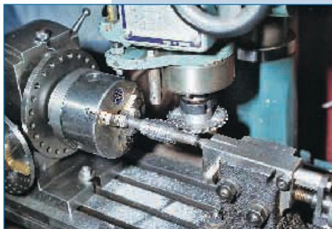
3. Gashing the hob to create the cutting teeth
