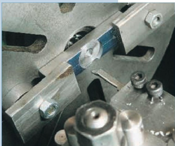
6. Recessing the cross bar. A similar operation to that required on the mounting bar but the set-up here is much simpler, as the assembly is automatically balanced
