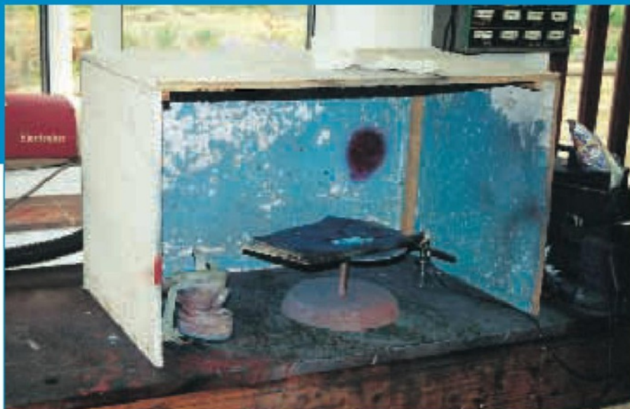
1. A general view of the cabinet. The vacuum cleaner is on the window sill while in the cabinet are the cake turntable, liberally covered with the Financial times, air brush to the right and face mask on the left
