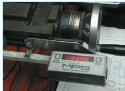
4. Digital read-outs fitted to the milling machine have proved invaluable when machining complex components from the solid
