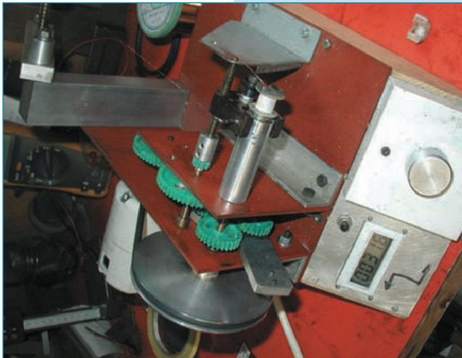
9. The winder constructed to facilitate the winding of the magneto coils. The secondary windings consist of 18000 turns of 0.0011in. dia. wire
