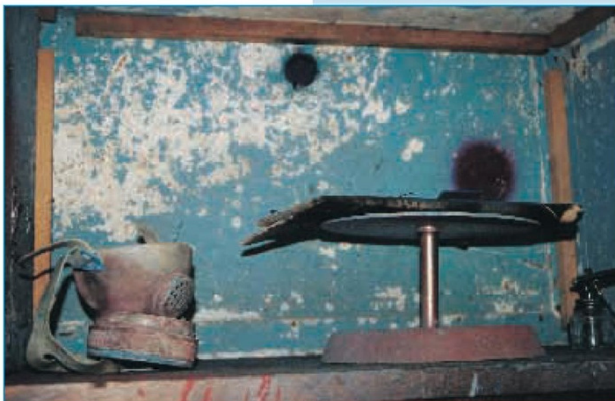
2. Looking up inside the cabinet, shewing the crude construction and vestiges of emulsion paint from its former existence. The red splodge is from a previous test run of paint, while the bluing around the vacuum outlet is obvious
