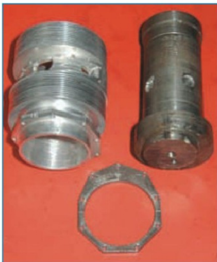
8. An Aquila cylinder barrel shown with the eccentric turning mandrel on which it was made and the barrel to crankcase securing stud hole drilling jig
