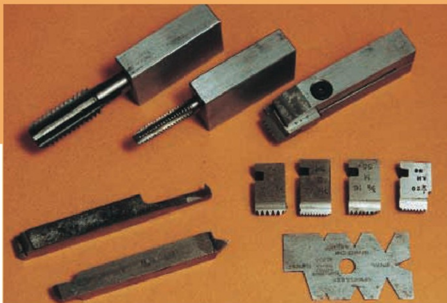
1. A selection of tools for screw cutting on the lathe including modified taps and individual die head chasers
