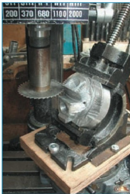
2. A test piece for the Hydra cylinder head being used to determine the process for machining the cooling fins. Brian has commented that he is still not certain how the full size heads were produced
