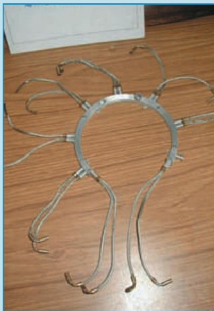
13. The Aquila ignition harness. Two plugs are fitted to each cylinder, independently energised by the pair of magnetos
