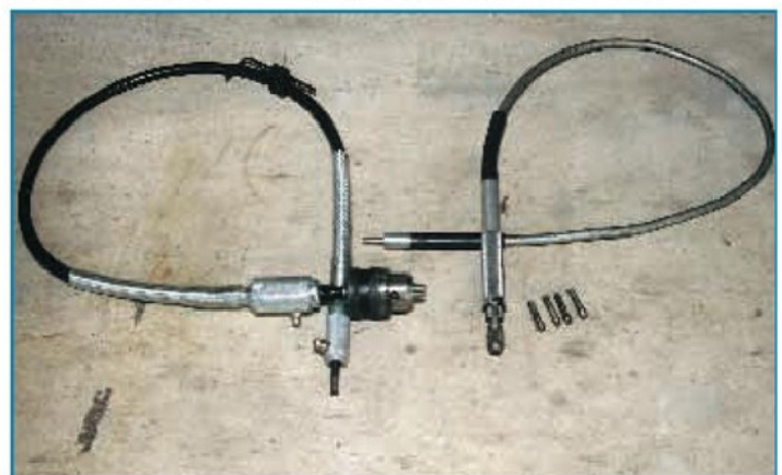
3. Flexible drives. The handpiece on the right has a movable sleeve to keep fingers away from the chuck
