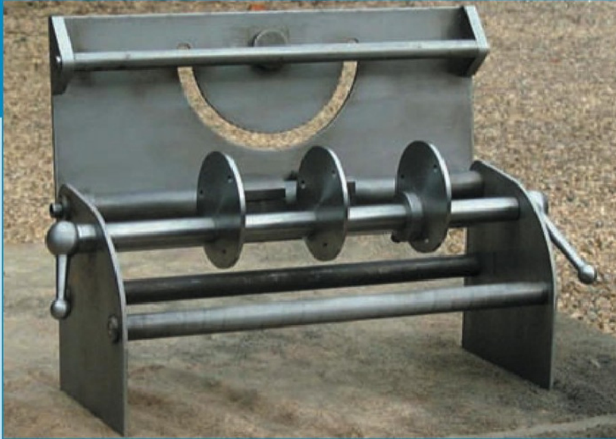
1. The revised table assembly, showing the new cam arrangement. The table now pivots at the back (i.e. on the side remote from the grinding wheel) rather than the front. Ball lever handles are used instead of knurled knobs, a modification which may be considered desirable by all Worden owners
