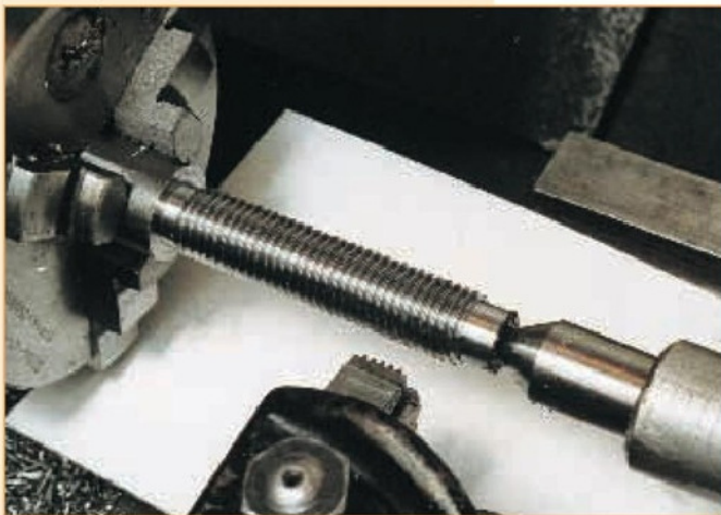
5. The thread now finished, using a die head chaser, shows a much improved thread. The thread could have been cut fully with the chaser as there is no need to use a single point tool to start the thread.
