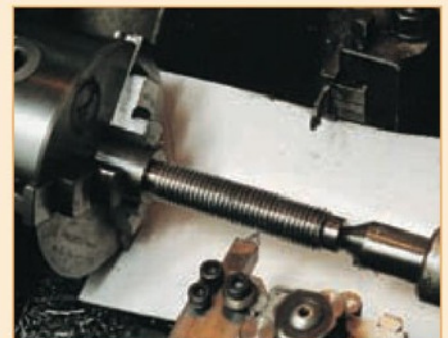
4. An almost completely cut thread having been produced with a single point tool.
