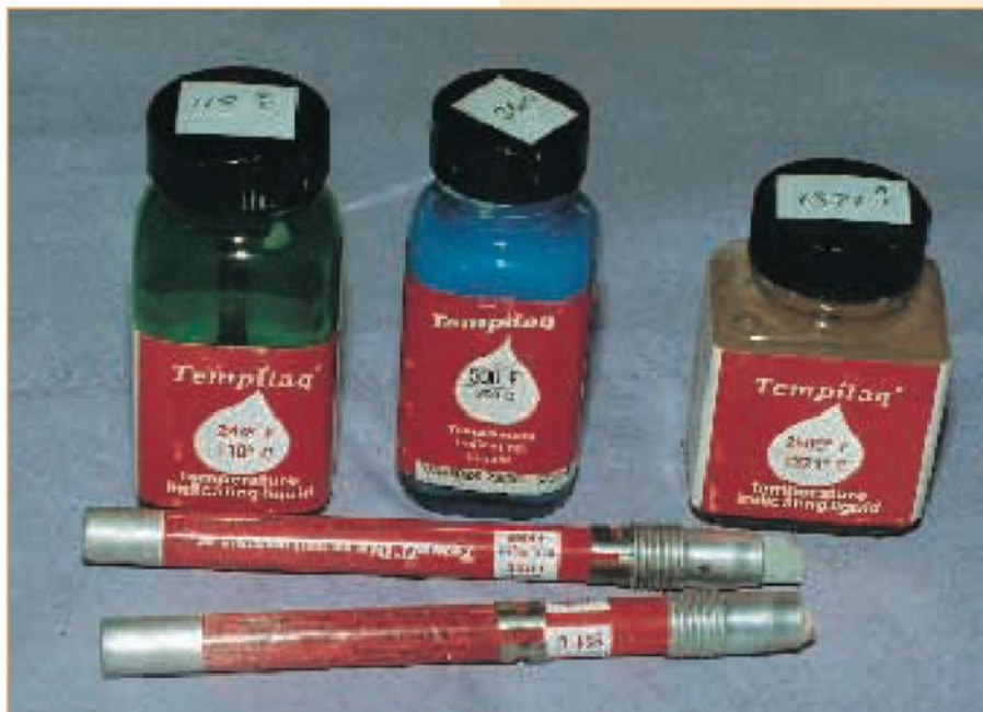
3. Tempilaq paints and crayons which are used to indicate, by melting, when a particular temperature has been reached
