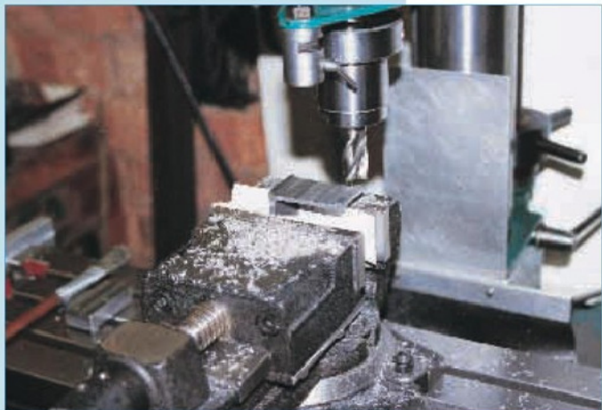
6. Milling the guide slot in the limit switch bracket
