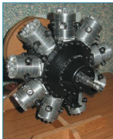
6. The 1/4 scale model of the nine cylinder 'Bristol' Aquila sleeve valve radial engine which won the Duke of Edinburgh Trophy at the Model Engineer Exhibition at Sandown Park
