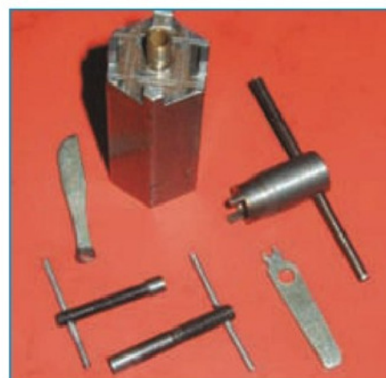
16. Assembly of the complex units requires miniature versions of the special spanners used in full size
