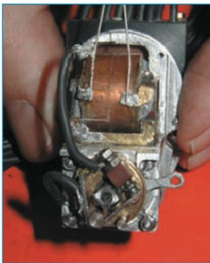
12. A view of the magneto coil and contact breaker. After winding, the coils are vacuum impregnated with epoxy resin
