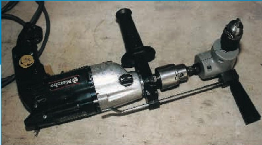
1. A right angle drive unit fitted to a portable drill, locked in angular position, with the drill depth rod engaging a hole in the attachment block
