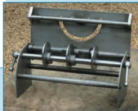
2. The bar attached by brackets to the front of the table bears on the cams. It serves the same purpose as the sheet metal angle section spot welded to the table on the later versions
