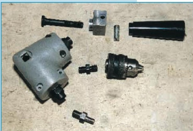
2. A right angle drive unit which had the bolt, handle and double threaded adapter supplied. The chuck, single threaded adapter, attachment block and screw are additions
