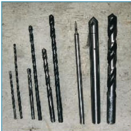
6. Jobbers and long series drills ( 1/8 , 3/16 , and 1/4 in. diameter) shown alongside a 1/2 in. diameter jobbers drill to illustrate relative lengths. Also shown are an extended centre drill and an extended countersink.
