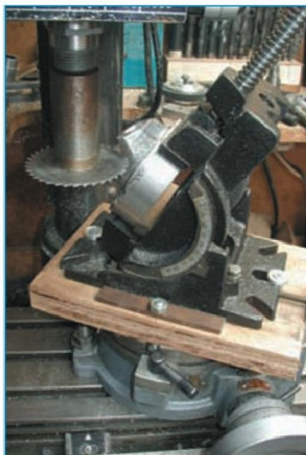
3. Another view of the set-up on the 'Warco' milling machine showing the simple base, attached to the rotary table, used to vary the radius of the cutting path
