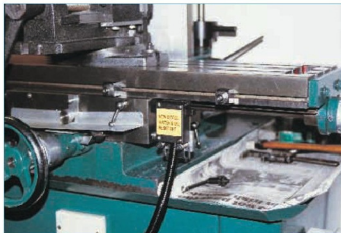
7. The limit switch shown in the raised position, ready for powered traversing
