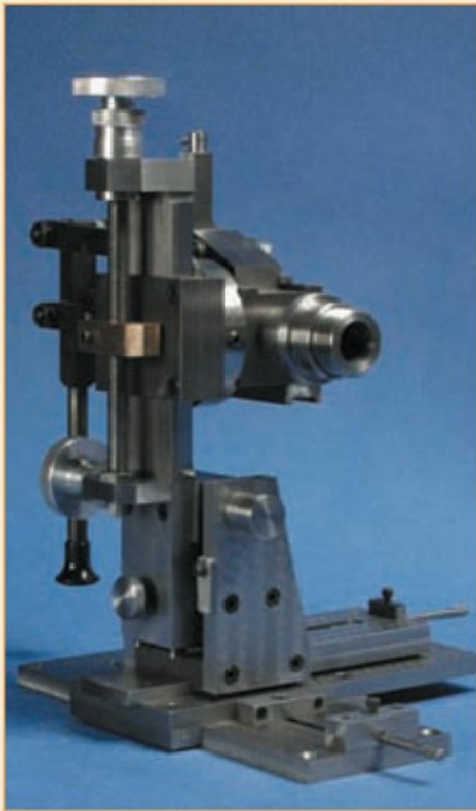
4. The Pivot Pillar Assembly, showing the feed screw and its mountings (Photo. Mike Chrisp)
