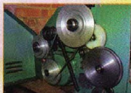
3. Headstock spindle drive is either direct from the motor pulley or via the countershaft. The leadscrew gearbox is driven by the train of gears to the right.
