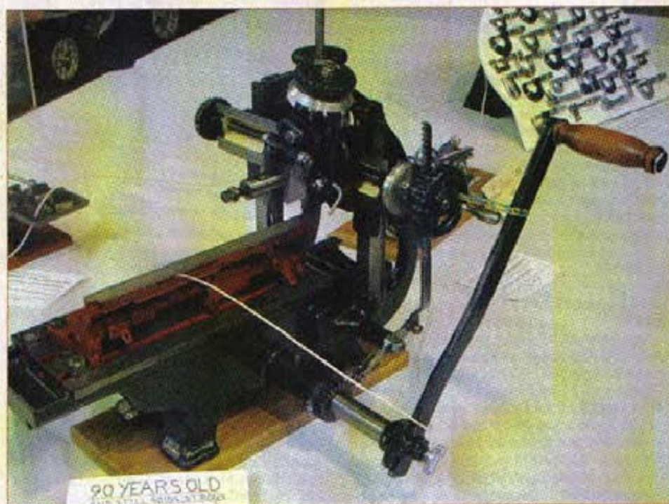
5. D. W. Clennel's hand planing machine was made by toolmaker Arthur Firth at the Atlas Works, Cleckheaton over 90 years ago.
