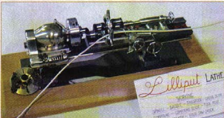
3. A recruit to the ranks of miniature machine tool builders is J. M. Clennel who entered this 1/20 scale version of a centre lathe, seen here with a small four-throw crankshaft mounted between centres.
