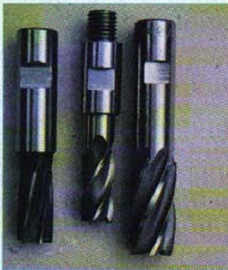
3. The sleeved-up cutter is the threaded one in the middle
