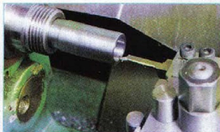
11. Boring the end of the Morse taper to take the die holder shanks
