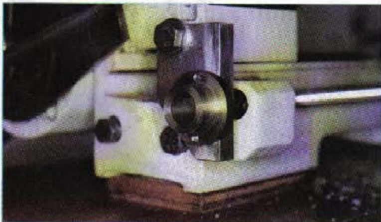
7. The quadrant bracket, 'in the rough', being tried for position
