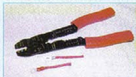
6. Crimping tool for the attachment of terminals to electric wires. Two examples in the foreground
