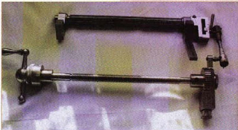
4. The saddle and ram assembly, fitted with the gear in its housing and the operating lever assembly
