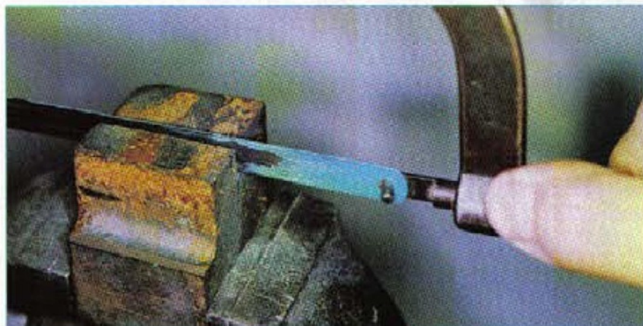
12. First stage in making the raising block
