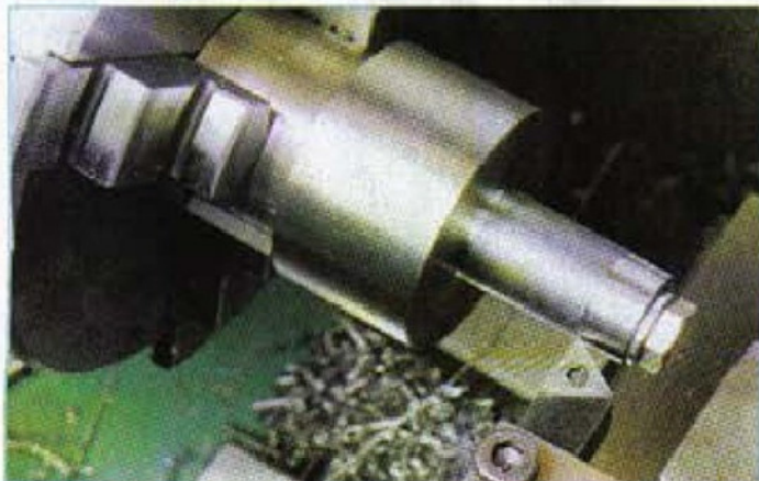
8. The larger holder shank being finished turned whilst held on a mandrel after boring
