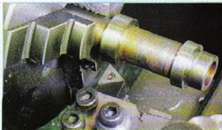
9. Turning the test piece for setting the top slide to the correct angle for machining a Morse taper
