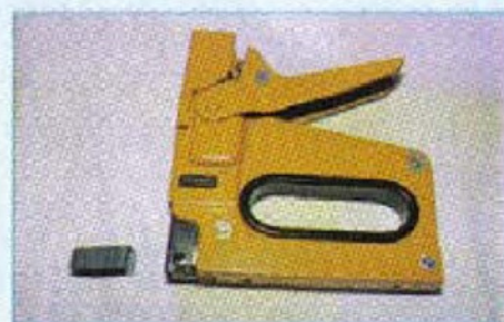
5. Workshop staple gun to fire staples into hard material such as timber. Collated staples seen at left
