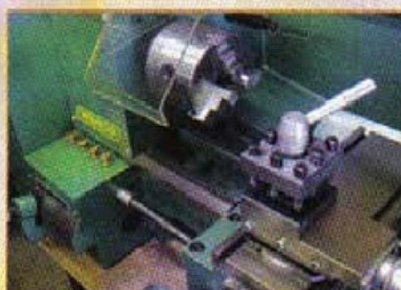
2. The 918 is supplied with an integral screw-cutting gearbox and a four-tool turret.
