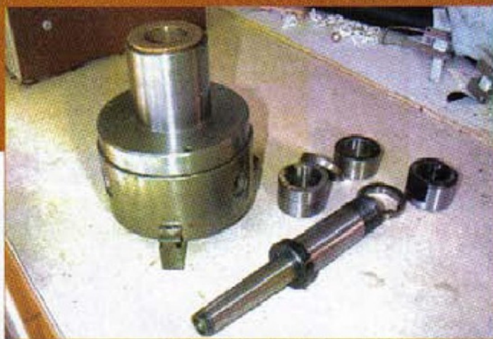
2. The chuck with the new backplate fitted and the No. 3MT mandrel. The spacers and nut are required when the mandrel is used for its original purpose - the mounting of side and face cutters
