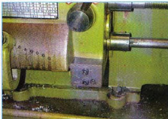
3. The left-hand mounting block for the trigger bar. This will have to be designed to suit the lathe to which the unit is to be attached
