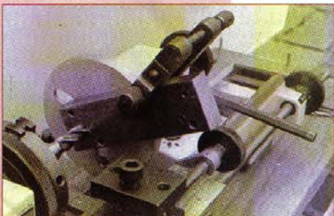
11. One clamp used correctly will hold work for counterboring
