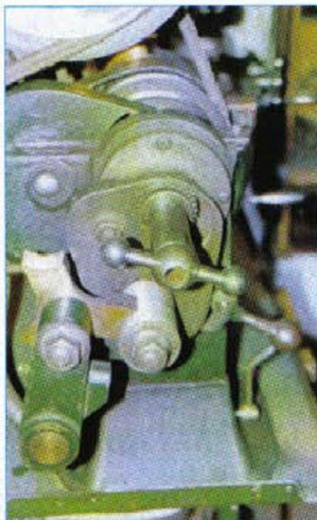
42. The 'hob' and follower of the lathe shown in Fig. 40
