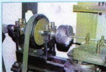
11. Headstock with division plate of lathe shown in Fig. 10
