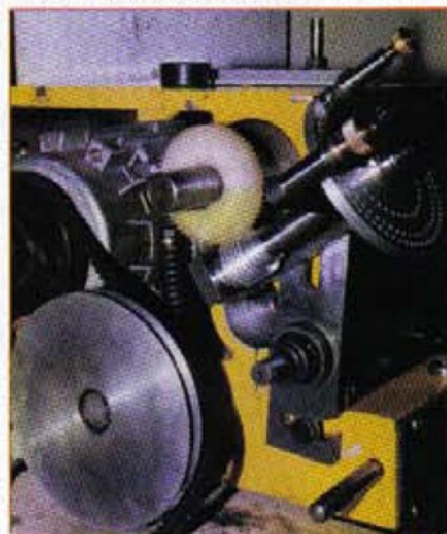
1. The unit bolts to the rear of the Hobbymat headstock, pivoting around the leadscrew bearing
