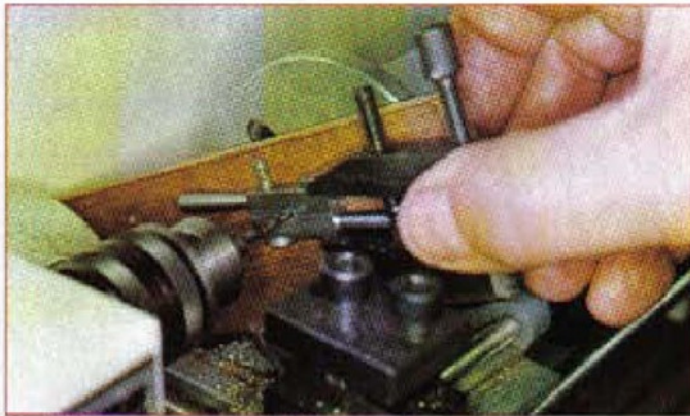
3. Drilling using a parallel clamp as a hand vice
