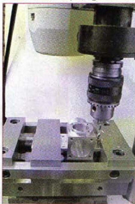
2. Drilling with the vertical head and fabricated vice
