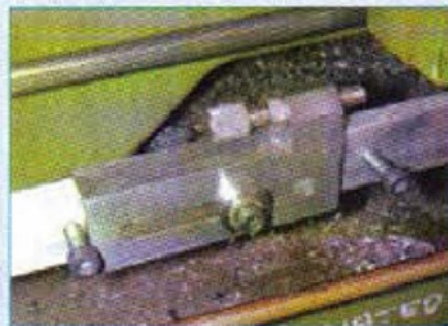
6. The trigger stop on the mounting bar. The clamp bolt hole positions may need to be adjusted to suit requirements
