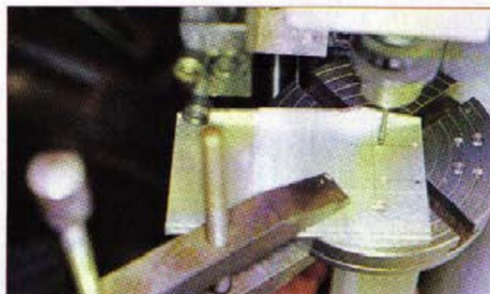
10. Thin work must be clamped to avoid spinning
