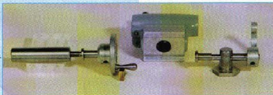
10. Tailstock components. The eccentric lock gives a firm grip on the bed
