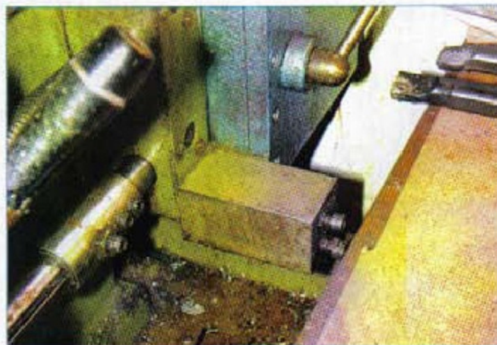
4. The right-hand mounting block will have to be tailored in a similar manner
