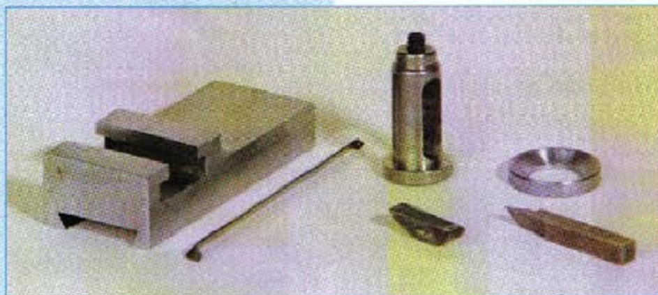
9. The cross-slide and toolpost components. The method of locating the corrugated stainless steel glib strip is evident
