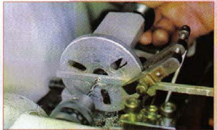
4. Simple shape - simple clamping
