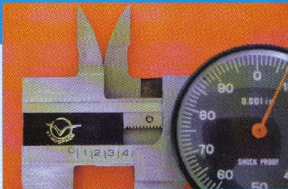
1. The internal jaws of a small dial caliper provide one of the most convenient means of measuring the width of external grooves
