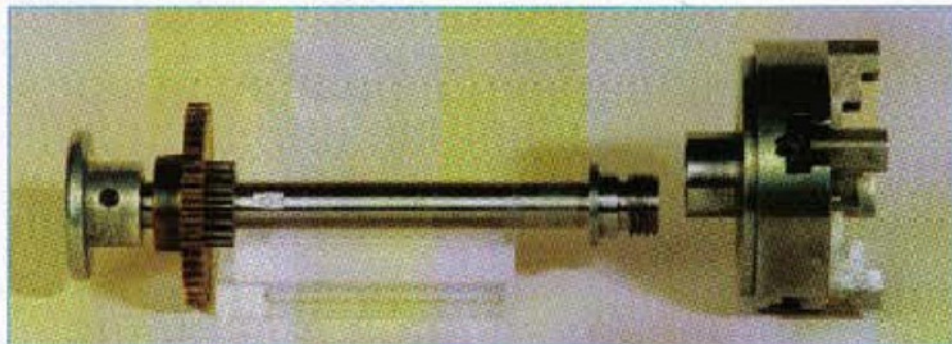
3. The headstock spindle, complete with the leadscrew drive gear cluster, shown with a 4-jaw independent chuck
