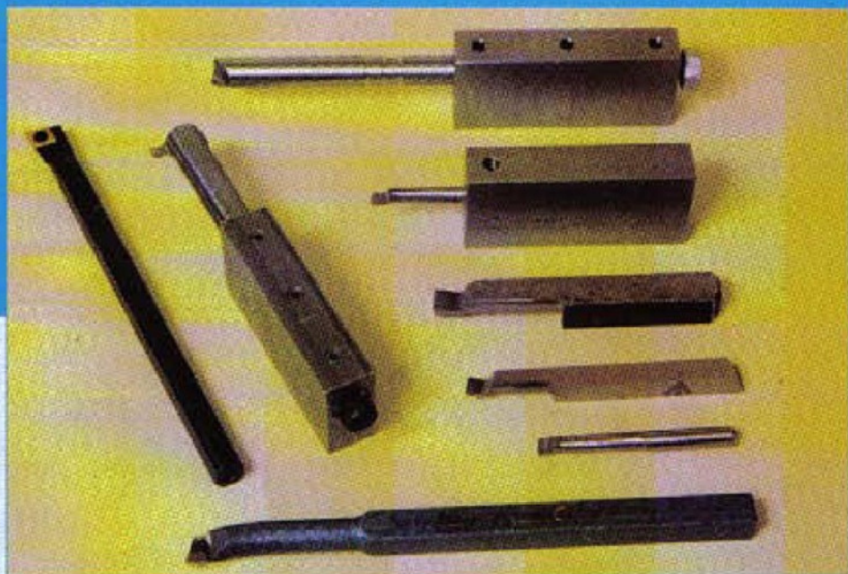
1. Even for basic boring, tool requirements vary depending on diameter, depth and material. This results in far more tools being required than for simple external turning
