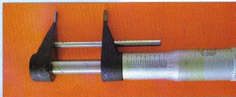
2. Slightly different in design to the groove measuring micrometer shown in Drawing 2, this instrument has a range of 1.2in. to 2.2in. It can also be used to measure the bore of holes or the inside diameter of tubes
