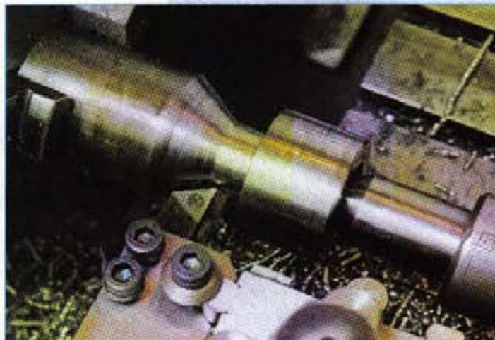
4. The first stage of creating the shank of the smaller holder using a left-hand knife tool. Note the support of the tailstock centre
