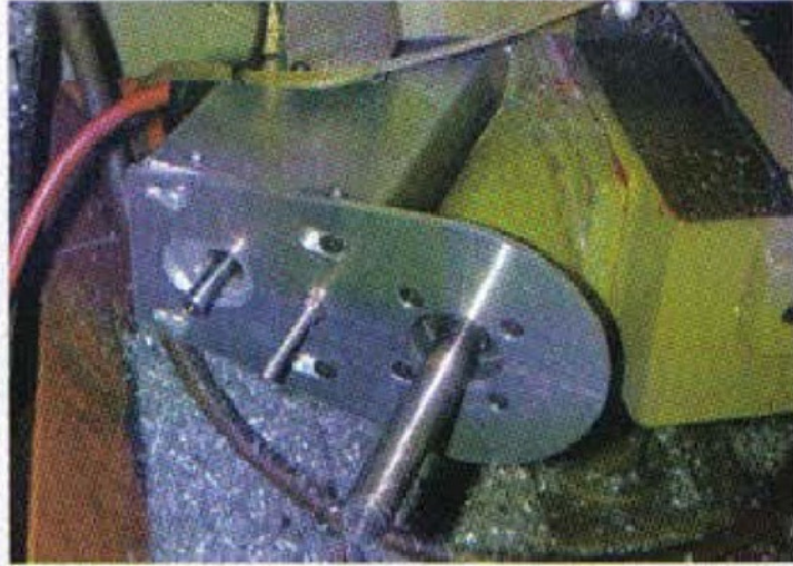
3. The new back plate fitted by means of the four countersunk screws
