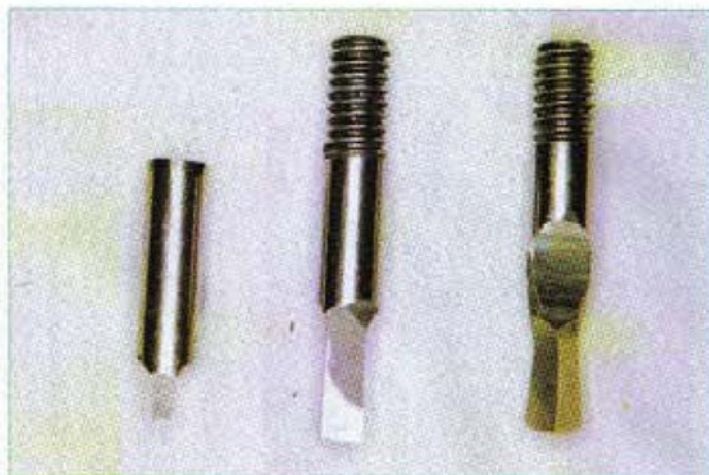
10. Cutters made from broken end mills
