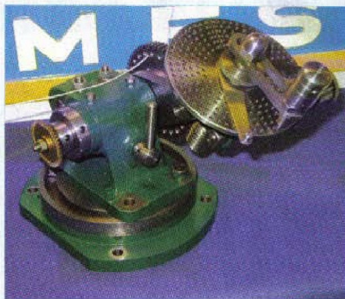
23. Another version of the Versatile Dividing Head was also to be seen on the St. Albans stand. This interesting variant, mounted on a swivel base was by John Caldwell
