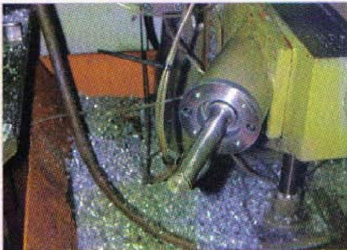
2. The modified bearing retaining plate. The article was written and the photos taken some while after the modification had been completed and while another major project was under construction - hence the swarf!
