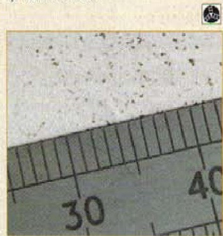
4. These dust-like particles were produced whilst reducing an outer diameter by a very small amount. The larger specks are multiple fragments.
