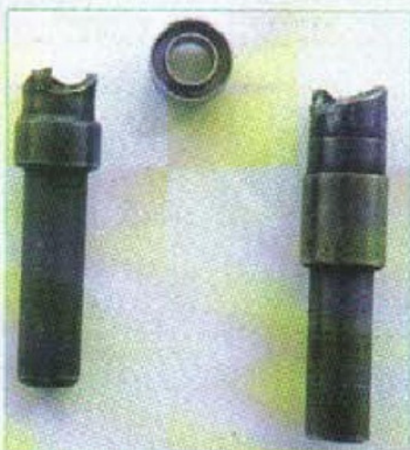
8. Ring cutters and the component cut by them
