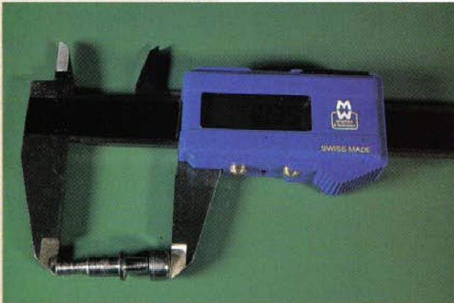
2. A digital vernier caliper is a versatile precision instrument which will suffice until more specialised equipment can be afforded
