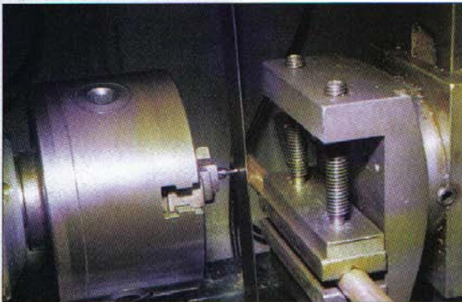
3. Setting the centre height in preparation for cross drilling
