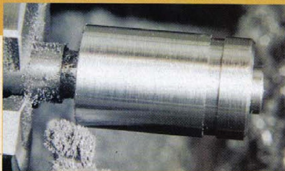
1. When using a tool with a very fine edge and a very shallow cut (in the order of 0.0005mm) grinding dust-like swarf is produced. The tool is in need of demagnetising
