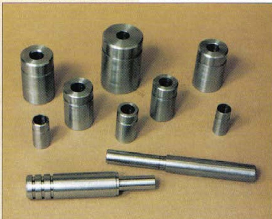
3. The finished hole gauges which need to be made to very precise diameters
