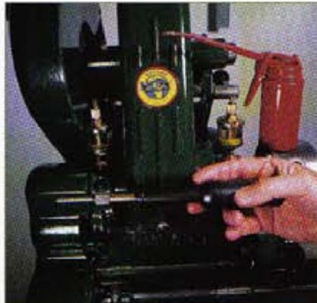
6. The Myford oil gun is designed to suit the nipples fitted to the oiling points
