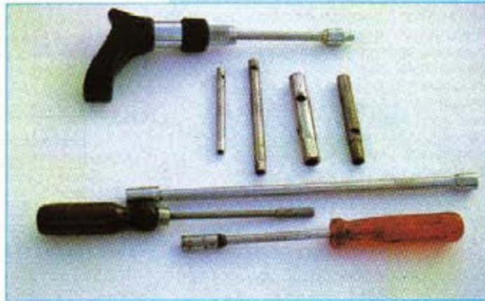
2. Box spanners and socket spanners, all commercial examples with their own disadvantages.
