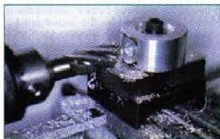
4. Using the larger chuck for the 9/16 in. end mill
