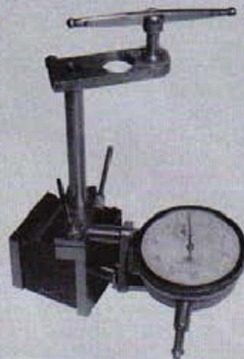
6. The device seen on the machine vice in Photo. 3 is this versatile magnetic clock stand equipped with a variety of fittings to aid workpiece alignment
