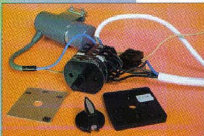
12. A sound suggestion is to wire up the electrical components before trying to fit them in to the plinth
