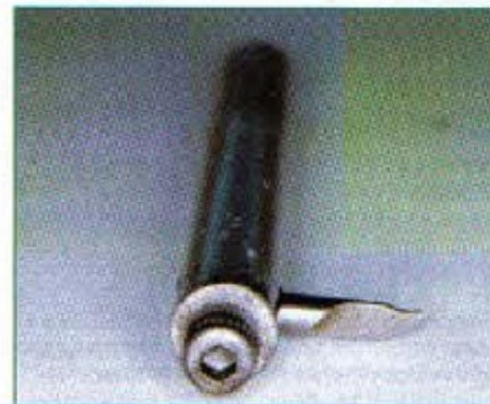
16. A fly cutter used for cutting thin slots
