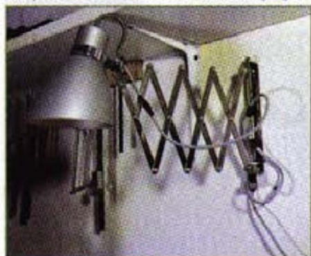
1. A good light on a properly engineered extending arm is invaluable because it can be quickly positioned to illuminate the working area
