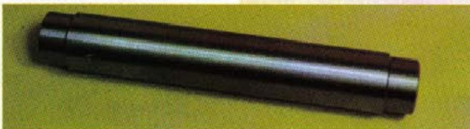
3. The test bar, turned between centres, will, after having been made to prove the tailstock's accuracy, find other uses in setting up the lathe. Treat it as a precision item and store away safely.
