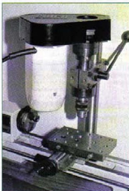
5. The milling table in position and the (not very good) drilling and milling head cutters with helical teeth will cut better than those with straight ones, because they have side rake as well as top. For the same reason hard brass and brittle materials will do better with straight fluted cutters. Slot drills have advantages, due to the way they cut all across the centre, which
