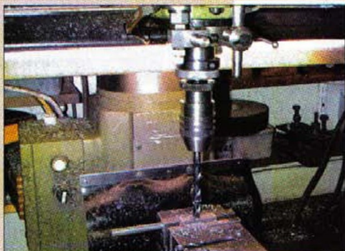
8. The large drill just fits when in the fully closed position
