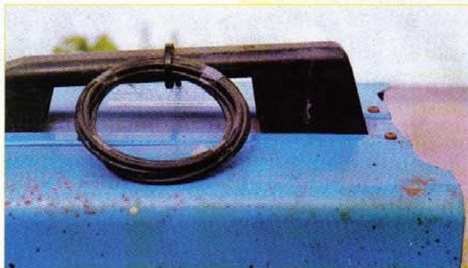
6. When purchasing your first batch of replacement copper tips, it is a good idea to purchase a low friction wire feed tube. Fasten it to the carrying handle of the welding set so that when you need it, months or years later, you will know exactly where it is.
