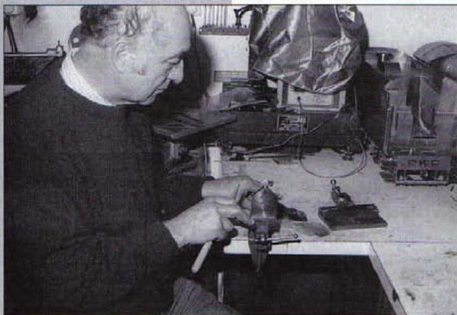
11. When we visited Derek he was putting the finishing touches to a small precision lathe tool honing jig
