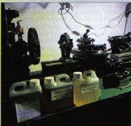
5. The range of oils required to keep the lathe in good order and to aid machining
