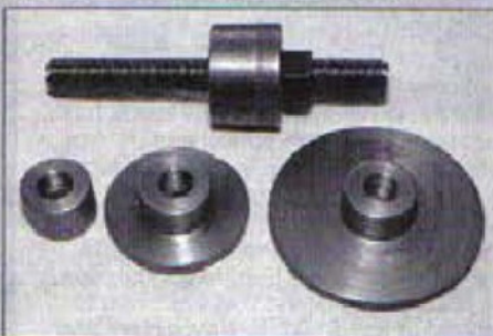
2. Caps, each stamped with its length addition when screwed on to rod
