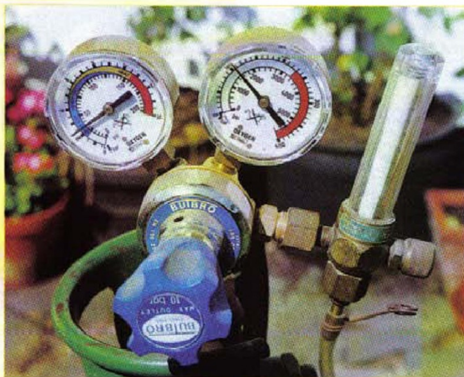
4. This type of gas regulator tells you how much is left in the bottle, allows you to adjust the value of the low pressure side of the system, tells you what that LP value is, and allows you to do fine adjustment to the flow rate.
