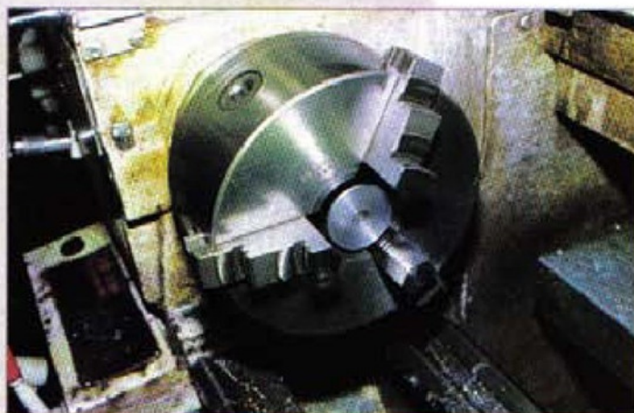
4. Flanged stop rod positioned with 3-jaw chuck
