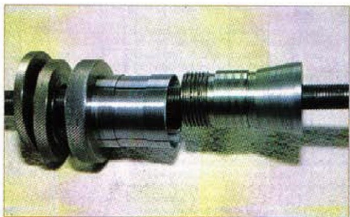
5. Separated components - 1/2in. NF locknut, 3/4in. BSPF draw-in nut, sleeve &amp; nut
