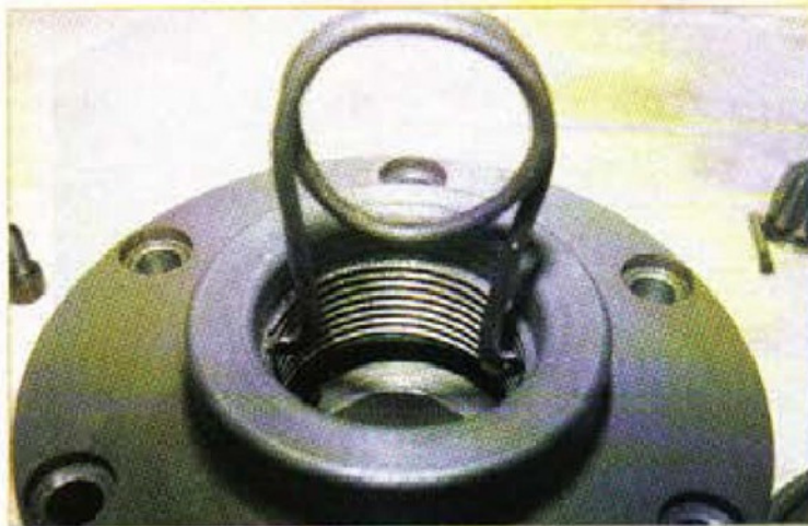
3. The home-made wire tool being used to clean the backplate threads
