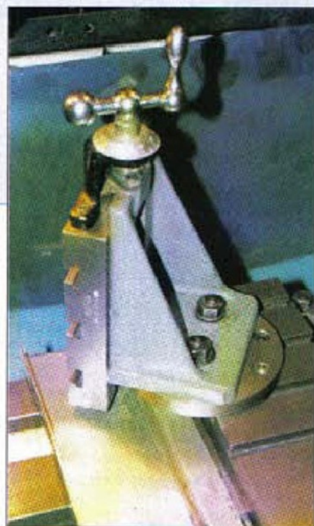
3. With the mount positioned at the extreme left of the side of the boring table, the vertical slide can descend below the top surface
