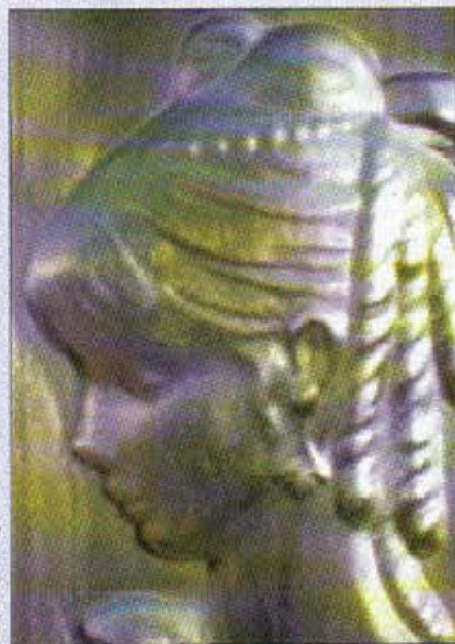
3. 3D cameo mould programmed using MillWizard by Delcam (machining time 6 hrs 49 mins)
