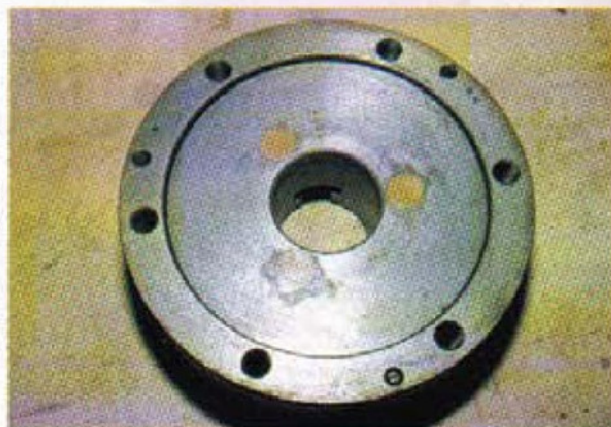
8. After assembly, the location casting holes have been puttied
