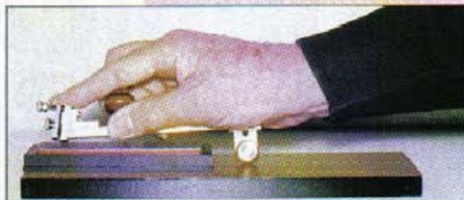
5. The grip adopted while tool edge is moved to and fro over the hone.
