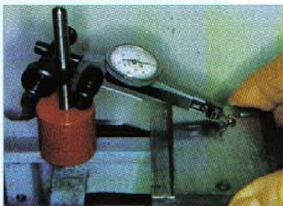
16. Another alignment check using the magnetic base on the lathe bed
