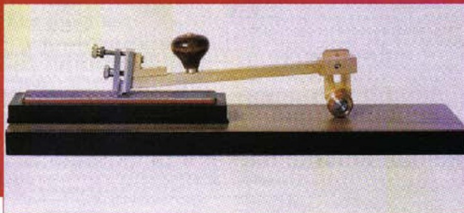
1. The diamond impregnated honing plate is supported above the baseboard to achieve the correct geometry
