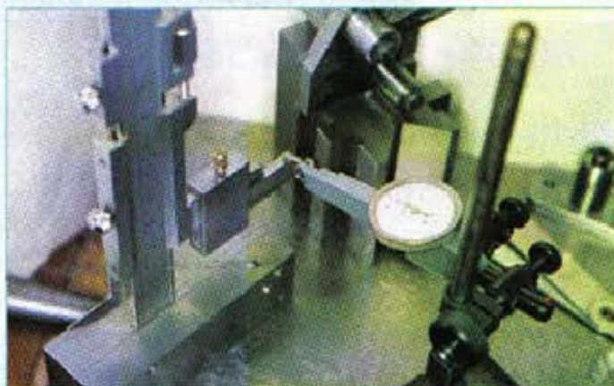
18. Making use of the clamping gear from the magnetic base, on a small scribing block, to measure the height of a button
