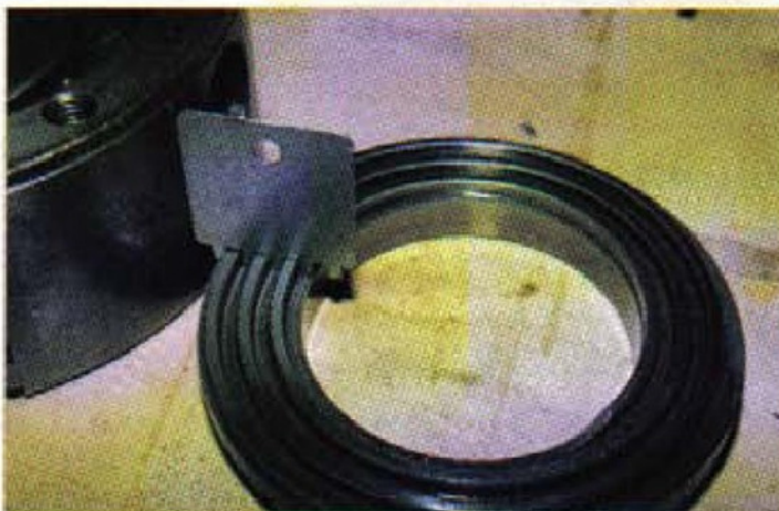
10. The cleaning comb engaged with the scroll
