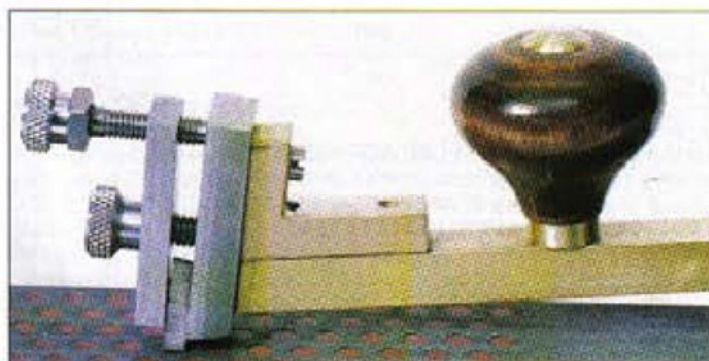
2. The tip being sharpened must be securely clamped during the operation
