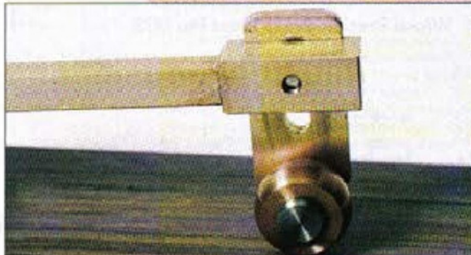
3. The guide wheel is barrel shaped to allow the device to be rotated in order to sharpen a radiused tip
