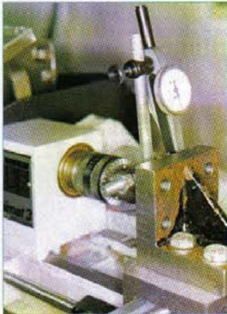
11. Setting a small angle plate at right angles to the lathe axis
