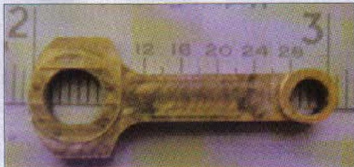
2. Miniature aero-engine conrod drawn & programmed using Dolphin CAD/CAM (machining time 11 mins)
