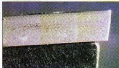
6. The edge shape on a newly-acquired tip
