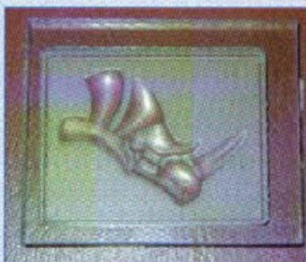
7. Rhino head cut in 6mm polycarbonate. Modelled using Rhino CAD and programmed using MillWizard from Delcam.
