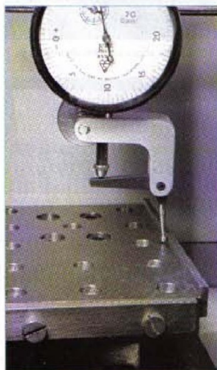
2. The dial indicator with attachments, used for lining up a milling table
