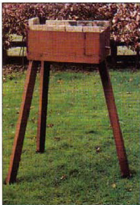
4. A need to modify some big hinges led to the construction of this simple forge hearth. All materials were left-overs from other jobs. The MMA is perfect for making such things out of doors, even working in more than a stiff breeze.
