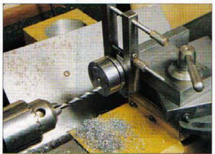
15. With the drill pad turned through 90 deg. the hole in the base can be similarly drilled.
