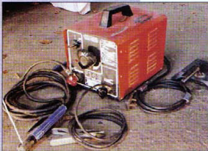
2. The faithful old MMA welding set. The only thing you adjust is the welding current. Since purchase, the set has been modified by fitting a small fan, effectively making it a 'turbo' model. The modification has allowed continuous use when using thick welding rods or 'sticks'.
