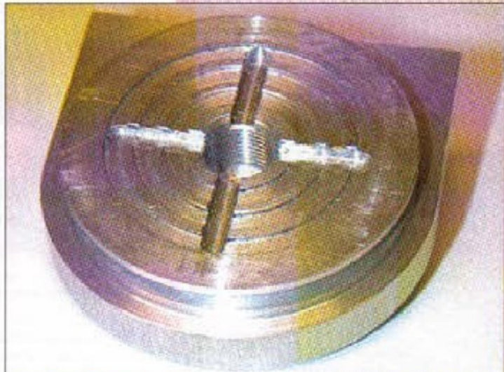
3. Grooves in the base transfer the fluid to the central outlet tube assembly.
