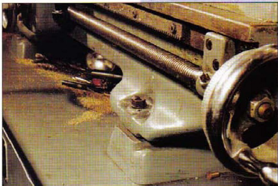
5. You can go on holiday with a much easier mind, secure in the knowledge that all your machine tools are welded to the floor! A potential thief would have to use an angle grinder or other power tool to remove the welds, and would probably not risk the attention drawn by the noise of that operation. (Remember of course, before securing your lathe by welding, that the holding-down nuts should not be more than finger tight, to avoid distortion of the lathe bed and that the machine should be covered to protect it when welding).
