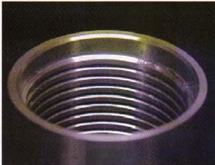
2. The fluid transfer passage was formed by screwcutting.
