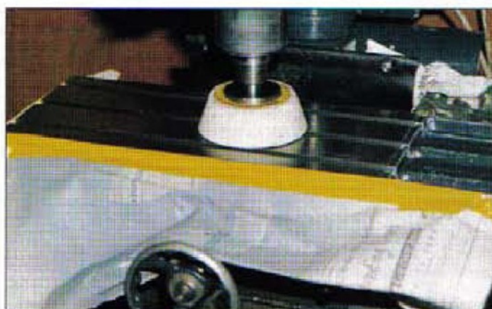
16. Surface grinding restores the machine bed to acceptable flatness.
