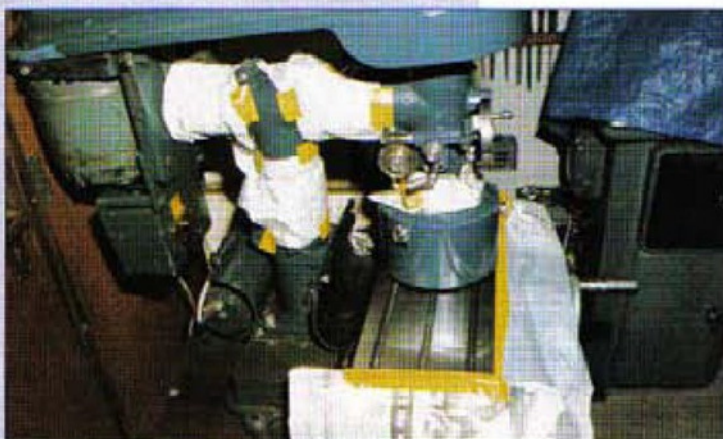
15. Slight over-kill perhaps, but protection of machine ways from grinding dust is always a wise precaution.
