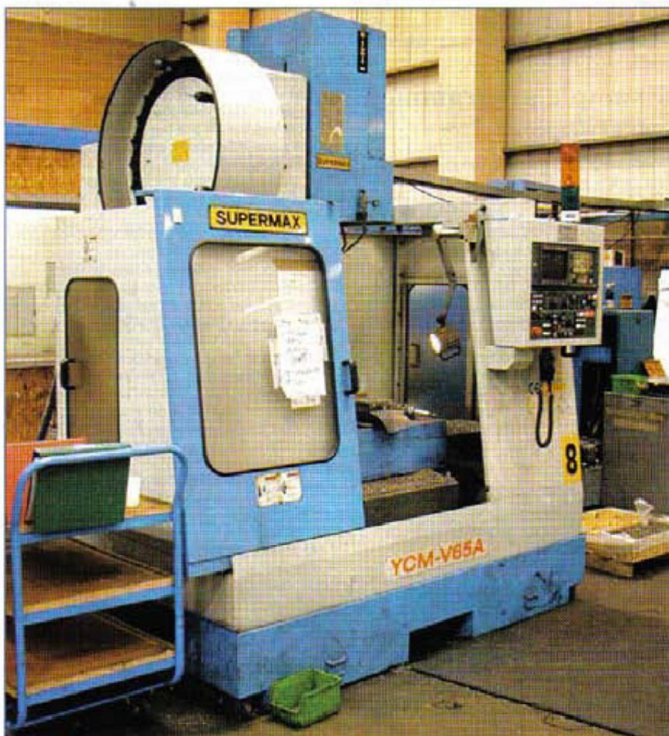
1. This 'Supermax' YCM-V65A Vertical Spindle CNC machine is one of a number used by Winson Model Technology to produce components for their kit-built small locomotives and traction engines.
