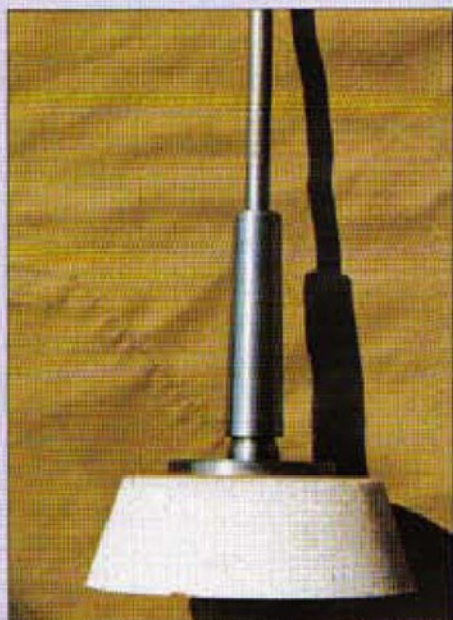
3. The assembled components. The draw bar passes through the Morse taper arbor.
