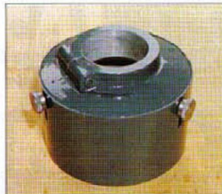
4. The completed wheel guard assembly.
