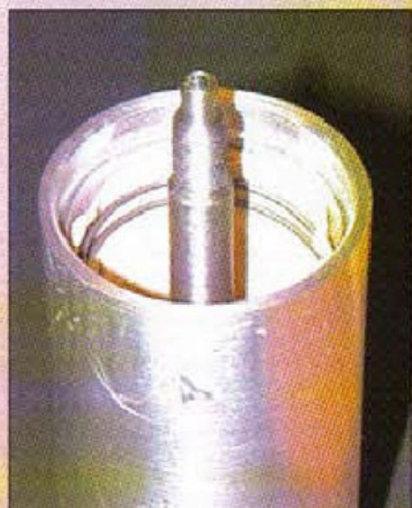
4. An internal spring holds the filter paper against the upper wall of the housing.
