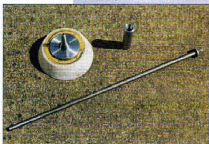
2. The new arbor accommodates Quorn grinding wheel arbors which are secured by the new draw bar.
