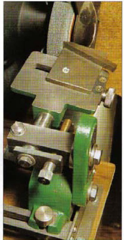
8. Shaping the end of the tool shown in Photo. 7. An adjustable tool rest such as this will give much better results than unaided free hand grinding.
