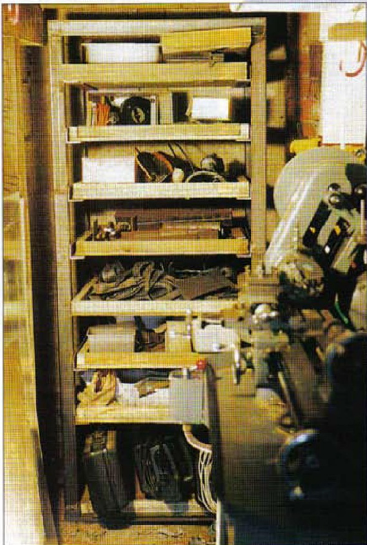
5. Shelves like this can be assembled in situ when access is difficult. The availability of 50mm x 50mm L-section steel makes it easy to provide sliding shelves, each of which will carry all the scrap metal that you can crowd onto it. You can customise shelf heights to allow optimum storage of your various hedge trimmers, alligator saws and the like.
