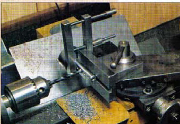
14. If you do not yet have a drilling machine all is not lost. With a drill pad on the top slide, the four holes in the column are drilled. The top slide is set at an angle to miss the tailstock, feed being applied by the leadscrew.
