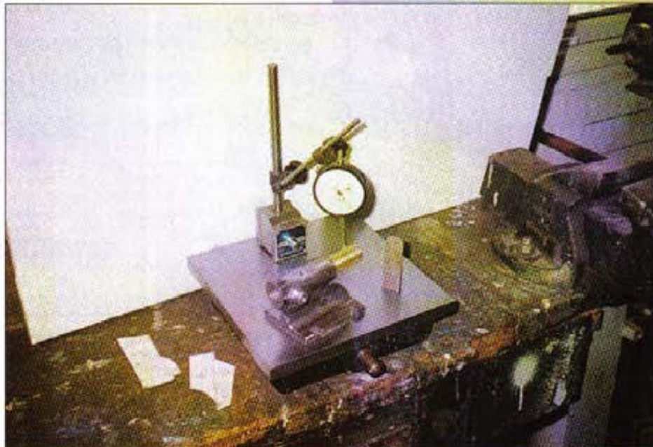
2. Finding the height of the barrel. Templates for the curved sections of the tailstock can be seen on the bench.
