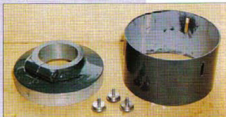
5. Wheelguard components. The slotted holes permit adjustment for variation in wheel depth.
