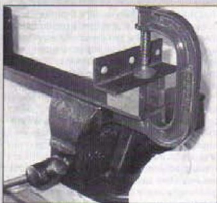
5. The anvil support plates were carefully clamped in position before welding.
