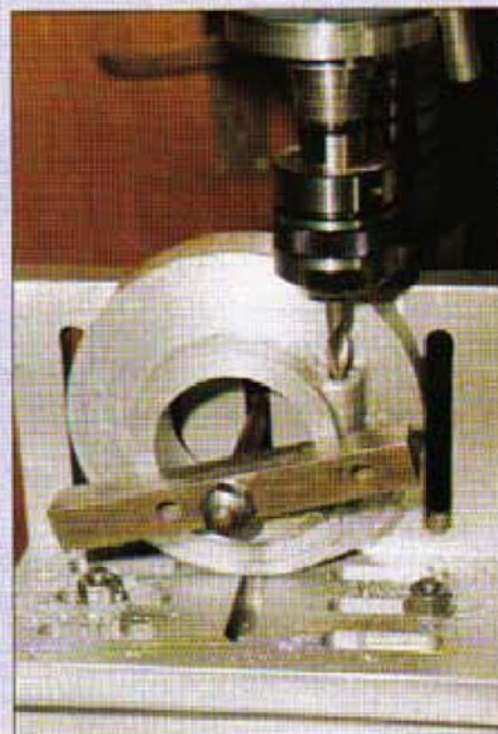
11. The new triangular key arrangement rapidly proved its worth when forming the tapped hole for the clamping screw.
