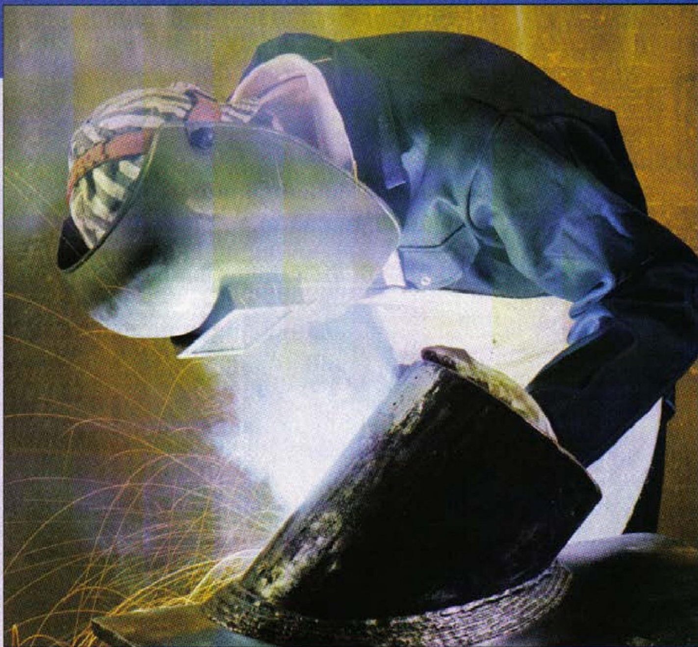
1. With just a little practice, quite substantial jobs can be tackled, but not with a bottom-of-the-range welding set! This photo, kindly supplied by TWI Ltd shows the potential of MMA welding in the construction of substantial fabrications.
