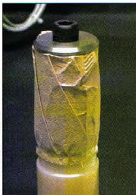
8. The filter paper is shaped over a former.
