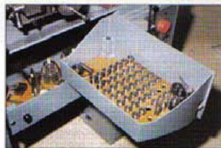
3. The substantial cabinet stand of the Schaublin incorporates conveniently accessible storage for the many accessories and attachments
