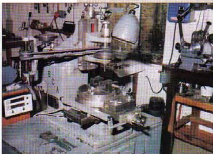
6. The BCA milling machine, complete with Ortec digital read-out equipment has departed since our visit, to be replaced by the Wabeco CNC unit described in the next article. The BCA was acquired in a very run-down condition and restored in the workshop.
