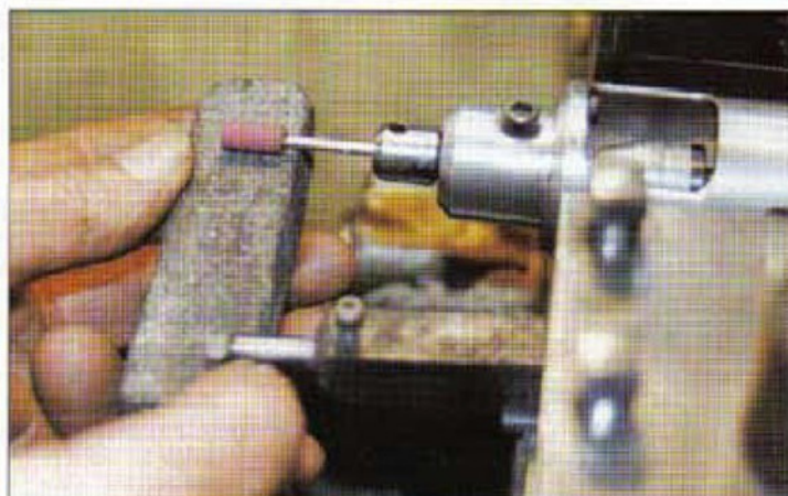
4. Dressing the mounted point with a carborundum stick
