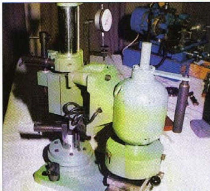
4. A swing head surface grinder, based on a design described by Alan Jeeves in these pages some years ago was entered by Peter Newby of Tyneside SME.
