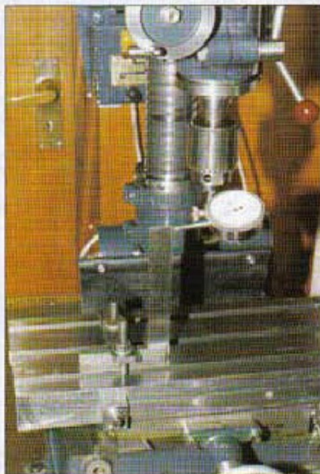
15. Alignment checks on the modified machine revealed that not all was well with the table. David Machin reveals how he overcame this in our next issue
