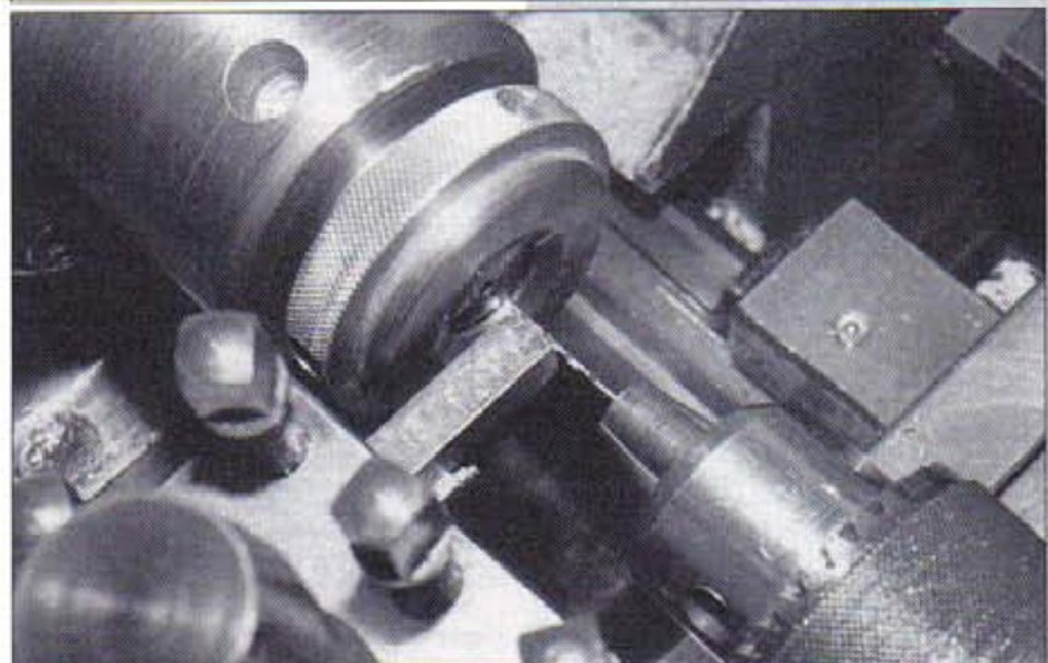
1. Providing side support for the drill by means of a bar held in the lathe toolpost.
