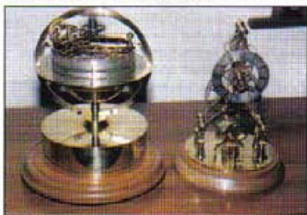
8. Two skeleton clocks built by Dick to his own designs. On the left is a spherical clock of unique design which won a Gold Medal and The Claude B Reeve Memorial Trophy at the Model Engineer Exhibition in January 1984. The time anywhere in the world can be deduced from its scales. The Inverted Y Frame clock on the right was built 20 years ago.
