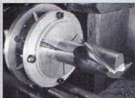
2. The super collet fixture set up in the lathe for a milling operation. The cutter with a 1.25in. shank is clamped in the aluminium collet
