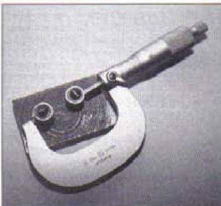
5. Setting centre to centre distance with a pair of toolmaker's buttons.
