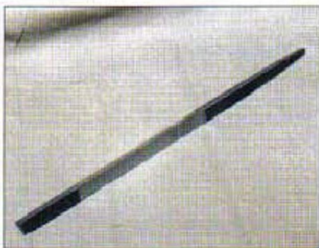
3. The part completed key, still with the tapered and centre-drilled ends
