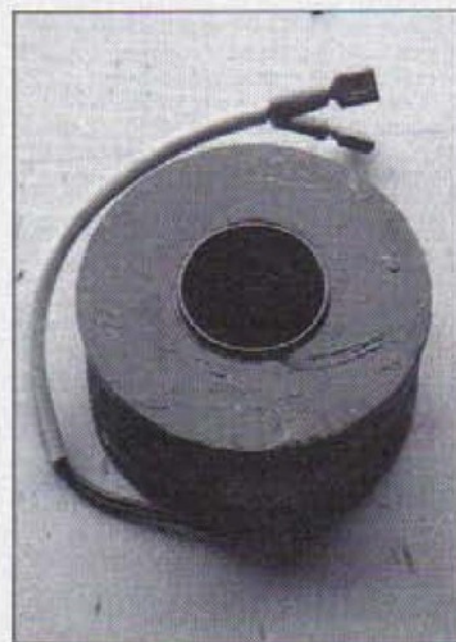
1. A simple solenoid. The brass sleeve mentioned in the first article is clearly visible.
