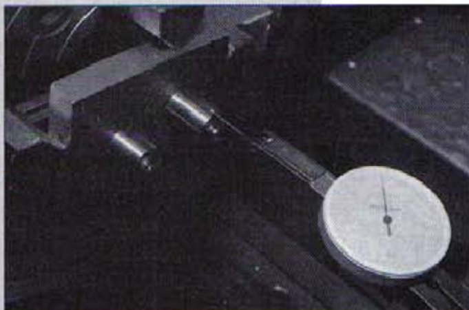
7. Centring by means of a toolmaker's button.
