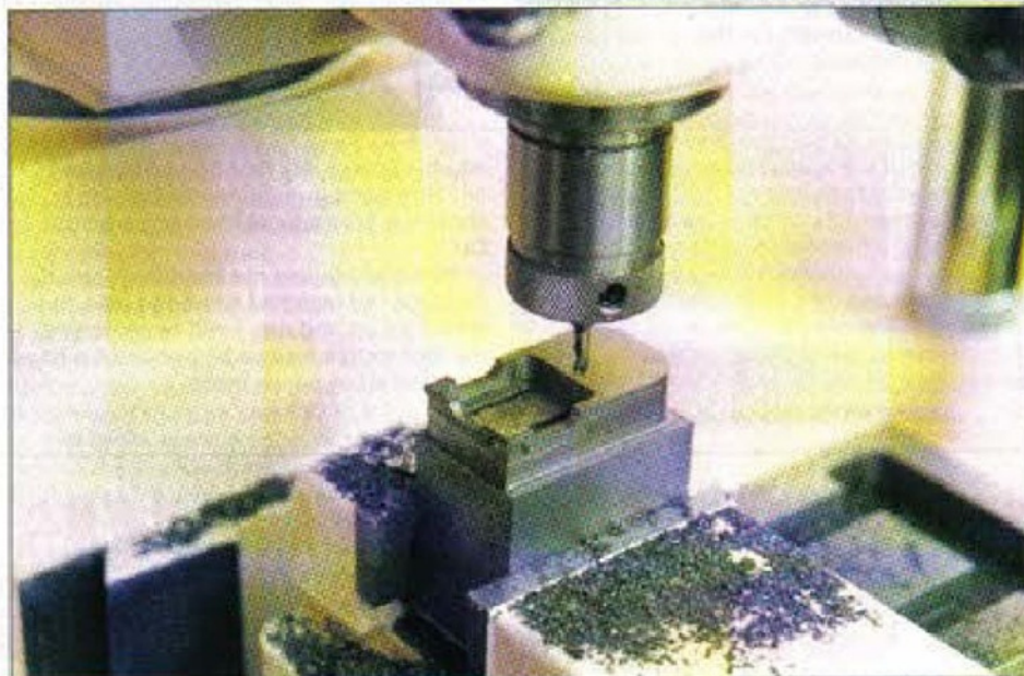
5. The base of the 'Fobco' Star being formed on one of the cast iron blocks
