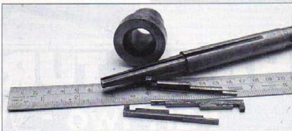
2. The components, showing that the blades are housed in shallow tee slots
