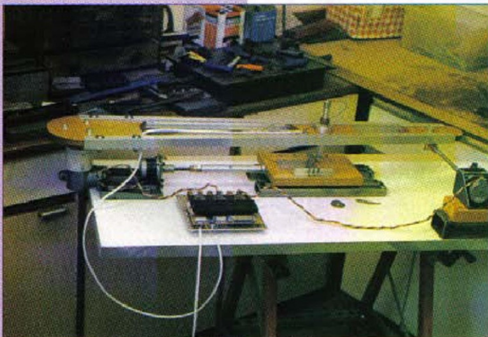
3. Compensating digitising board set to 5x scale of the Compucutter
