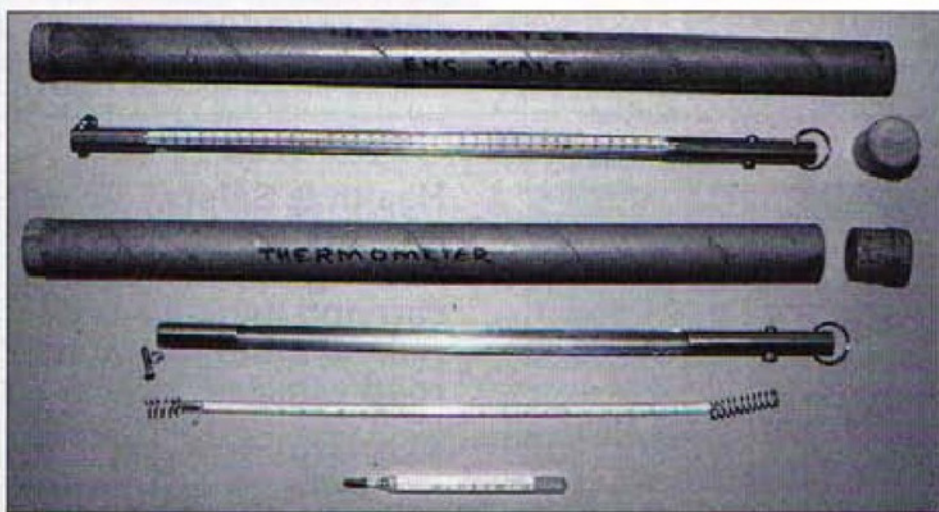
2. Physical protection for mercury-in-glass thermometers
