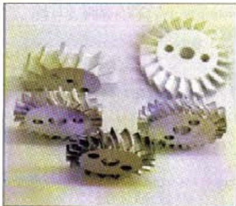
5. Test rotors showing a variety of blades shapes machined in polyester resin (rear), aluminium alloy (centre) and stainless steel
