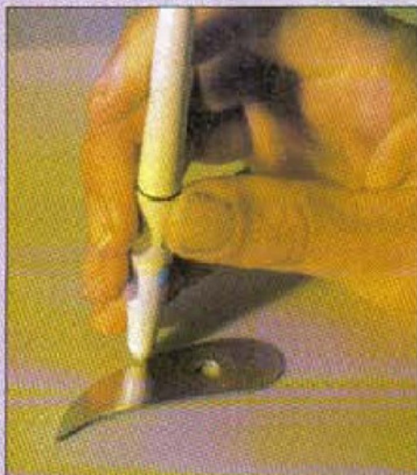
9. Whilst tracing around a profile, the co-ordinates of the data points are being stored in a file in the computer.
