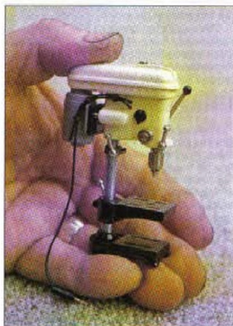
2. The \frac{1}{12} th scale model of a FOBCO 'Star' bench drill which was used as the test vehicle
