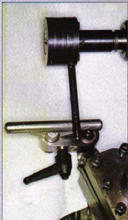
8. Another use for the tool rest - supporting the torque arm of the tailstock die holder when threading
