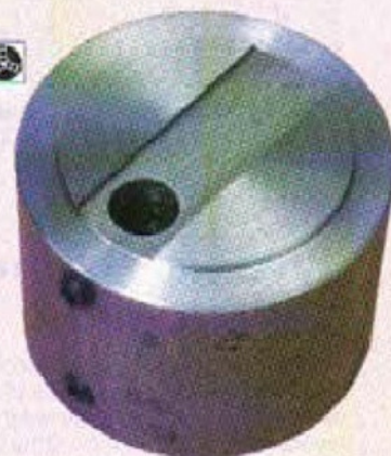
6. The fixture to be used for machining the crankpin
