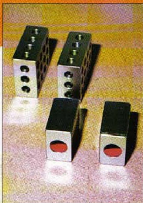
1. The four blocks provide a useful combination of heights on to which to set a workpiece
