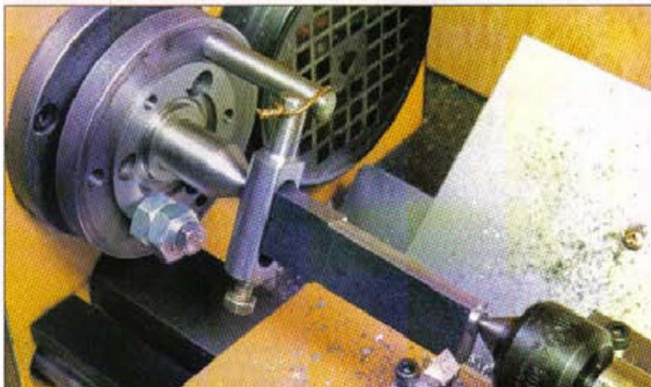
3. Turning a short portion of the end journals to use as a guide when sawing away the excess material to bring it to the form shown in Photo. 4
