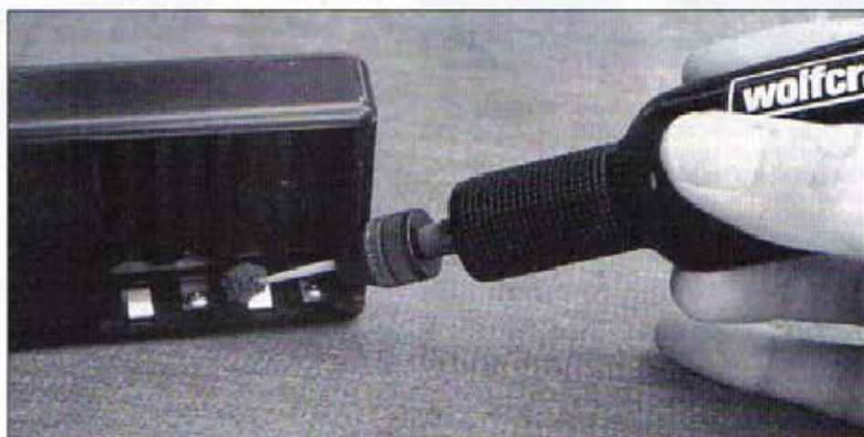
5. The 'tooth pick mandrel' is more suited to finer work
