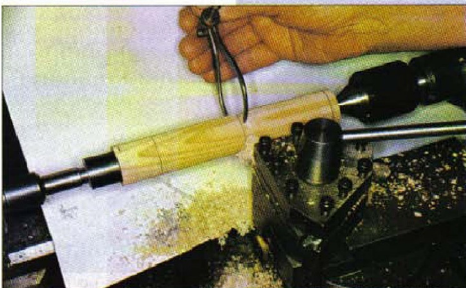
5. Sizing the sighting groove which will determine the maximum finished diameter
