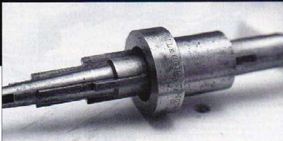
1. Hugh Smith's mandrel clearly shows the legend C. W. LeCount, Norwich stamped on the collar
