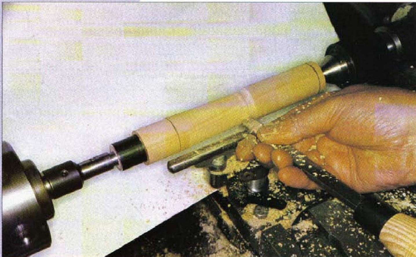
6. Shaping using the half round tool. The white background allows the generated profile to be seen clearly
