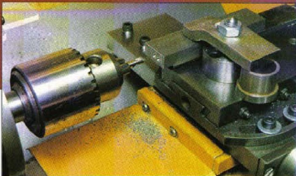
1. Drilling each end with two centres for use as in Photos 2 and 5
