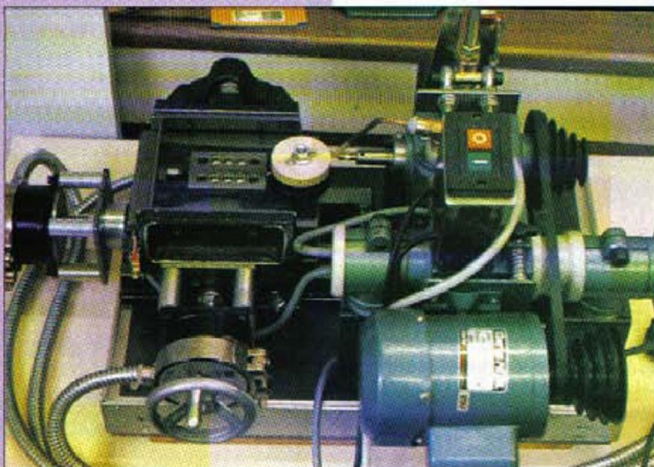
2. A Compucutter machine set up to mill a turbine rotor
