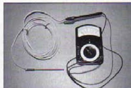
4. Chromel/Alumel thermocouple, continuing 5m leads and analogue multimeter (used on 0-50 microamp range)
