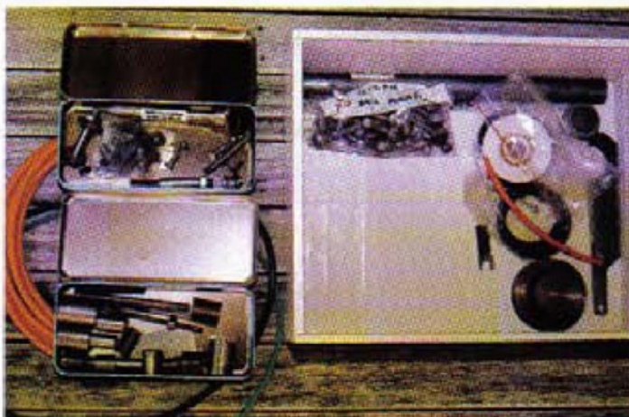
22. The special tooling used in the manufacture of the Quorn has been retained and is kept in Box 4. The first spindle made can be seen in one of the tins and the displaced ball handles are in one of the plastic bags
