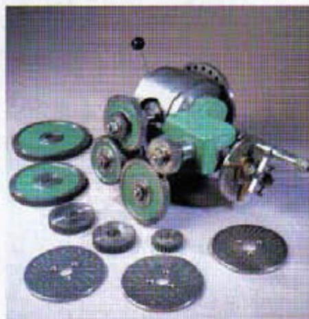
We have persuaded Chief Judge Ivan Law to exhibit his Universal Spiralling and Differential Indexing Dividing Head in the Loan Section
