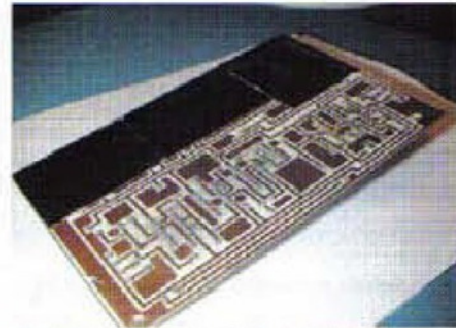
20. The track side of the Combined PCB showing that the tracks which are at mains potential have been protected with insulating tape
