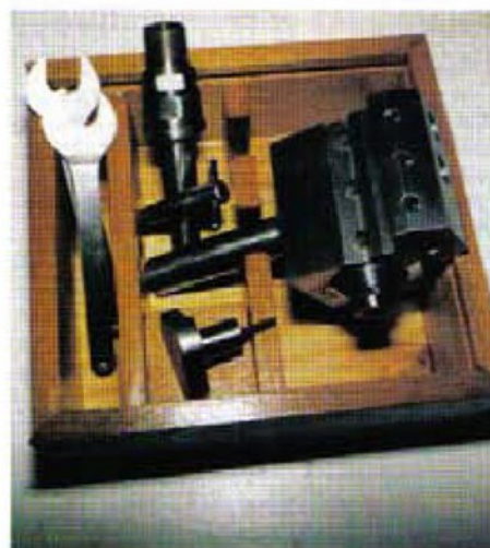
This boring head, entered in Class A5 is the work of Malcolm Leafe of Dewsbury, West Yorkshire
