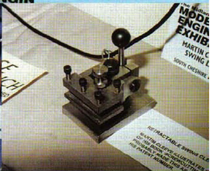
8. M. W. Smith entered this version of the Martin Cleeve swing clear toolholder for display on the South Cheshire MES stand. It is suggested that it was made by the designer as it is stamped with his Patent number
