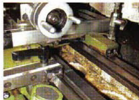
12. A linear scale fitted to a lathe
