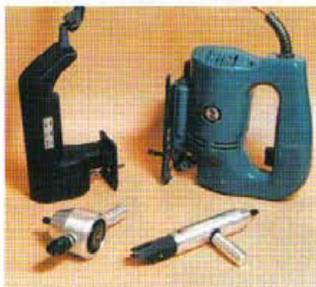
9. Power tools for cutting sheet metal.
