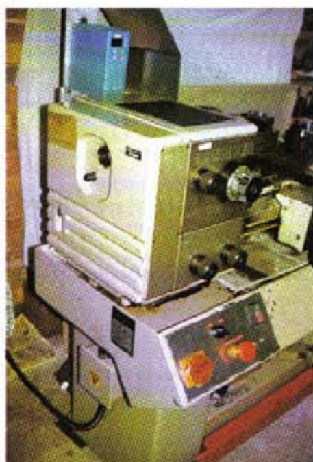
4. The panel has been incorporated into the lathe structure, bringing all controls conveniently to hand
