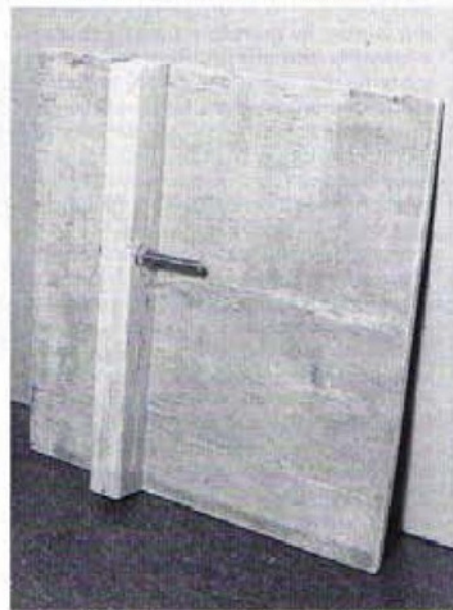
2. The bar on the back of the work table that permits it to be held in the bench vice.
