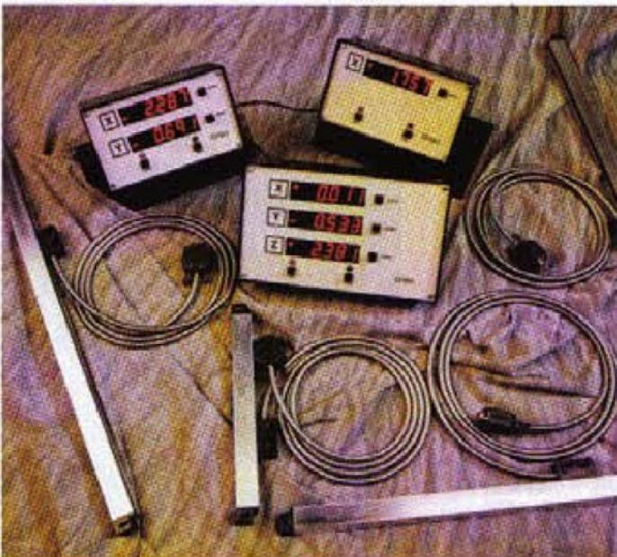
9. The Ortec system uses a linear encoder
