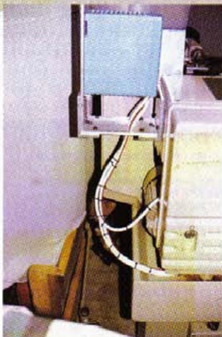
2. The unit is secured to a bracket mounted on the rear of the headstock. If preferred it can be wall mounted
