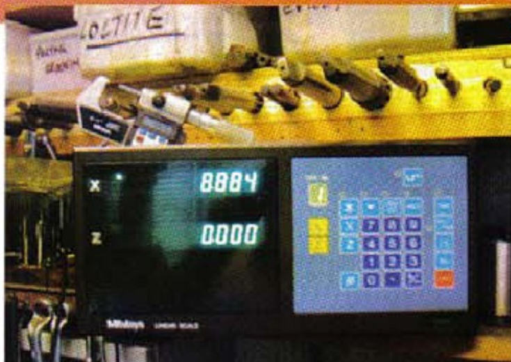
1. The 2 axis read-out of the system fitted to the author's lathe
