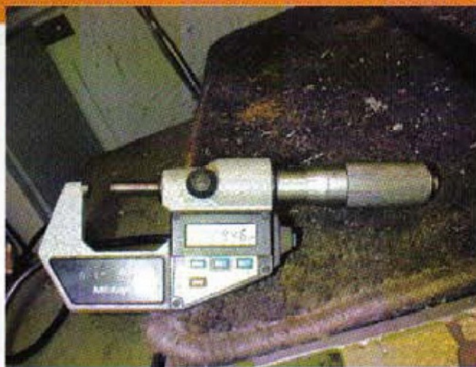
2. A digital micrometer of the type which can be connected to the system
