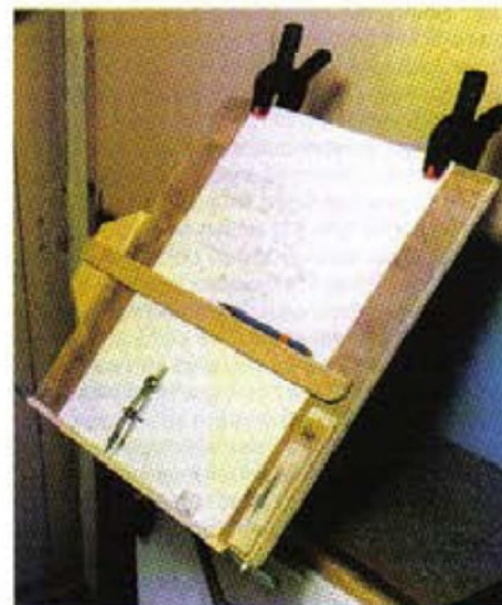
6. Using the bolt seen in Photo. 2 , the table can be mounted at an angle providing a drawing board or a stand for one's plans.
