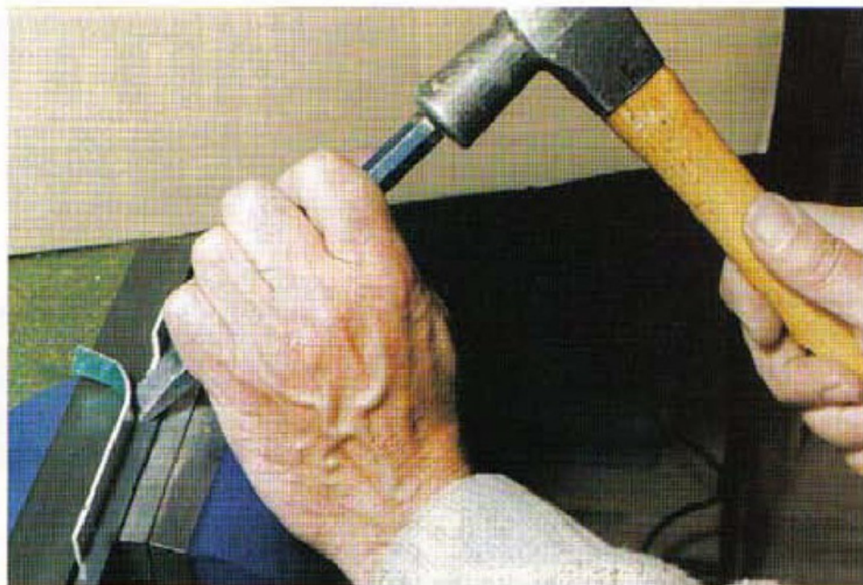
8. A cold chisel makes easy work of cutting out a notch on the side of a piece of metal. The sides of the notch having been cut using a saw.
