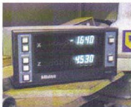
4. The X and Y axis read-out on the author's milling machine
