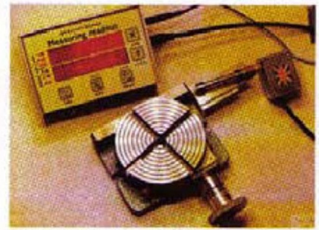
8. The B. W. system can also be adapted for use on a rotary table
