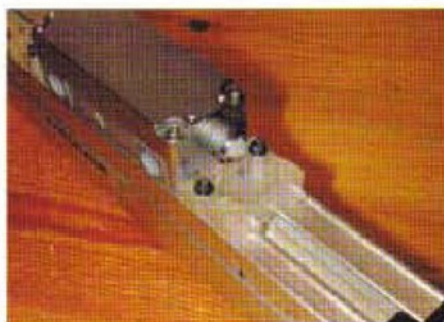
13. Transit blocks which protect the components until they are secured in position
