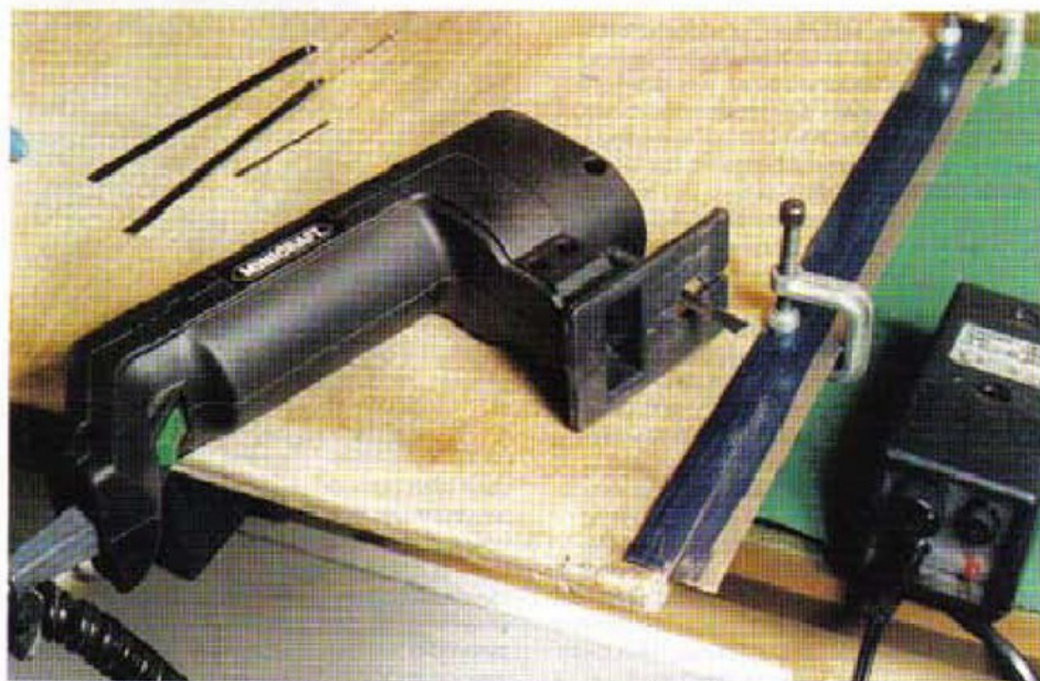
11. The small jig saw is more at home with thinner material, this time 0.5mm thick steel.
