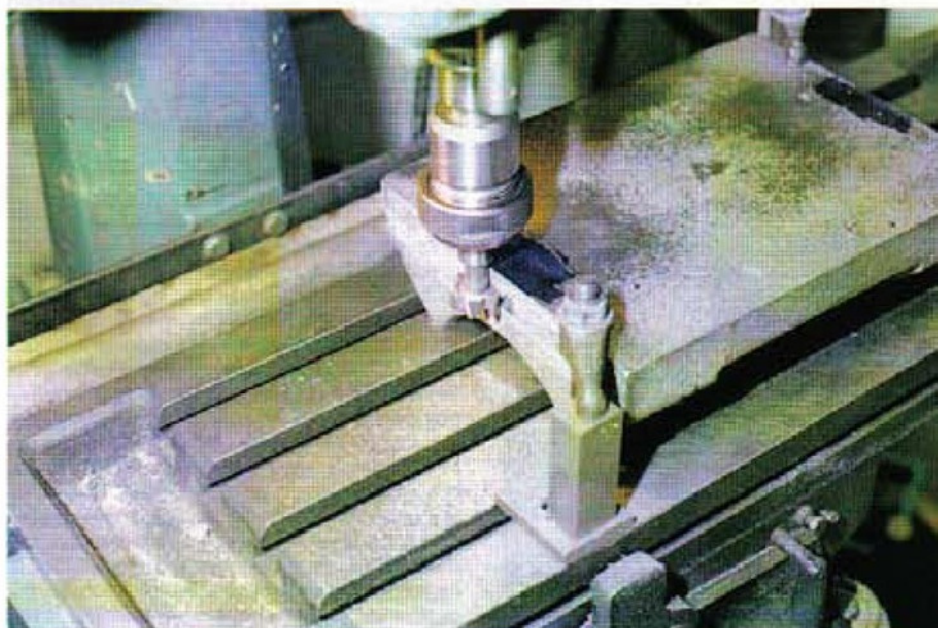
6. Milling the holding-down recess
