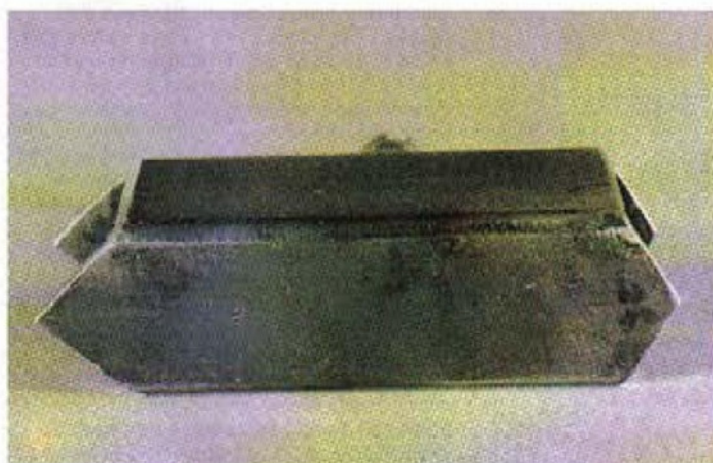
3. Mk. 1 jig, underside. Note the different angles at the two ends, one for drills and the other for countersinks
