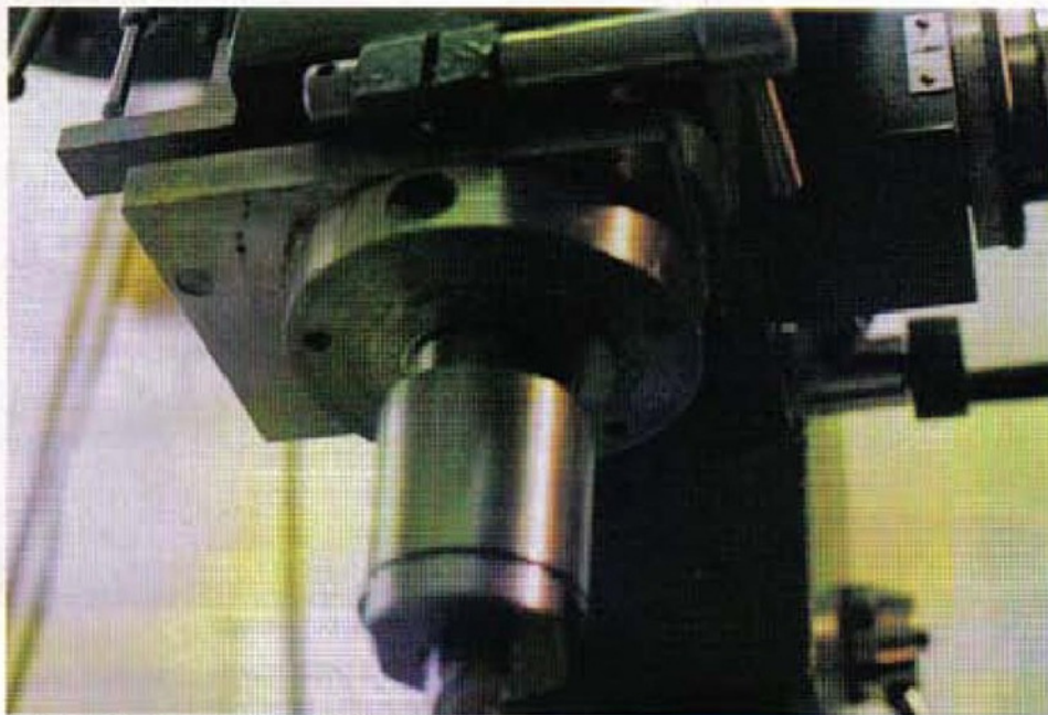
The spindle flange for mounting a boring head, the register having been machined in situ
