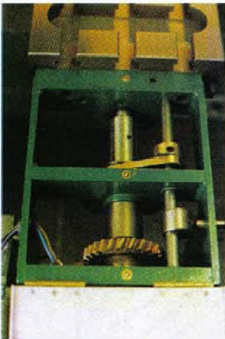
The centre wall forms a bearing support for the gear shaft. Note the three spring loaded oiling points which facilitate spindle lubrication
