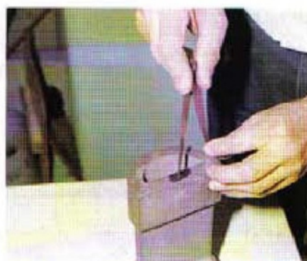
3. Setting out centres on the base casting
