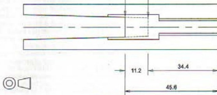
FIG.1 Arbor ejector requirements tailstock barrel
