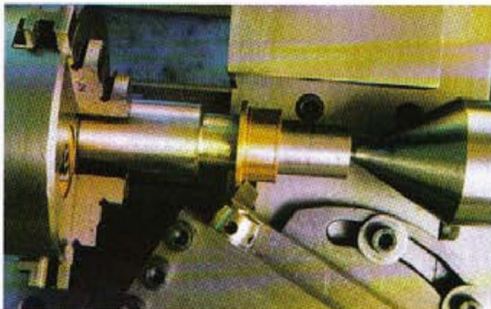
Turning the Spindle Bush Liner (Item 8) to produce the gap required to obtain a satisfactory adhesive bond. Note the lands which maintain concentricity of location
