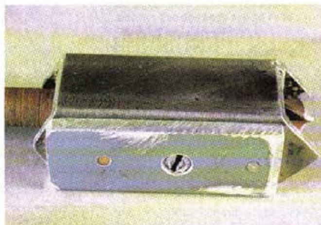
4. Mk. 2 jig showing the recessed clamp screw and guide pins which allow the jig to be turned over. This removes the need to re-set the drill position in order to grind the second facet. The drill shown is a near-scrap one which was successfully resharpener
