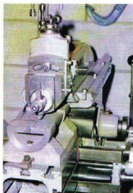
10. Cleaning up the undersurface of the base casting
