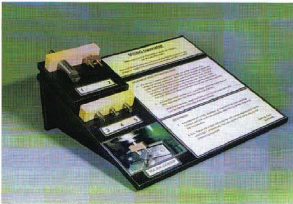
2. A simple 'lectern' style display board: Five individual pieces of setting equipment are mounted in blocks fitted to a sloping board for easy viewing. The descriptive notes are augmented with a photograph showing their use.
