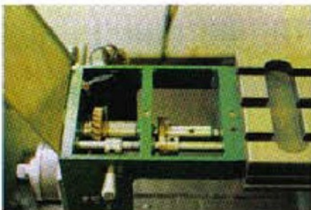
With the cover open, the dog clutch mechanism is easily accessible. To the left is the housing for the wire wound variable resistor which provides control of the feed rate
