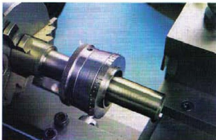
Graduating the Micrometer Index collar while mounted on a tapered mandrel
