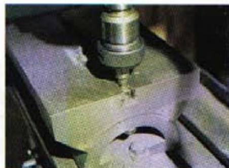
16. The danger moment for a tee slot cutter
