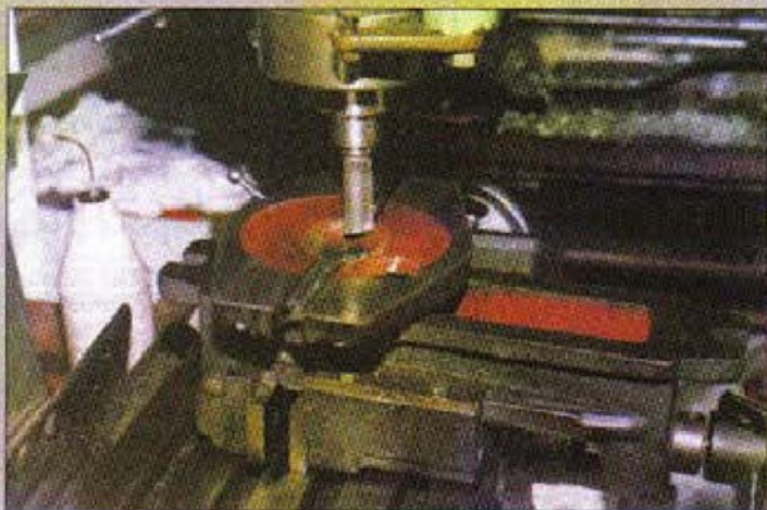
3. Cutting the \frac{1}{8} in. deep slot in the base of the vice
