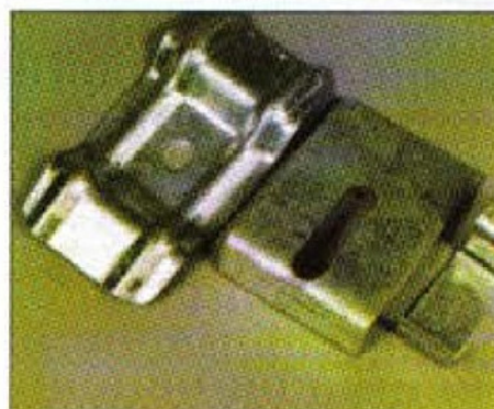
2. Hot dip galvanising is more appropriate for items for external use
