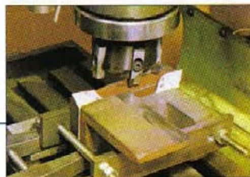
9. Surface on the hob spindle housing being machined to take the bearing bracket (Item 3)
