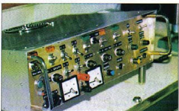
23. Final view showing how important it is to attach clear labels to the front panel
