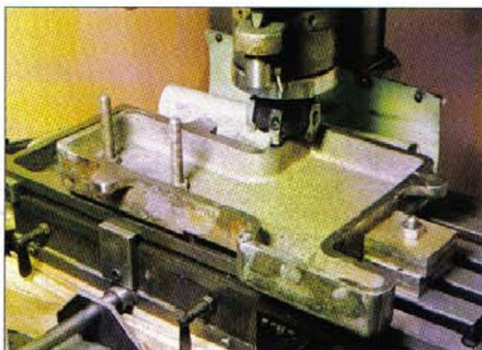
4. Machining the underside of the bedplate. The bedplate had to be moved three times to complete this operation.
