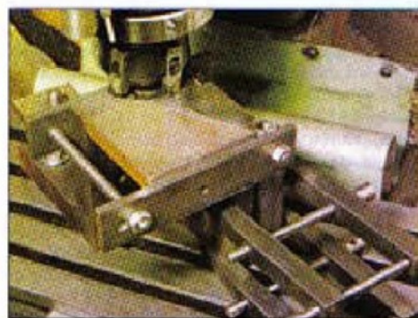
6 and 7. Machining the vertical slide bracket (Item 5)
