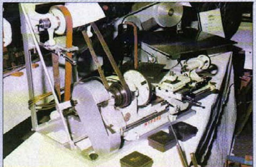
Barry Keal of Lincoln & District M. E. S. exhibited a neatly restored early Myford lathe, complete with a flat belt drive assembly.
