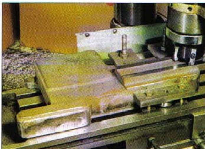
3. Preparing a surface on the top of the bedplate so that it can be turned over and mounted on the machine table for machining the underside.
