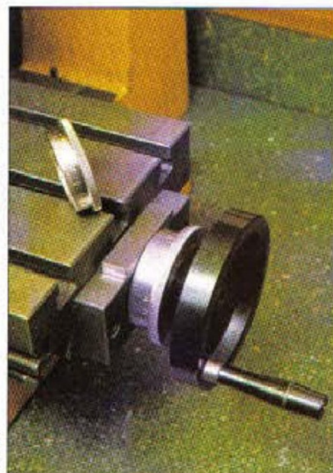
6. The new dial fitted to the milling machine. The original dial is standing on the machine table for comparison
