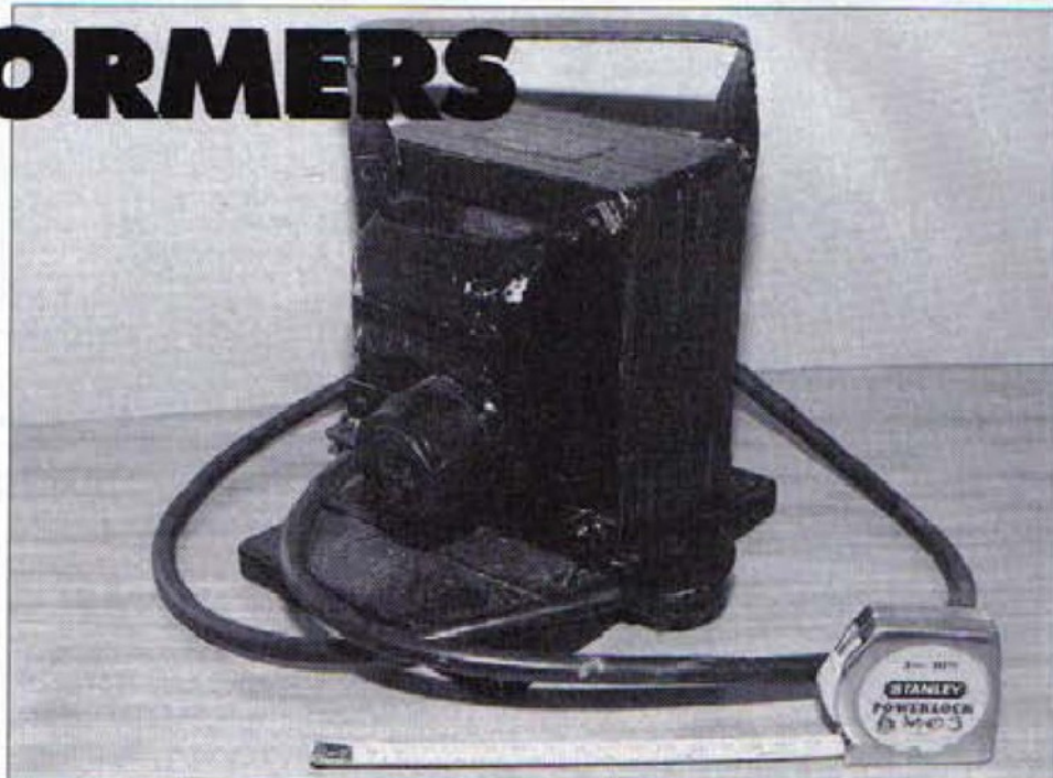
1: Typical 240/110 volt small power transformer with plug & lead for primary and socket for secondary connections. Coils are enclosed with metal shields and a carrying handle is provided. Note ventilating louvres in metal end shields.
