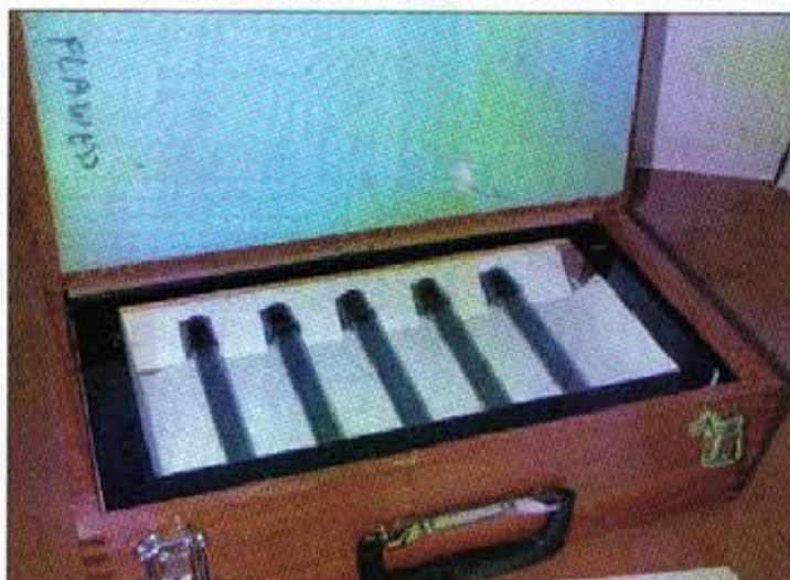
6. Plate glass and a foam lined lid complete the light box
