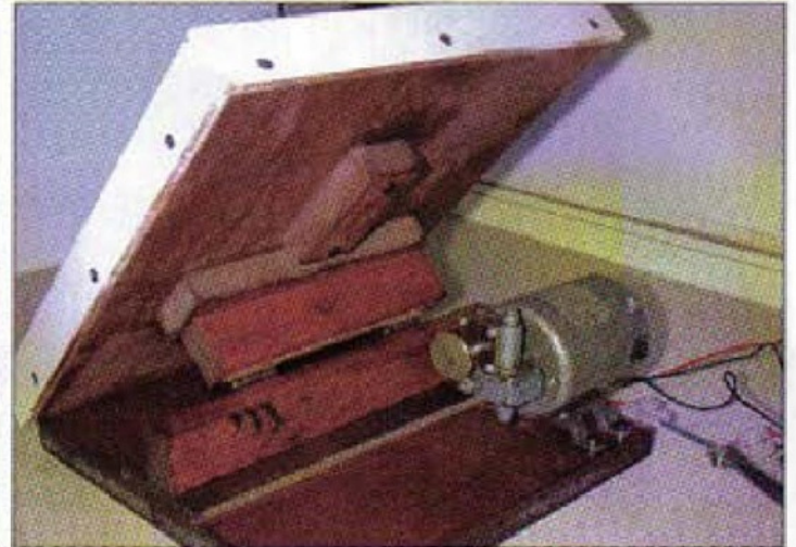
8. The 'works' of the rocking table
