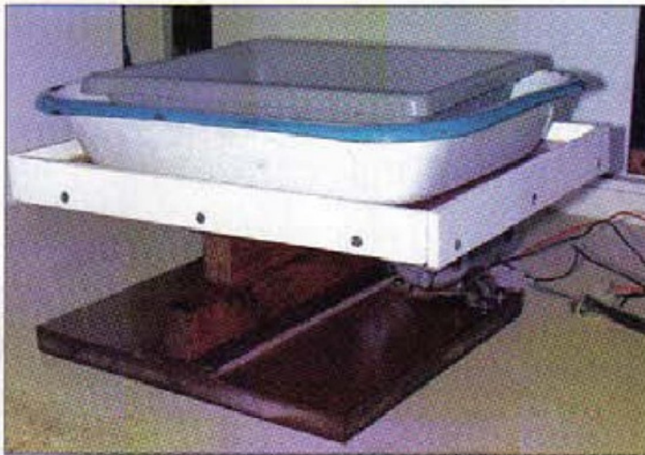
7. A simple rocking table assists the etching process
