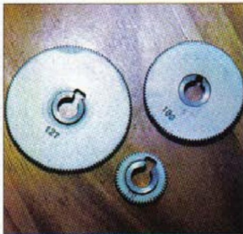
11. Sherline changewheels adapted for use on the Peatol by bushing
