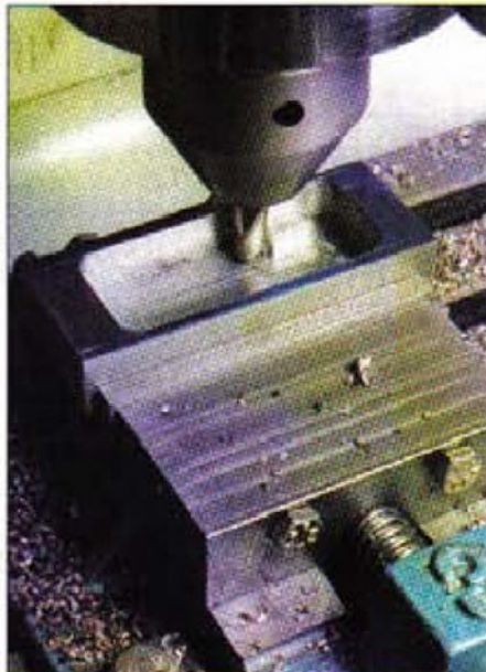
2. Milling the recess in the slide body
