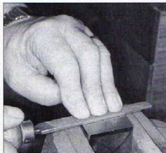
6. Finishing off one surface of the toolpost
