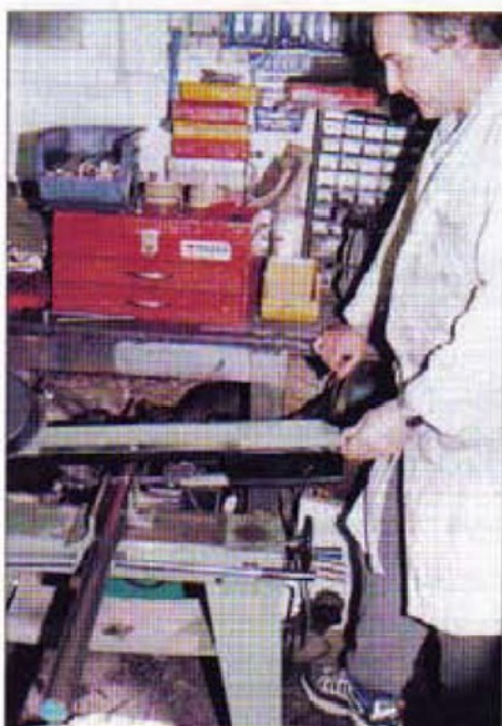
Alan sets up the bandsaw to cut one of the larger sections
