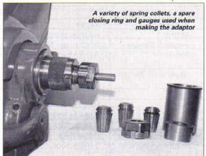
The adaptor fitted to the Myford mandrel nose
