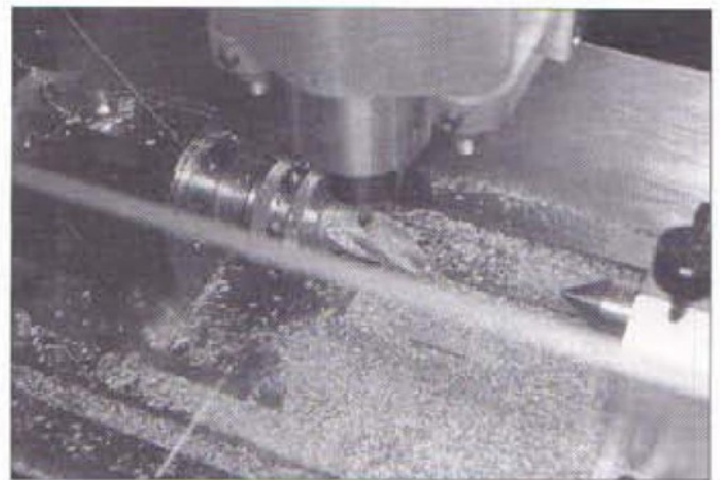
50. The previously plotted spiral being machined in brass
