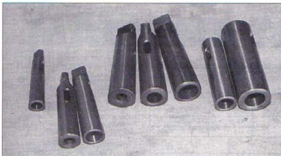
1. MT Sleeves - left to right - No. 1 to No. 2; No. 1 and No. 2 to No. 3; No. 1, No. 2 and No. 3 to No. 4; No. 2 and No. 3 to parallel
