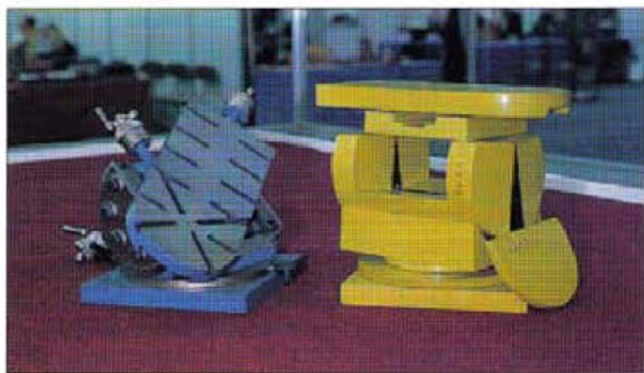
3. Another Silver went to Geoff Allen for a cast iron version of his tilting compound table. This one was shown complete with patterns. (Photo. Jon Jolliffe)
