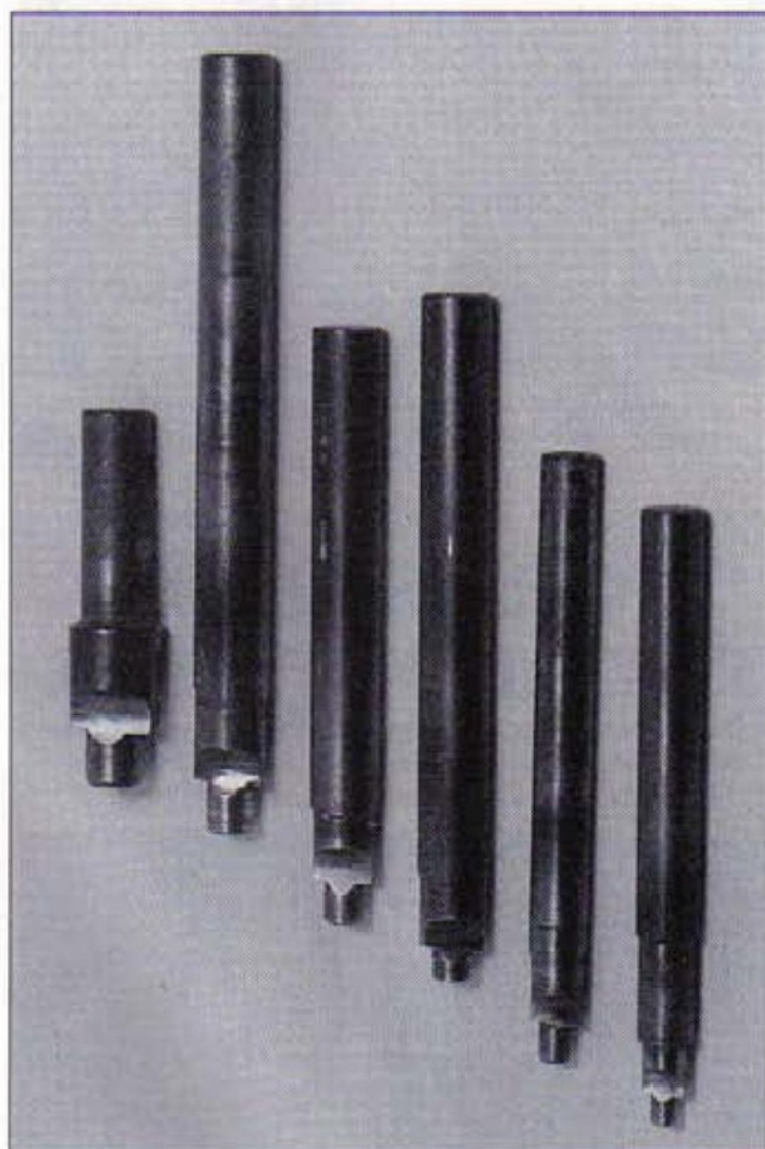
5. Counterbores to suit cap head screws from M3 to M10
