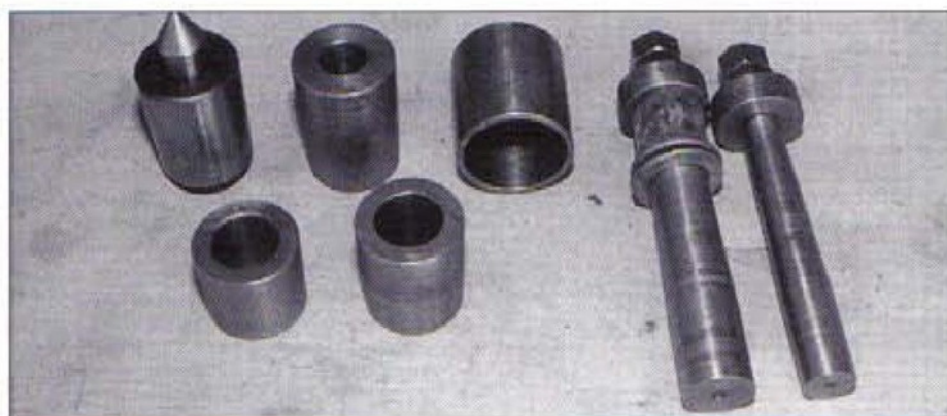
6. Left to right - 'Bought' sleeve No. 4 1/2 / No. 2MT with No. 2MT soft centre; 'Made' sleeve No. 4 1/2MT / No. 2MT; No. 4 1/2MT gauge; No. 2 and No. 3MT mandrels. Foreground 'Made' sleeves No. 4 1/2 / No. 3MT
