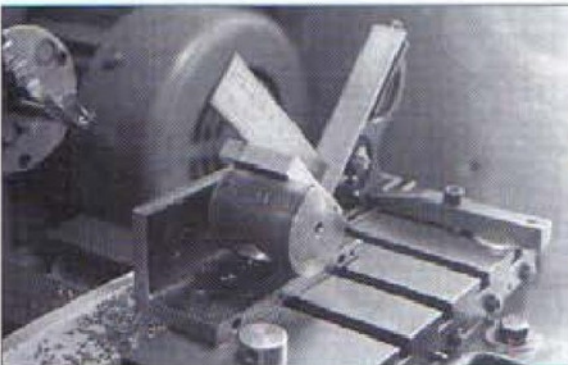
13. Method of setting the body at 45 deg. to the angle plate (operation 3.10)
