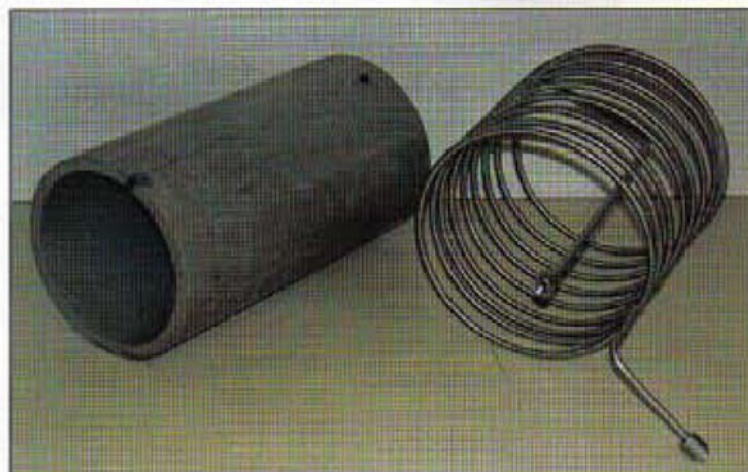
1. The Large Diameter Tube Bender and typical coil formed on it
