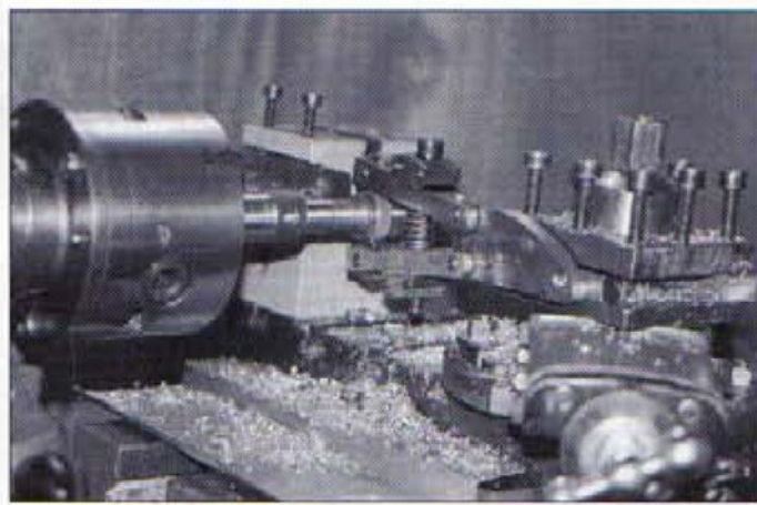
7. Straddle Knurling the clamp nut (operation 1.23)
