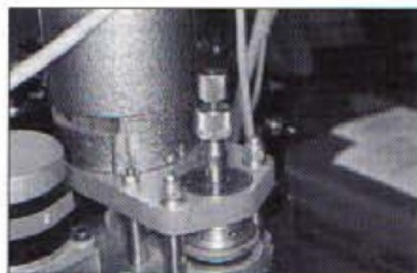
30. The spindle drive arrangement showing the collet draw bar, pull nut and cap on the spindle
