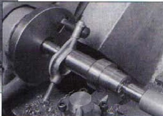
6. and 7. Machining the spindle between centres to ensure concentricity.
