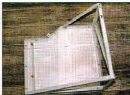
14. Table assembled with bracing angle across blade access slot
