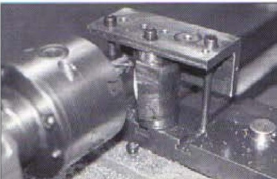
14. Milling the 45 deg. clearance flat on the body (operation 3.11). The packing piece under the body is the shell of a discarded bearing
