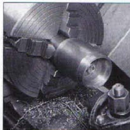
8. Boring the second end of the outer bearing whilst mounted on a stub mandrel.
