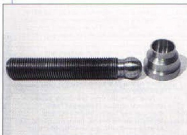
6. The ball ended clamping screw and the foot
