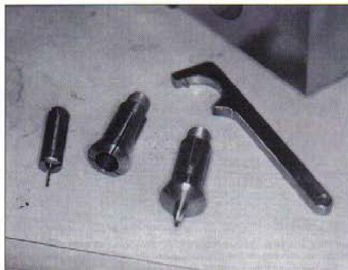
27. Collets to fit the original pattern spindle
