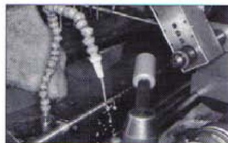
28. The tailstock drilling unit was used to make the draw bar hole in the spindle
