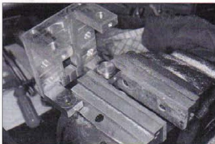
23. Using a button to mark out the radii on the arms of the partly machined Z axis support frame
