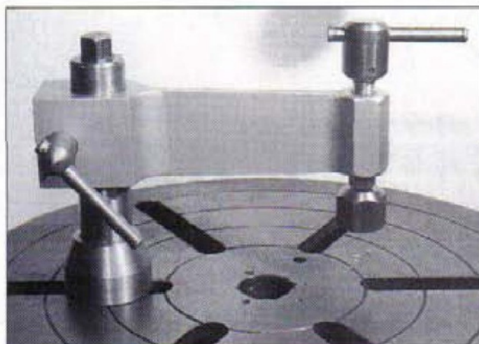
4. The earlier version of the clamp which features a fixed length beam with cotter clamping
