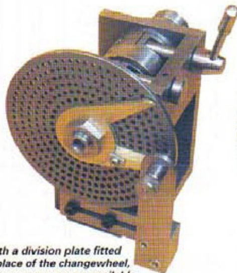
16. The worm and wheel provide the maximum flexibility
