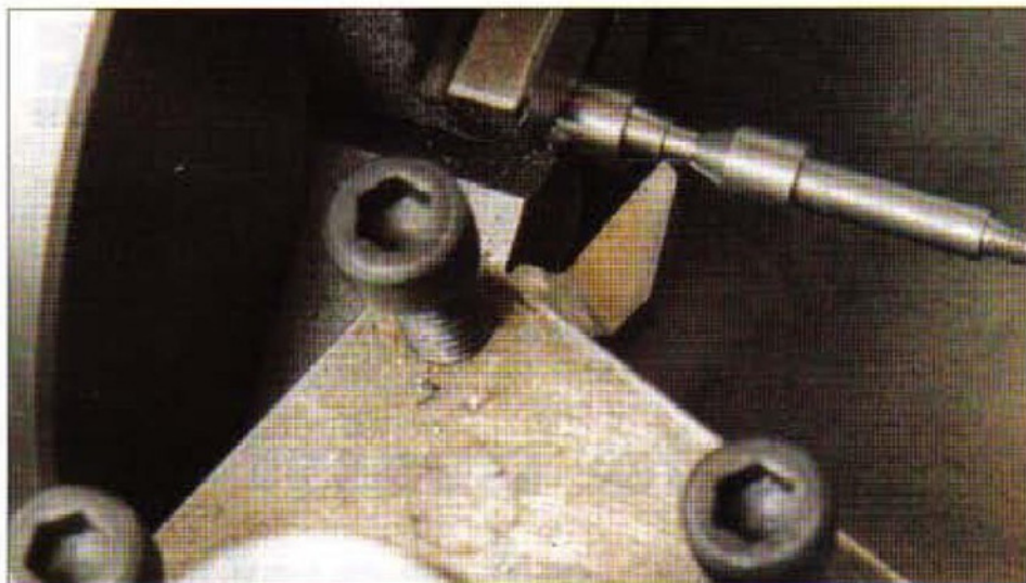
22. Machining one of the detents, all diameters being machined at the same setting to ensure concentricity
