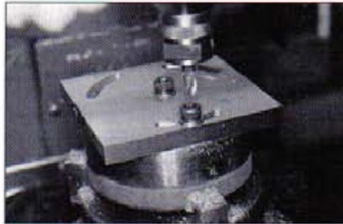
17. The slots which allow the turret to be tilted were machined on a rotary table
