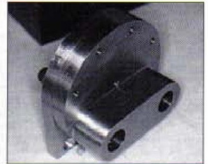
18. Removal of some of the excess material improves the appearance of the turret mounting components
