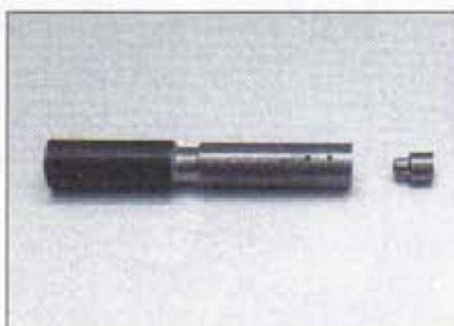
14. Test rod with vent holes and cap screw insert
