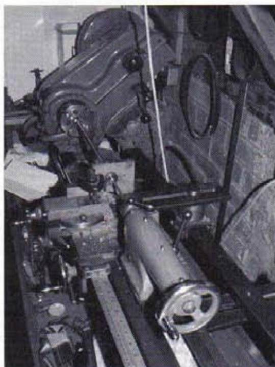
John Hughes' method of taper turning
