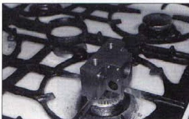
13. Heating to remove the clamps
