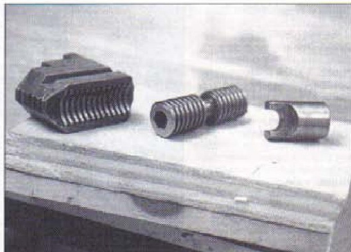
13. Finished screw, together with its jaw and thrust fork
