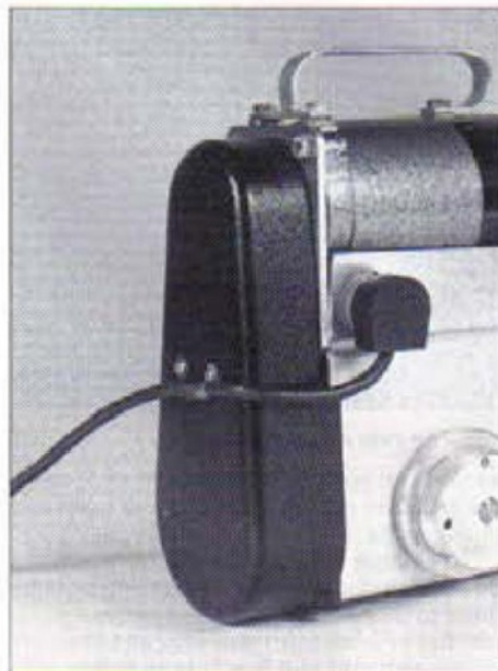
12. By careful positioning of the cable clip, the belt guard cannot be removed until the cable is unplugged. This photo shows an earlier standard, where the cable was secured with a 'P' clip fitted to one of the belt guard plug self-tappers. A cable tie may be used if preferred
