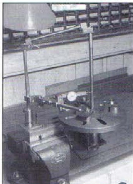
6. Using the balancing fixture (to be described in a later issue) to position the main frame end plates on the faceplate prior to preliminary boring of the large hole
