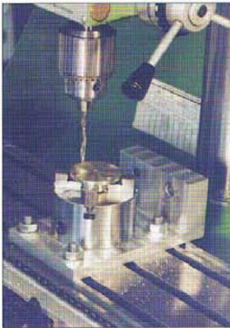
4. End drilling with the fixture
