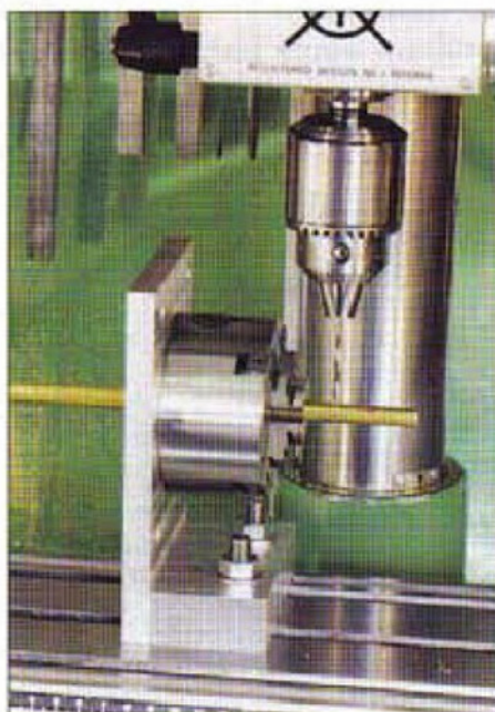
2. Cross drilling with the fixture
