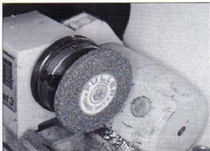
9. The grinding wheel used to grind the slots in the cutters
