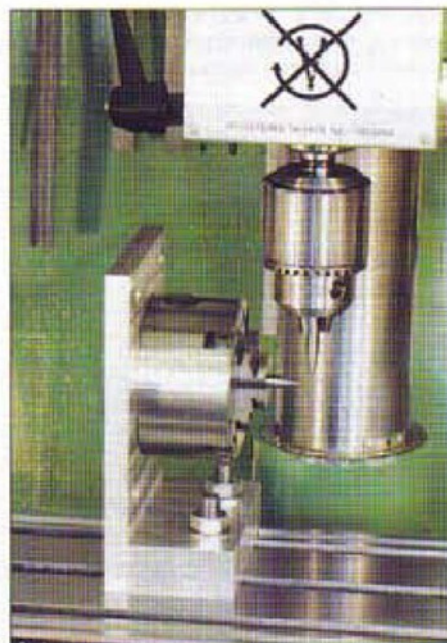
3. Alignment technique for cross drilling
