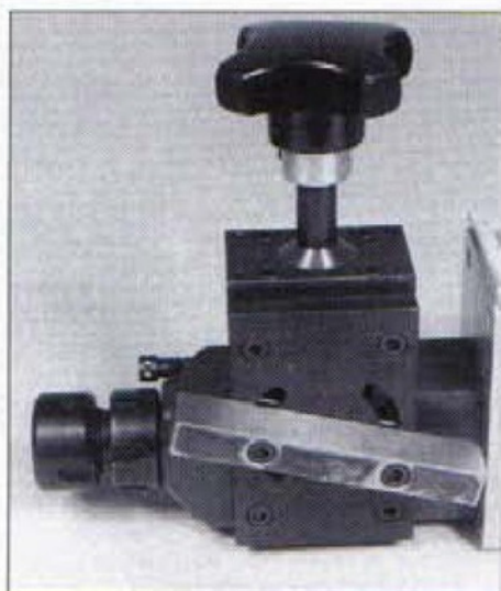
9. The swivel assembly allows the unit to be mounted at an angle, particularly useful for such operations as spiral milling
