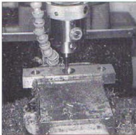
2. Machining the bearing recess in the slide bar support
