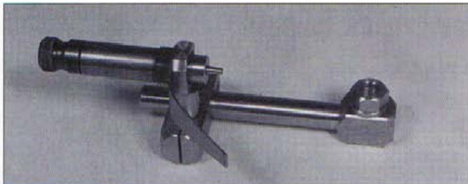
14. This detent assembly is designed to be attached to the Myford S7 headstock. The finger is adjusted to sit just over the division indications on the chuck backplate or indexing ring
