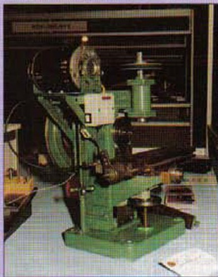
8. Somewhat bigger was the bench milling machine, also made by Tom Bartlett
