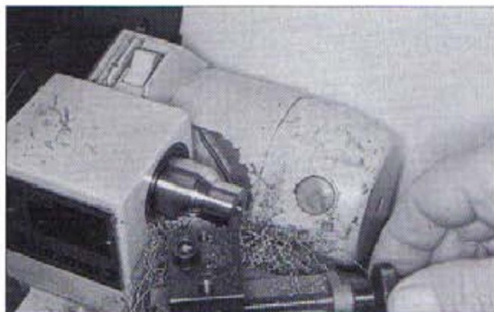
13. Turning the large chamfer on the small holder
