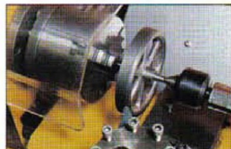
13. Finish machining all machined surfaces of the flywheel whilst mounted on a taper mandrel.
