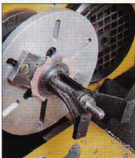
10. Again using the base plate, this time whilst machining the feet of the standard.
