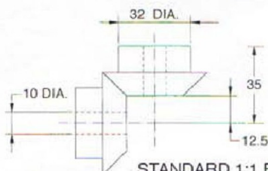
STANDARD 1:1 BEVEL GEARS 1.5 MOD. 26 TOOTH, STEEL
