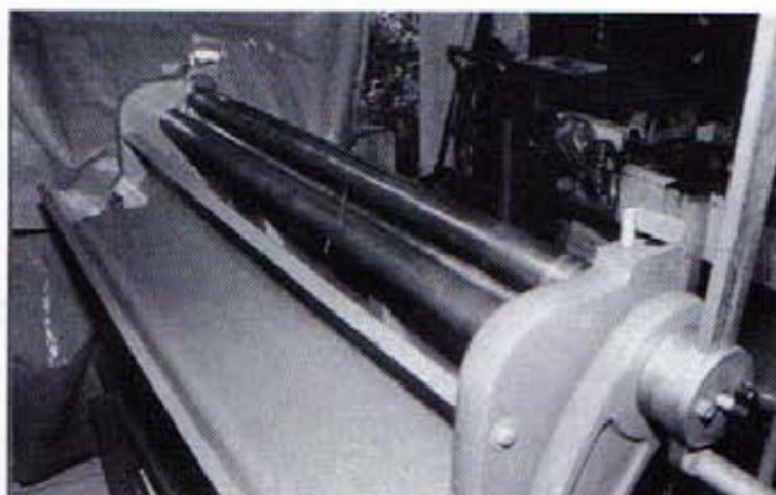
13. Deflector roll. Gearing of pinch rolls can be seen at far end
