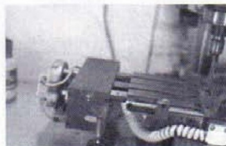
1. The box containing the microswitches acts as the fixed stop
