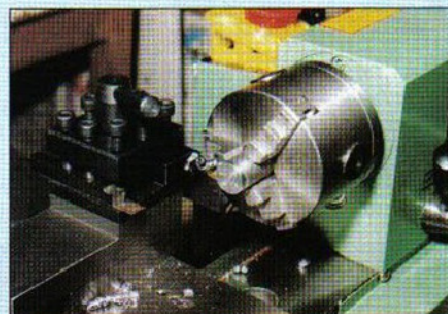
A Greenwood Tools parting tool made short work of producing some steel discs.
