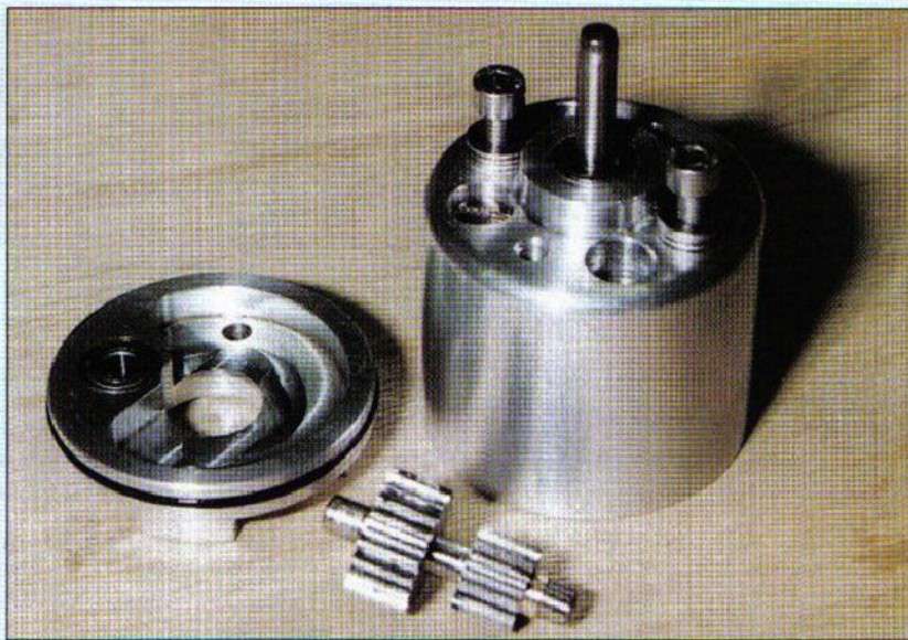
The works of this beautifully machined aircraft gearbox had become deranged, but were restored by the judicious application of a little 'Loctite'. However, the main problem proved to be how to gain access to the 'works', so well did the components fit together.
