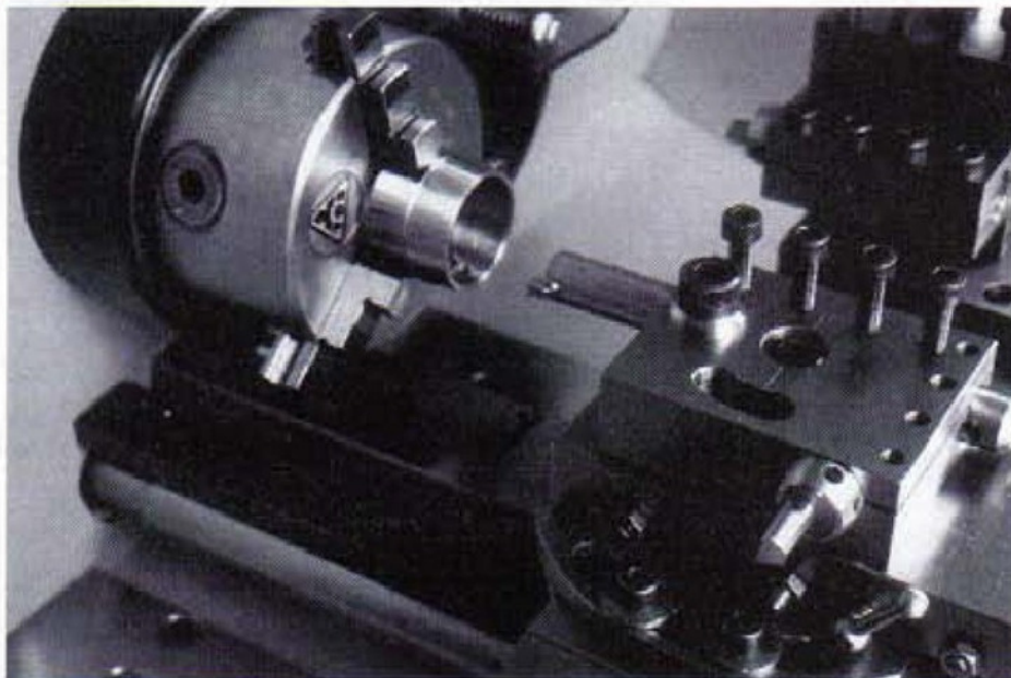
13. Boring the bearing housing with a High Speed tool
