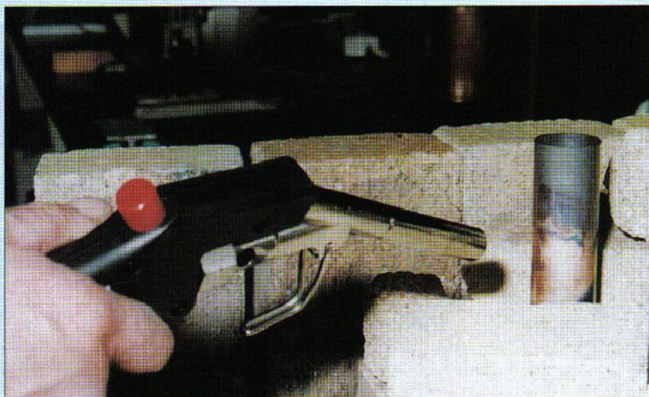
The Editor had the opportunity to try the new Autotorch Brazing System, loaned by Bullfinch. It was capable of silver soldering smaller boilers.
