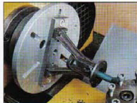
11. Machining the bore of the standard, again using the base plate. The top flange was also machined at this stage.
