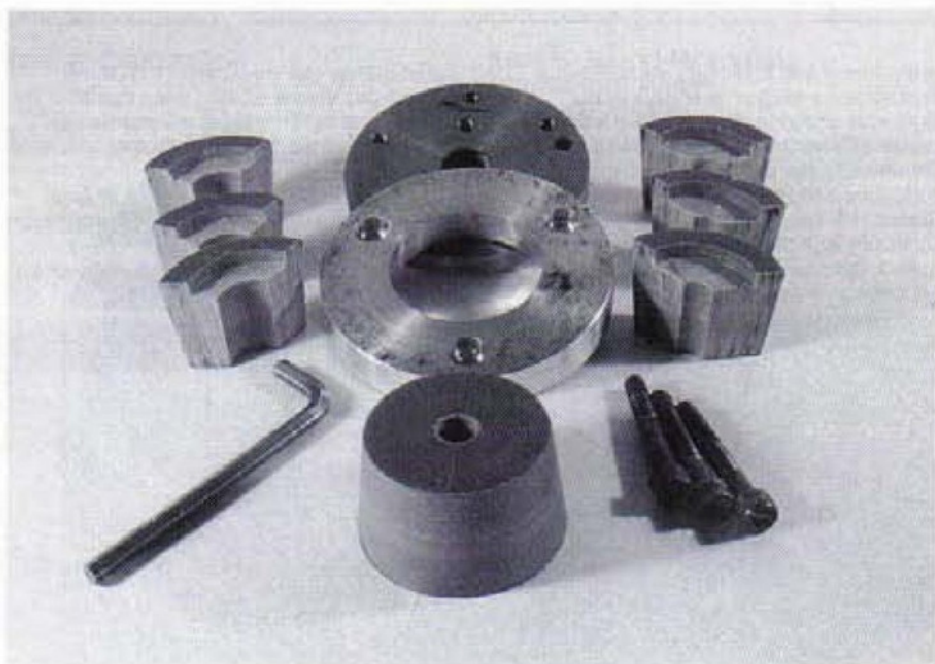
1. The component parts of the collet fixture. On the left hand side are the segments of the 0.75in. dia. collet, while those on the right are for the 0.50in. dia. version. In the foreground is a collet blank, ready for boring to size and then slitting when required
