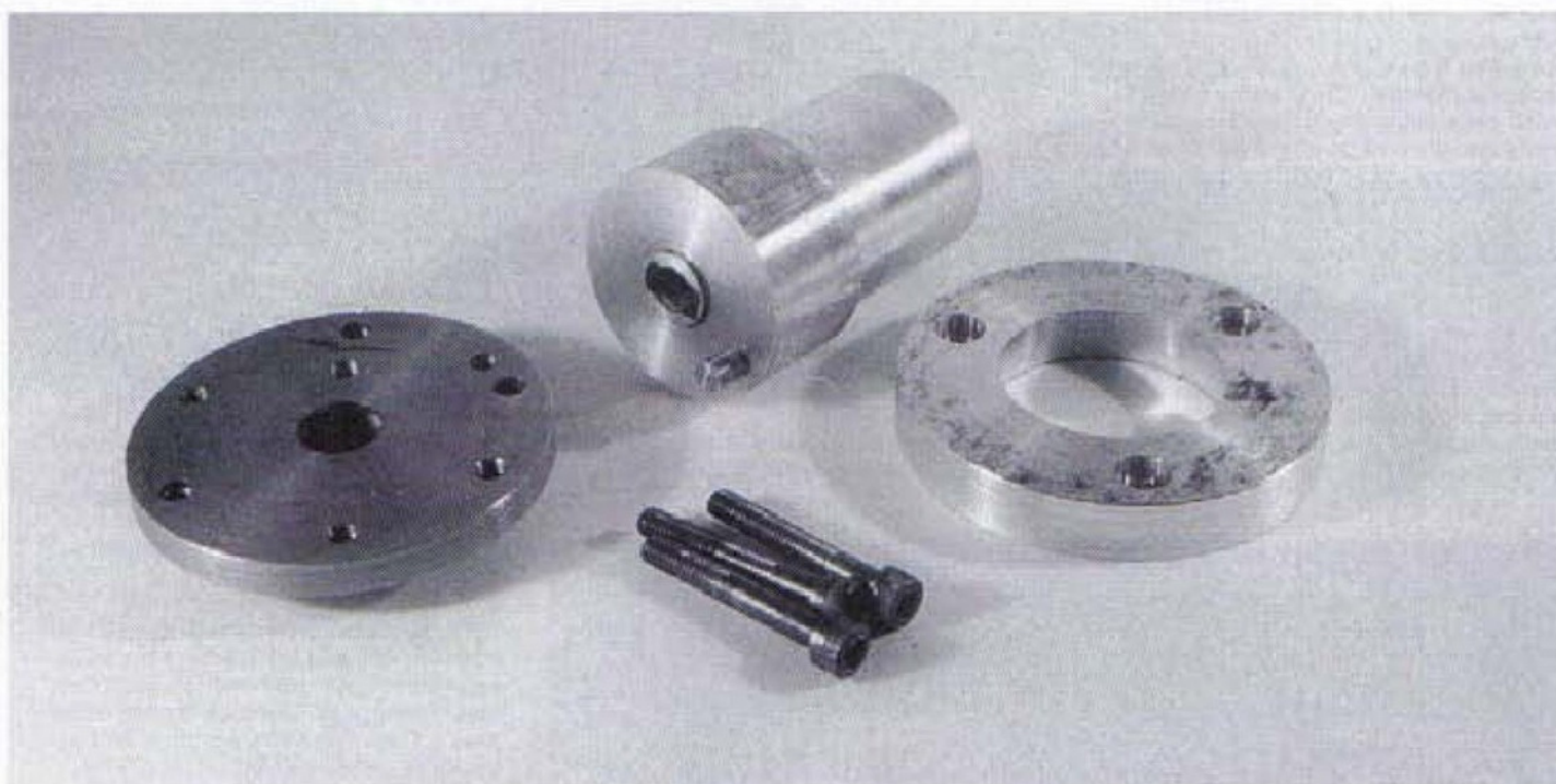
3. The component parts of Morse taper fixture. On the left hand side is the modified catch plate with its driving pin removed. In the centre is the Barrel which has a Morse taper bore. The tang slot can be seen with the locating spigot and driving dowel in position. On the right is the clamp ring
