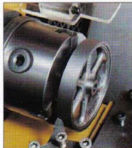
12. Set up for rough machining the flywheel outer diameter, sides and central boss.
