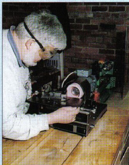
Mike Chrisp, Technical Editor of Model Engineer magazine demonstrates lathe tool sharpening on the latest version of the 'Worden' tool and cutter grinder, supplied by local firm Messrs Hemingway of Burstwick, Hull.
