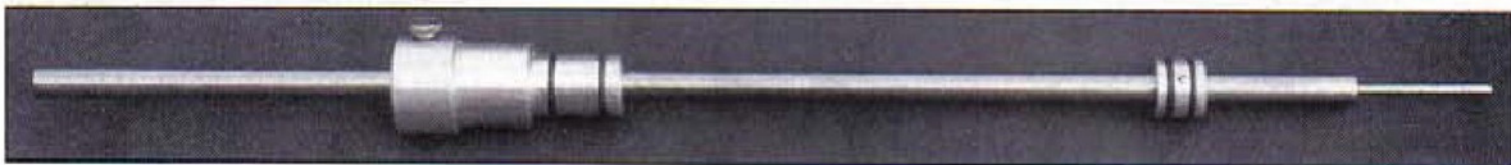
The completed depth stop, this one was made for a Myford Super 7 but there is no reason why the design should not be made applicable to any other lathe with a hollow mandrel.
