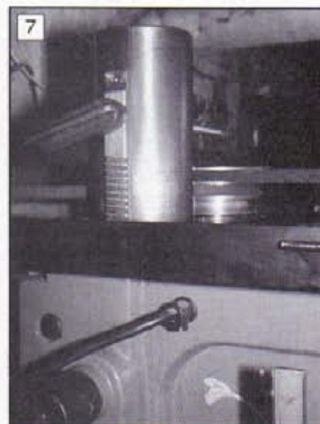
The upper end of the rack secured for drilling.
