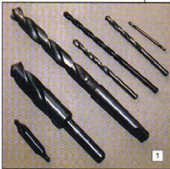
From bottom to top - Sloccombe centre drill; reduced shank drill; Morse shank drill; pilot point drill; long series drill; jobber's drill; panel drill.
