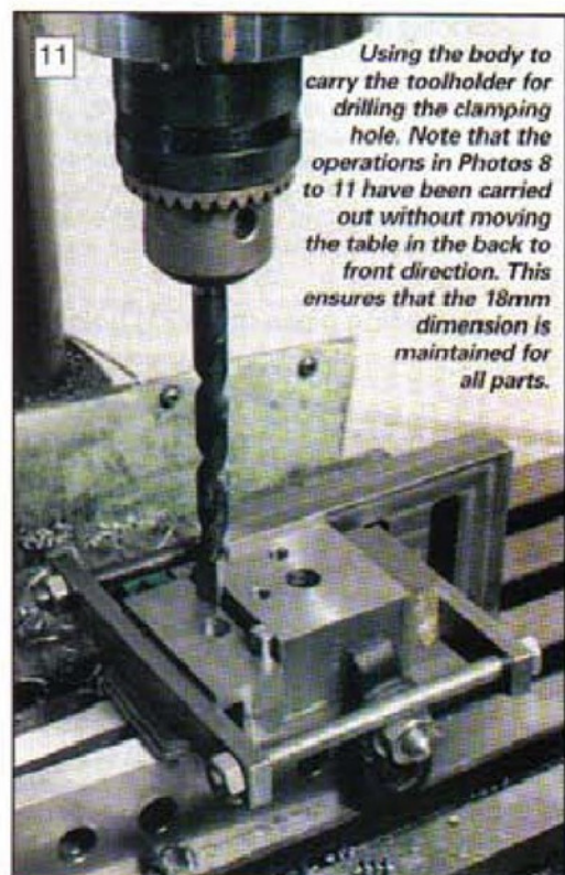
Drilling the body (ii)
