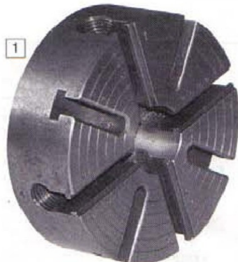
The chuck body, fully machined.
