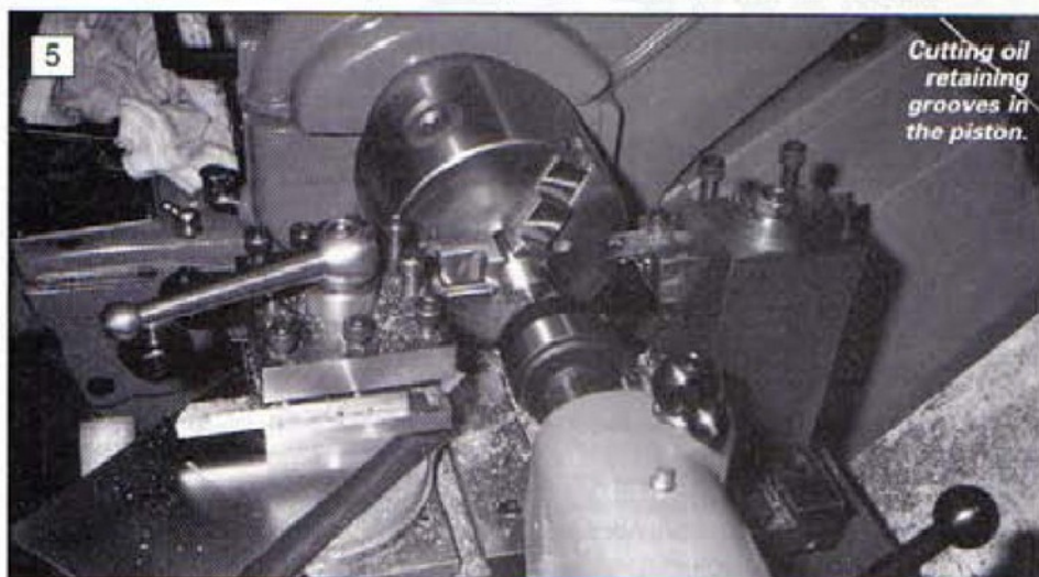
Screwcutting the barrel for the piston rod guide. Note the split bush in the chuck.
