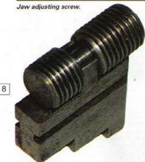
ABOVE Adjusting screw fitted to a jaw. BELOW: Jaw and screw started in body.
