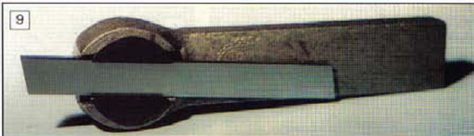
The clamping arrangement featured in this holder allows the blade to be pivoted to the desired top rake angle. The front clearance angle is adjusted accordingly. The toolholder was kindly loaned by L.A. Services, and the blade by Tracy Tools.
