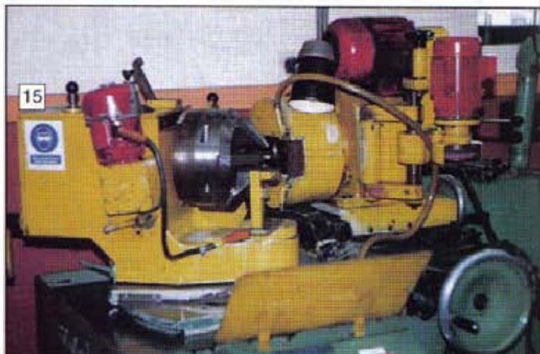
A drill grinding machine which features an almost fully guarded wheel.
