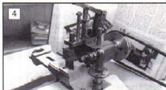
3: A simple pinion polishing machine built by John Lynam, demonstrating how equipment for clock making need not be complicated or expensive.
