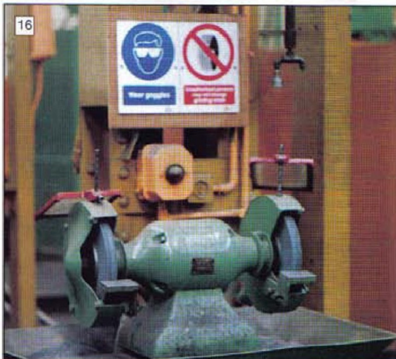
Warning signs displayed near a grinder in a factory. The right hand sign indicates that unauthorised persons may not mount wheels in this situation.
