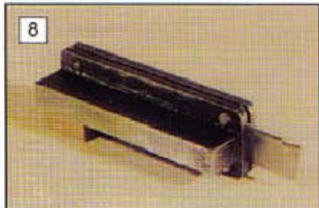
The tongue on the Mason holder can be clamped in a variety of toolposts.
