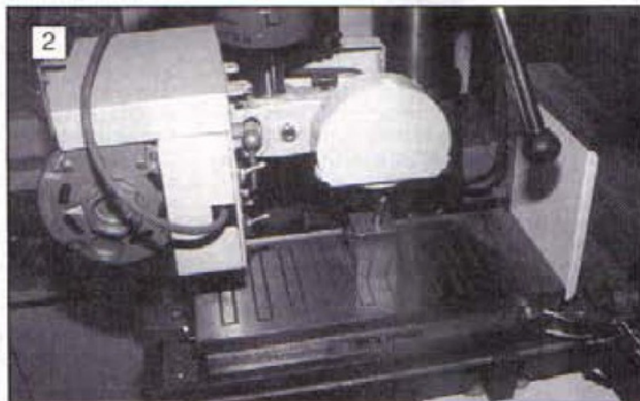
General view of set-up showing truing diamond, wheelguard and effluent shields.
