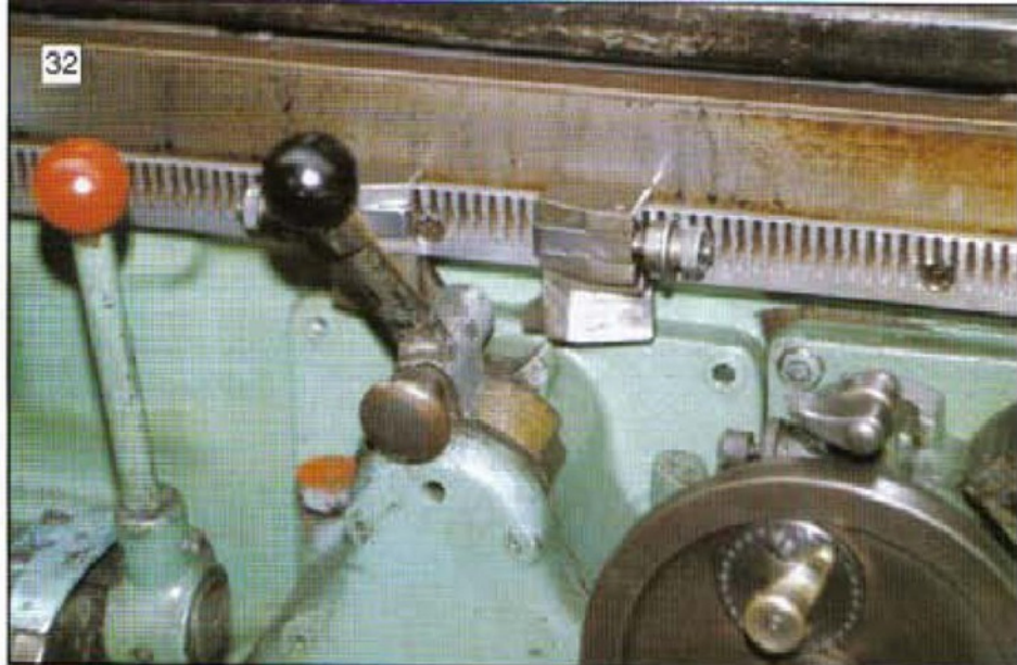
As well as moving on a rack, these stops have a fine adjustment screw
