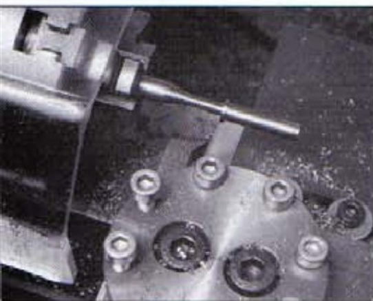
A good test of skill, turning a slender workpiece to a shoulder.
