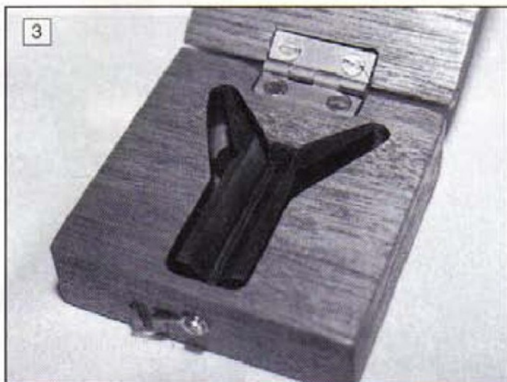
Mk. 1 Centring Device (Drill only). The Mk. 2 was similar, and would assist in the setting of saws.
