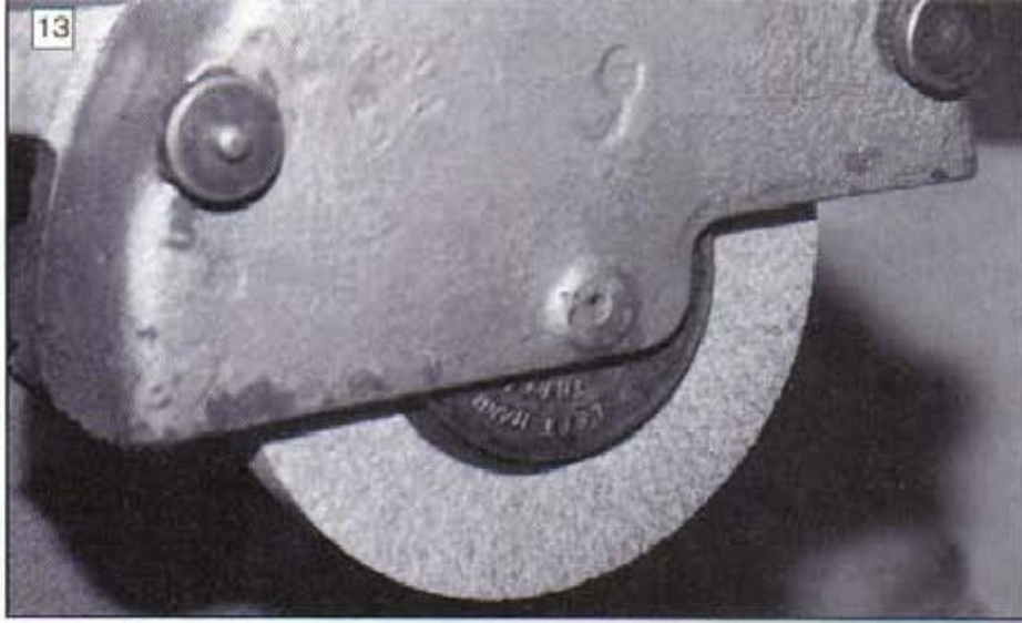
13 Wheel well guarded
