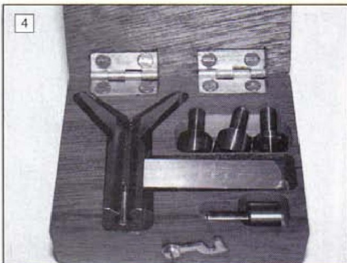
The Mk. 3 Centring Device, showing the accessories added to enable the setting of small end mills to be achieved.
