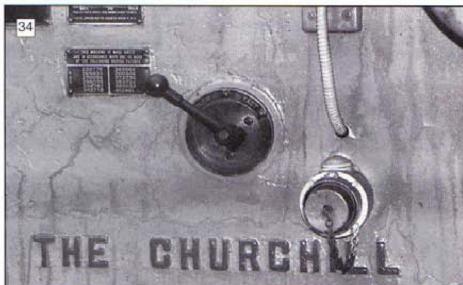
Workhead speed control lever on a Churchill grinder. This company was once the world's largest manufacturer of precision grinding machines.
