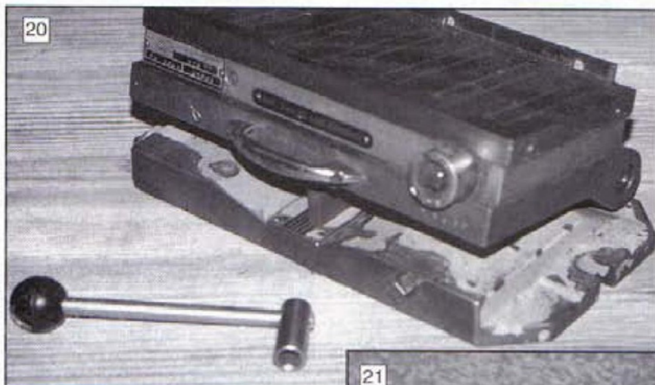
20 Magnetic sine table for grinding angles
