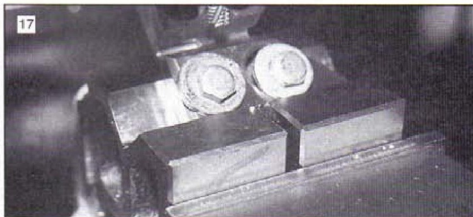
After drilling the central hole, the face 'V' is milled.
