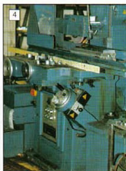
Sophisticated surface grinder with coolant/filter system.
