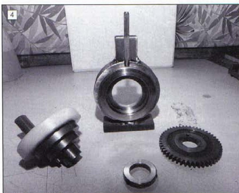
The cross slide handwheel stamping jig. Construction is self evident.
