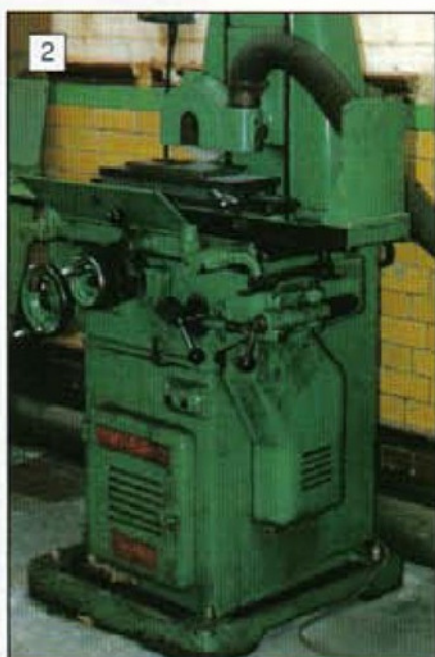
Small surface grinder with mechanical traverse. Note dust extraction.
