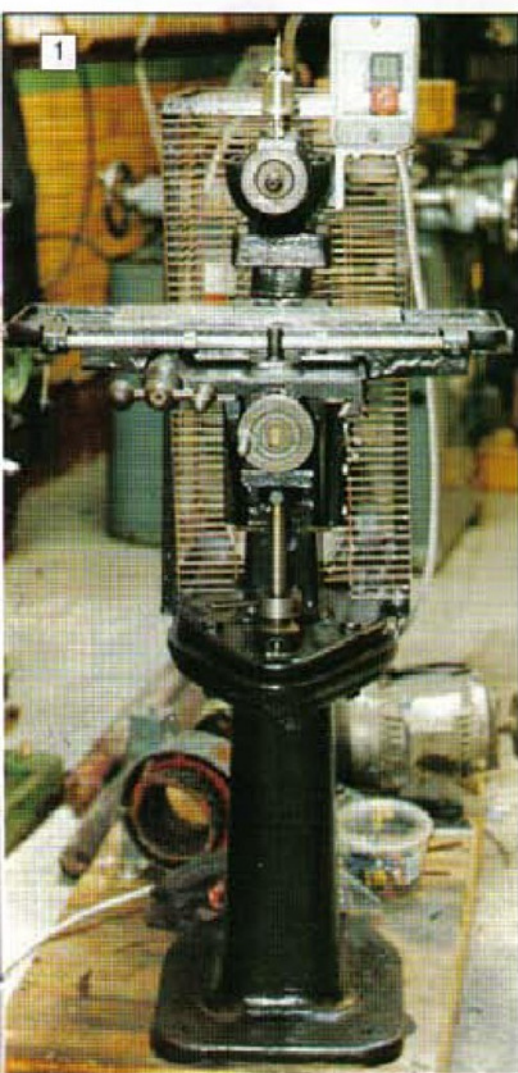
Basic surface grinder - very compact (hand traverse)
