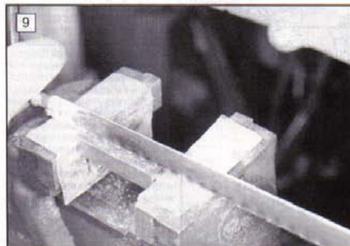
Splitting the jacket for the boring bar.
