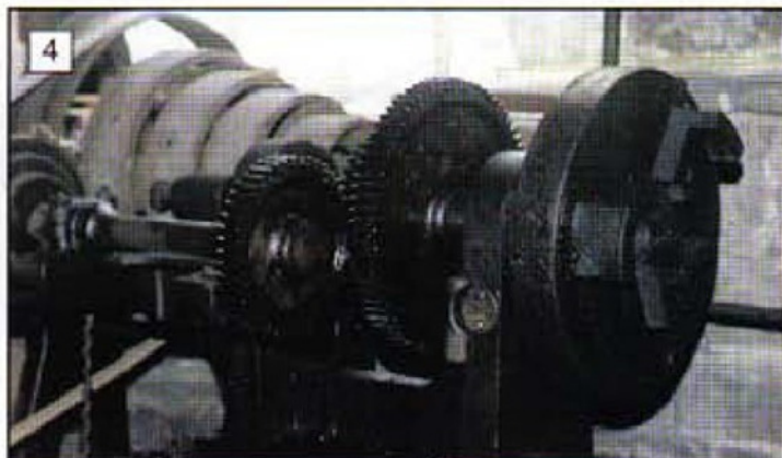
The headstock of this c.1820 lathe by James Fox of Derby is not very sturdy
