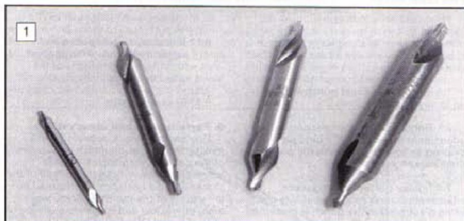
1 A range of centre drills, but two should be sufficient for the average workshop user
