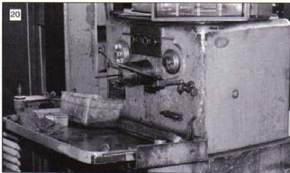
A honing machine for accuracy & finish on bores.
