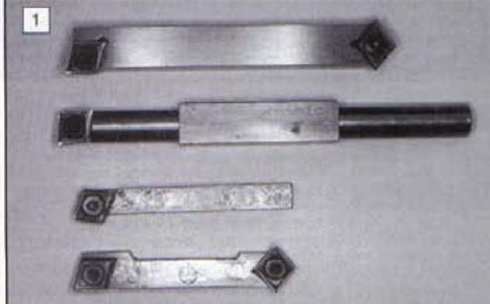
A set of home-made tipped cutters.
