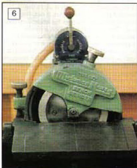
A diamond lap for fine finishing tool sharpening.
