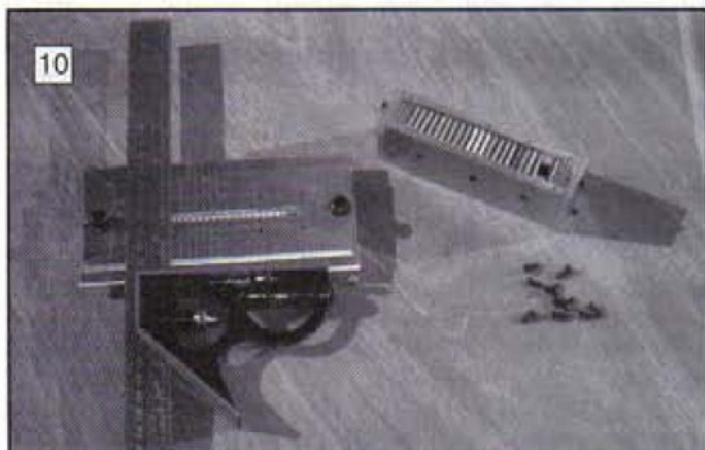
Transferring the inter-character scribe marks to the upper surface of the bottom plate. (Operation 8.3)
