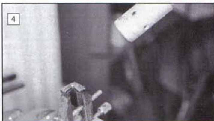
A finished insert being tinned for soldering.
