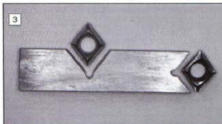
Two inserts filed to fit the tips, ready to separate and finish.
