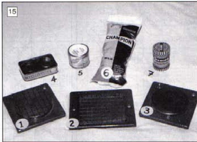
Small flat laps with lapping compound.
