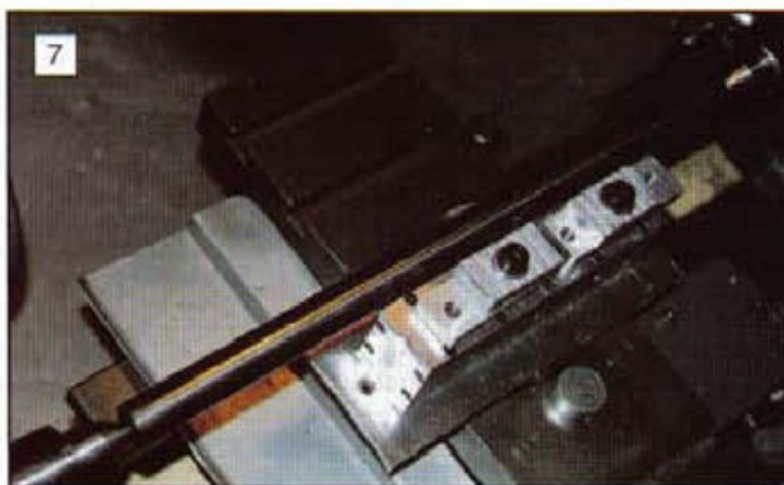
Setting the work parallel to the lathe axis using an accurately centred piece of PGMS bar. (Operation 4.21)
