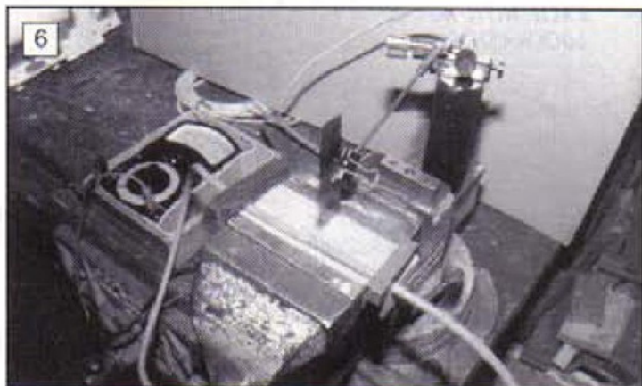
Belt joining jig, end cutting jig, thermocouple & butane torch.
