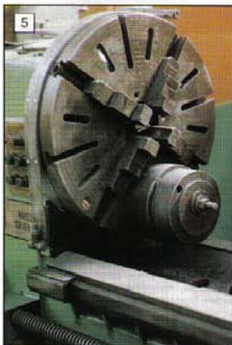
The chuck is counter-balanced to compensate for a top-heavy job, to achieve a better finish.
