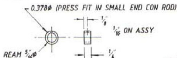
(11) SPACER, MAT L B.D.M.S. EN3B 1 OFF
