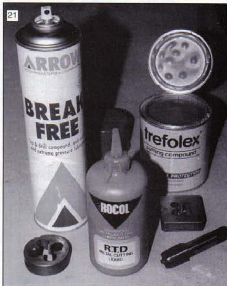
Cutting compound can enhance finish, especially when screw threading
