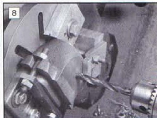
A set of faceplate dogs that permit total access to the front face, also precise positioning of the workpiece.
