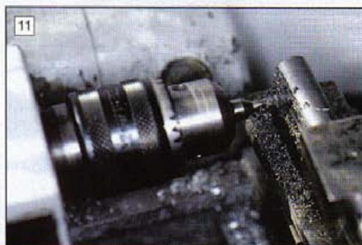
Milling the slot in the cutter holder body.
