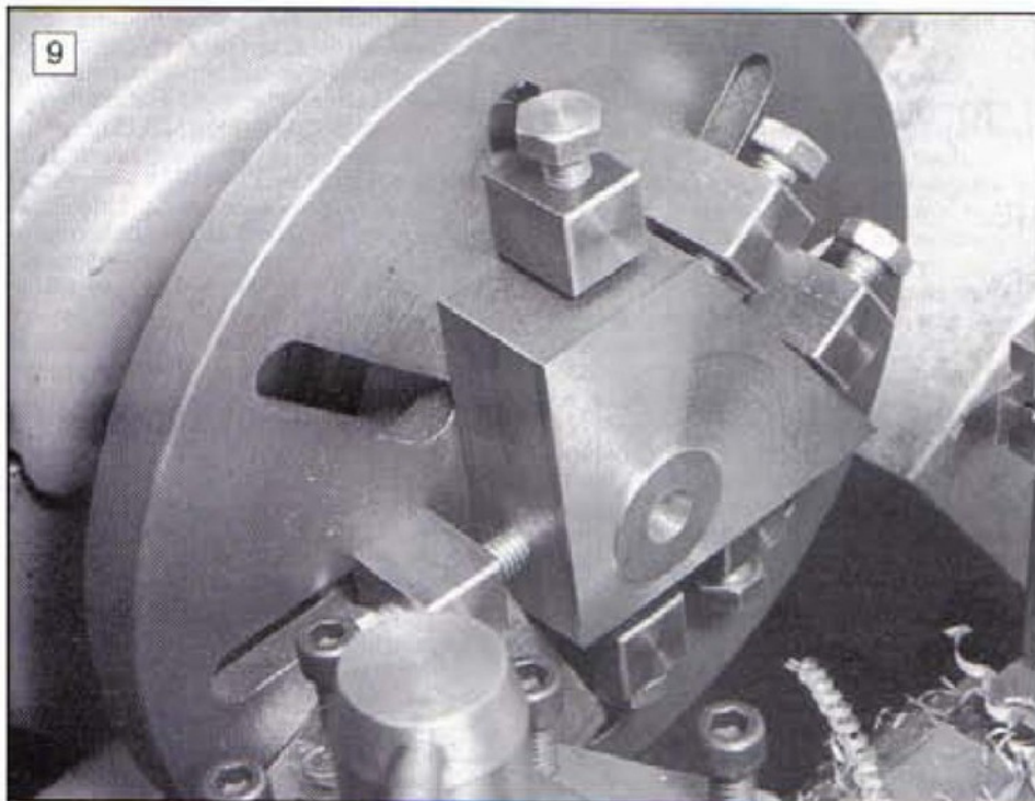
9 Secondary mounting arrangements are sometimes added to the faceplate, in this case a small angle plate.
