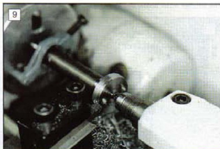
Turning the diameter of the spindle flange.
