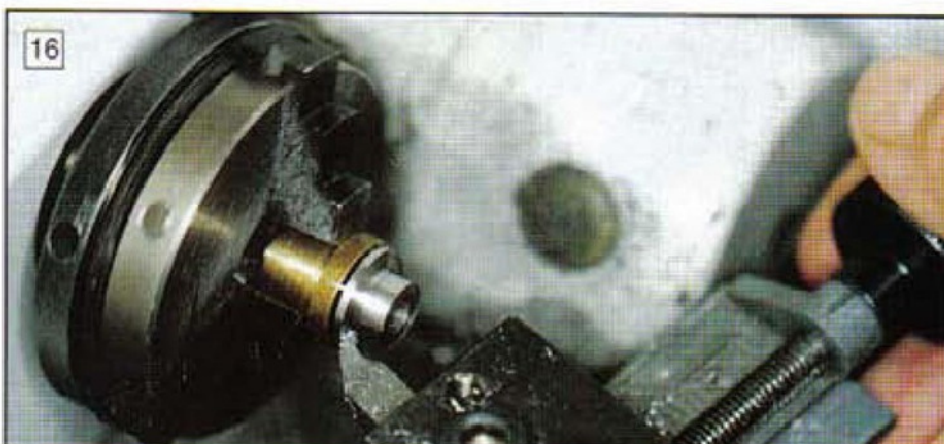
Machining the 20 deg. angle on the indexing dial; note the split bush and the cranked tool.
