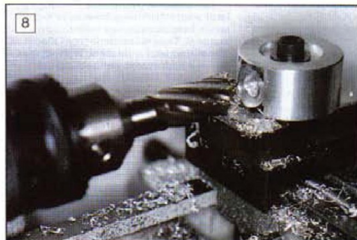
Using the large chuck to hold the 5/8in. end mill for counterboring.
