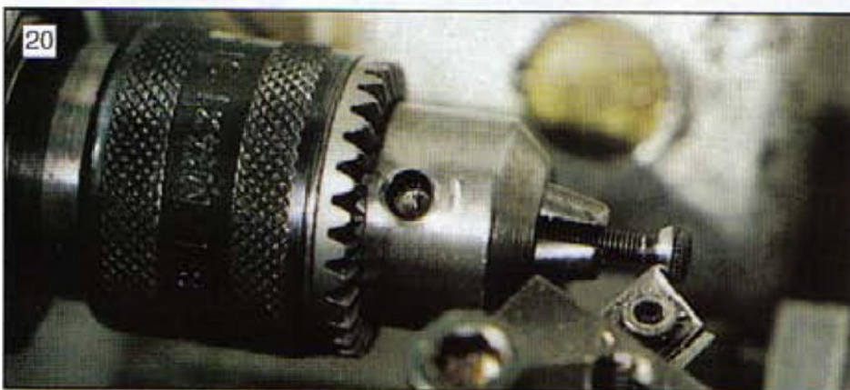
Turning the 60 deg. angle on the tip fastening screw.
