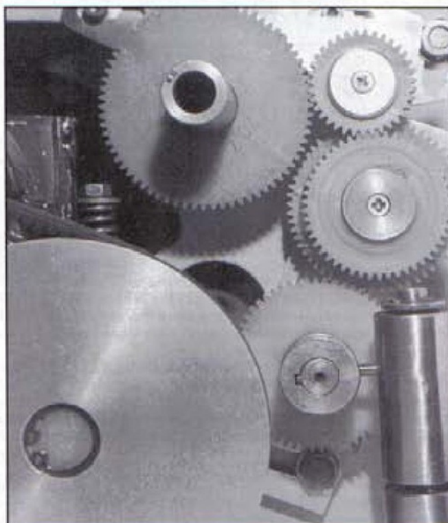
The 'Mk. 1' device set up to cut LH 20 TPI thread.
