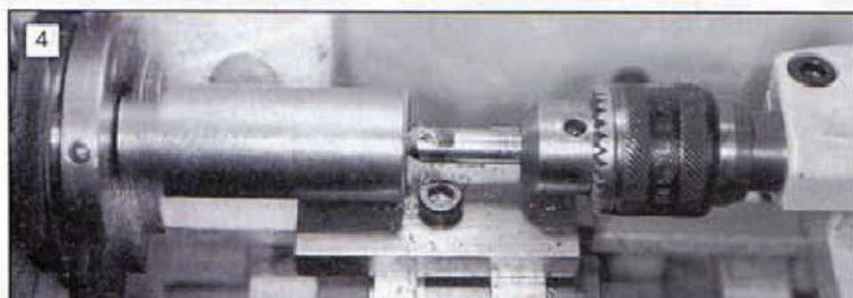
An emergency method of centring a bar which won't pass down the spindle.
