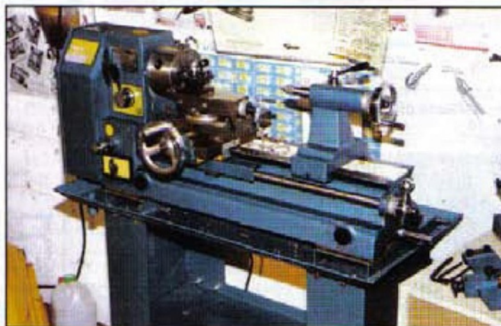
The 'Nu-Tool' lathe with some of its accessories. The combined lathe/mill version can be seen in Photo. 1.
