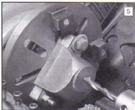
Mounting a large casting on the faceplate. Note the fixings are well spaced for secure mounting.
