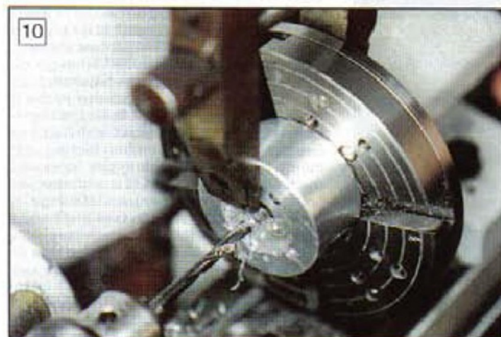
The method of drilling the holes in the head. The work must be clamped.
