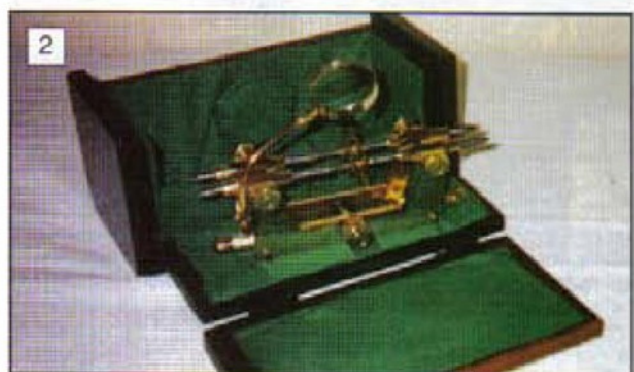
2. Based on a design published in M.E.W. No.8, this clock wheel depth tool is by Anthony Pedley of Totnes, Devon
