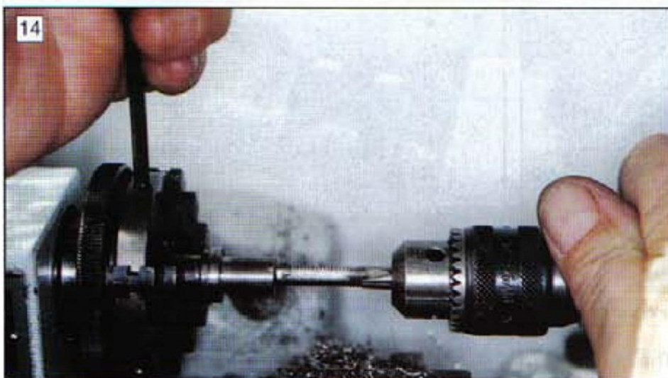
Starting the tap in the indexing dial. The lathe is turned off at the mains.
