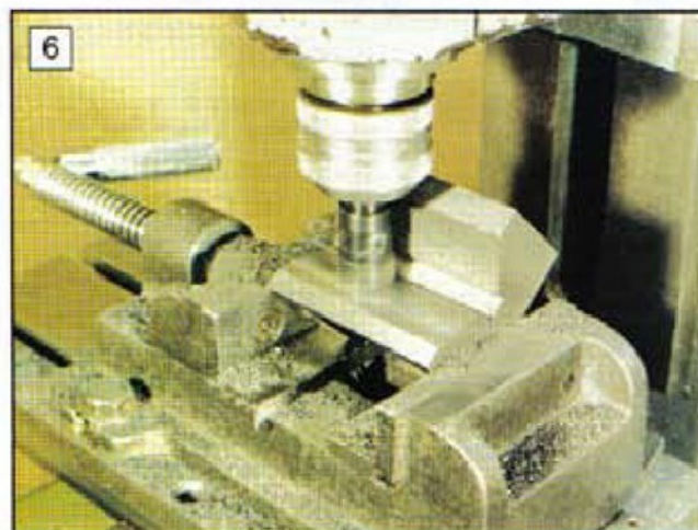
Machining the first 'Vee' face, using a single inserted tooth cutter in the milling machine.
