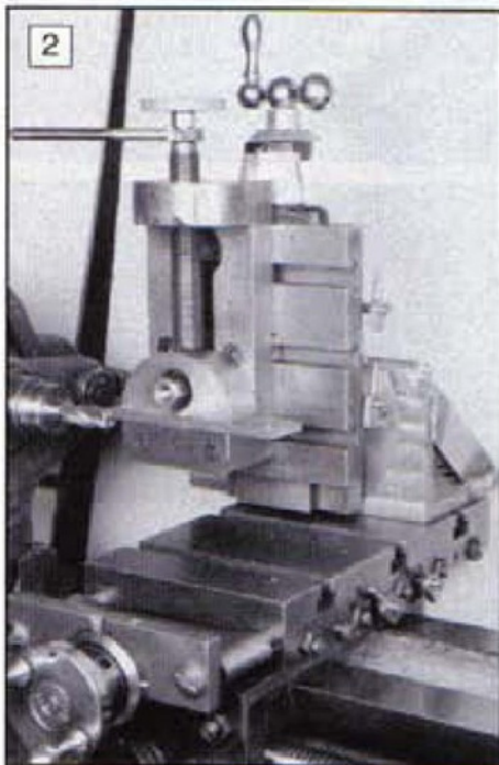
Counter-balanced clamps are featured on both the cross-slide and the vertical slide, while the machine vice has a long arm version for its leadscrew
