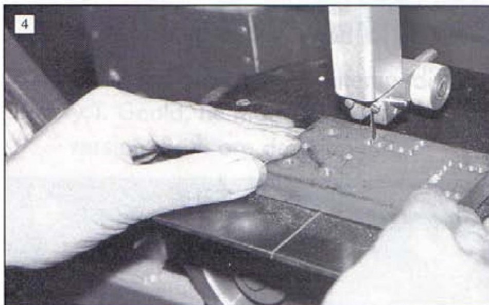
After chain drilling, the cut-outs in the outer end plates were formed on the band saw
