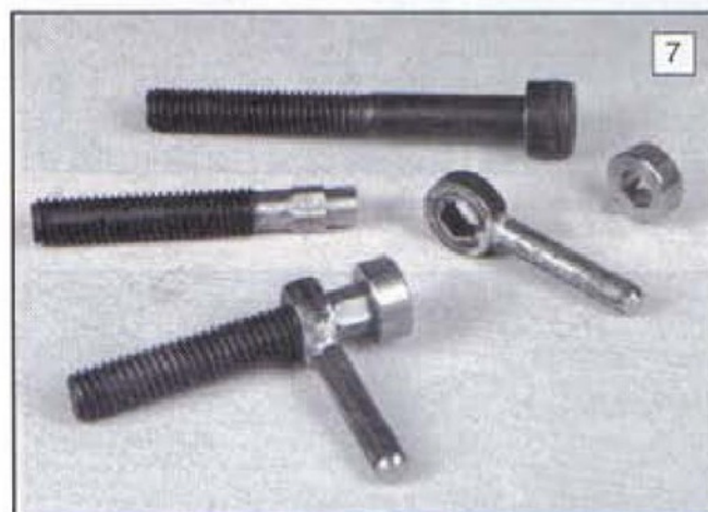
Locking arms for the ML7 cross-slide, shown with the type of plain shank cap head screw from which they were derived
