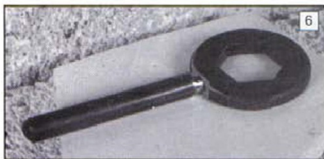
Preparing to butt braze a locking arm
