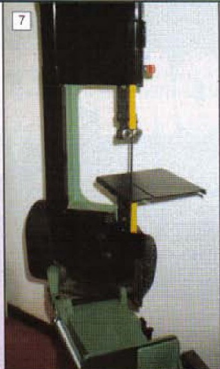
J. Vickers' saw, showing the long length of unguarded blade
