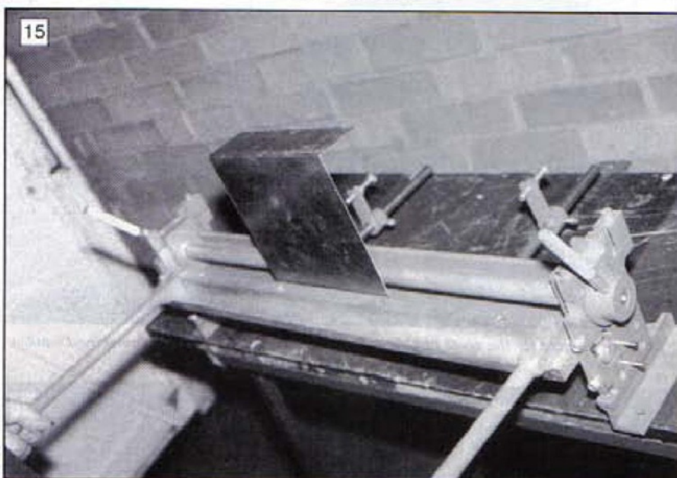
These show the second folding beam, with the 20mm square stiffener. Photo 15 depicts a fold in 18 swg mild steel, while Photo 16 illustrates folding a reverse flange
