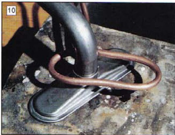
10 Brazing an oil strainer head on to the suction tube of a large diesel engine. The induction coil is large enough to allow the strainer to be removed after brazing. In Photo 10, no flux has been added so that the braze ring can be seen, but flux was applied prior to heating.
