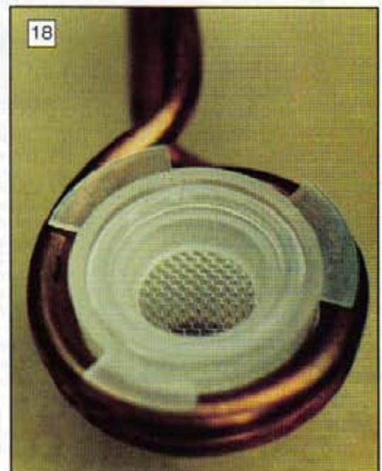
Plastic to metal bonding. In this instance, the stainless steel mesh is heated to a temperature high enough to melt the plastic component parts in contact on either side of the mesh, which then bond securely together on cooling. The assembly is an oxygen mouthpiece for the emergency oxygen supply in passenger aircraft.
