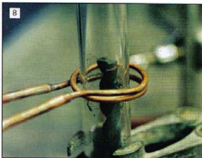
8 Brazing a polycrystalline diamond tip on to a tungsten carbide drill shank. An inert atmosphere is used, hence the glass tube.
