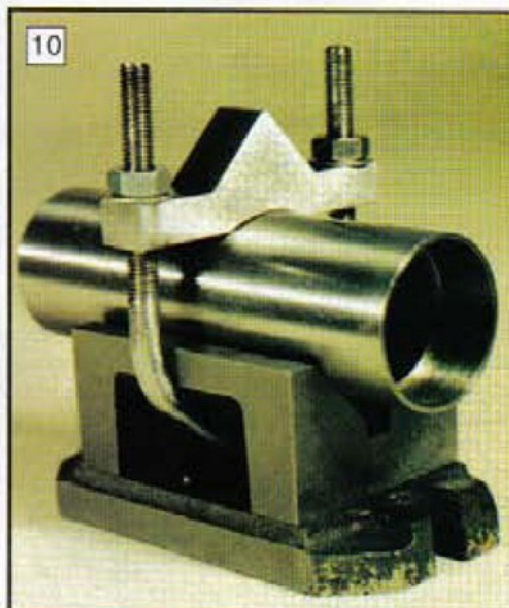
In the alternative configuration, the device becomes a conventional Vee block.
