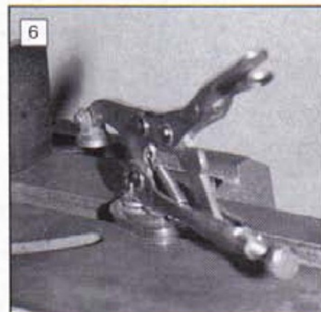
A proprietary clamp of the type used on drilling machine tables will help to secure some jobs
