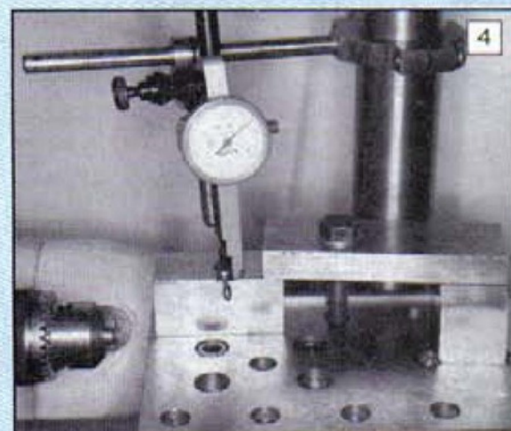
A small dial test indicator is a useful setting up aid.
