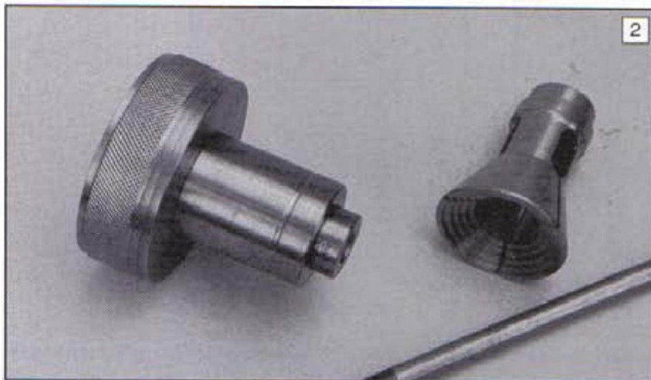
Thin piece collet for use with system in Photo 1. Maximum diameter 30mm, each step 1mm deep.
