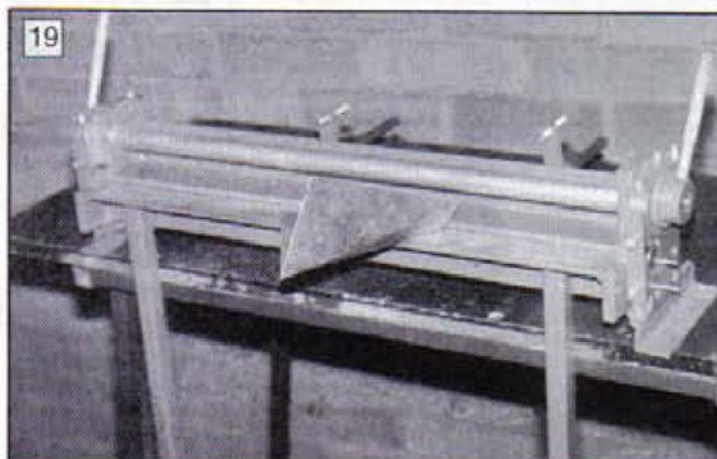
Folding all-round flanges. a 12mm packing piece (seen under the clamping beam) is required
