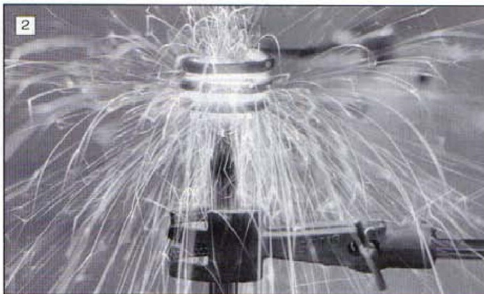
The end of an ejector pin taken to a temperature beyond melting point simply as a demonstration.
