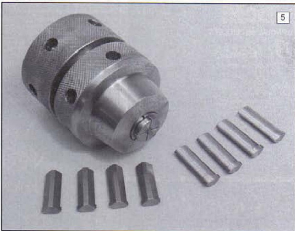
Collet adaptors to enable a standard collet to be used with square or hexagonal material.
