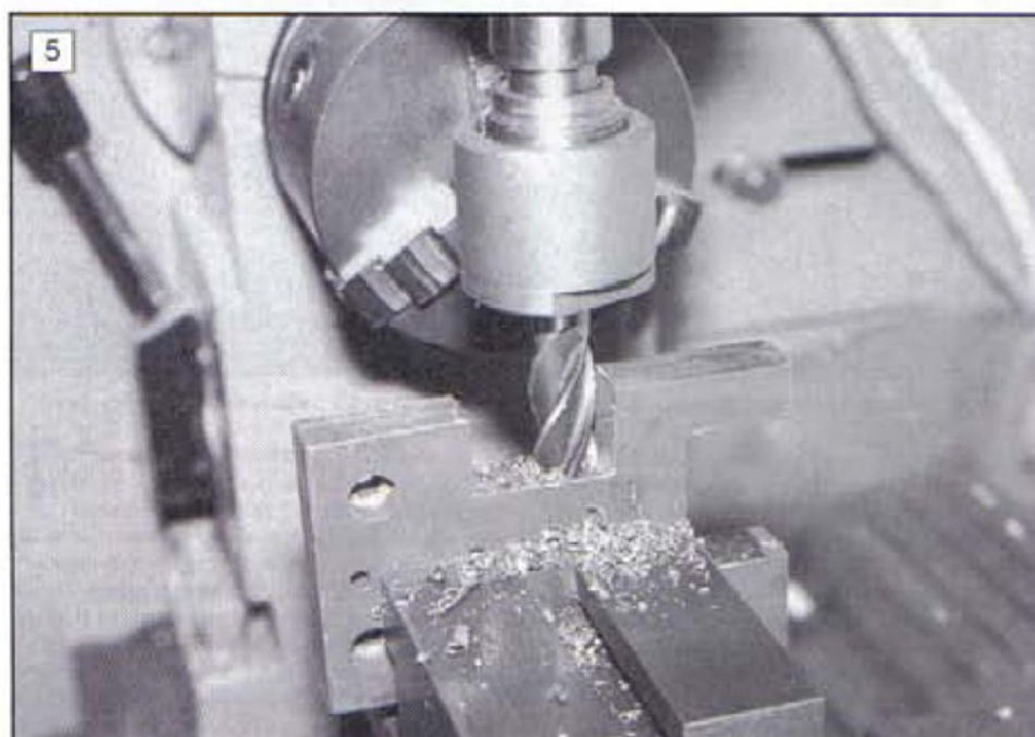
Milling the cut-outs in the outer end plates
