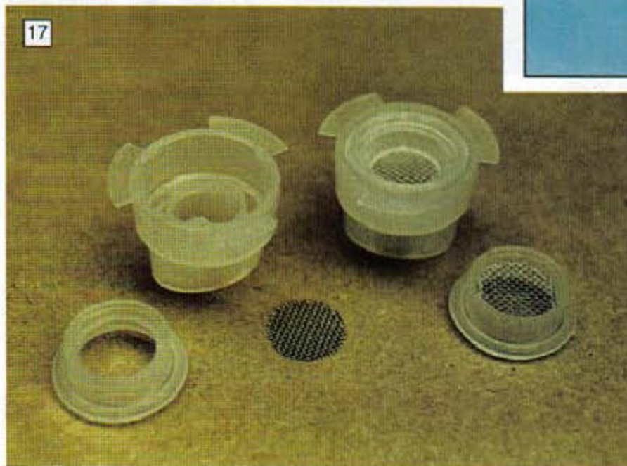
Plastic to metal bonding. In this instance, the stainless steel mesh is heated to a temperature high enough to melt the plastic component parts in contact on either side of the mesh, which then bond securely together on cooling. The assembly is an oxygen mouthpiece for the emergency oxygen supply in passenger aircraft.
