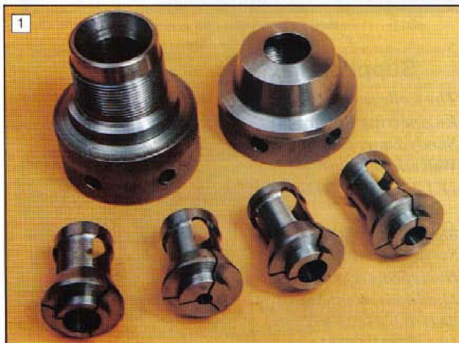
Simple home made collet system. Maximum diameter 16mm.
