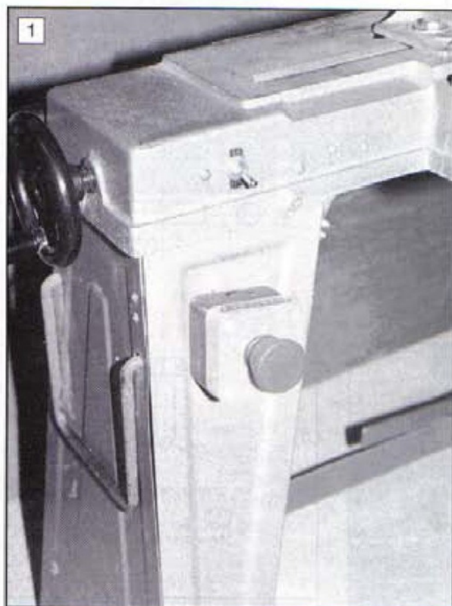
1 A 'No-Volt Release' switch provides additional safety when both hands are occupied
