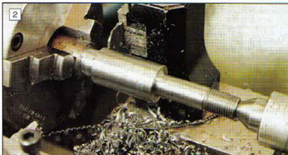
The tailstock centre being used to support the outer end of a workpiece held in the three jaw chuck. All diameters and thread were machined while in this set-up, thus ensuring concentricity of the important surfaces.
