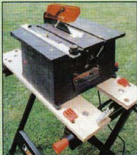
This Dremel circular saw has a 4in. blade and its ability to cut accurately makes it a favourite tool, but alas, it is no longer marketed.
