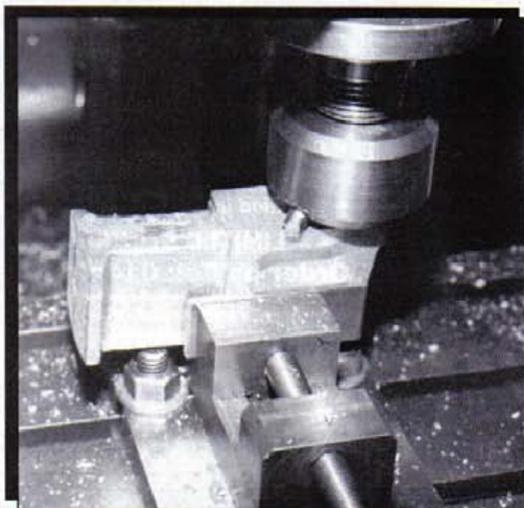
Facilitating an awkward task, one of the many applications for Alan Jeeves' light toggle press is for keyway cutting. Full constructional details of this useful item of workshop equipment begin on page 22.
