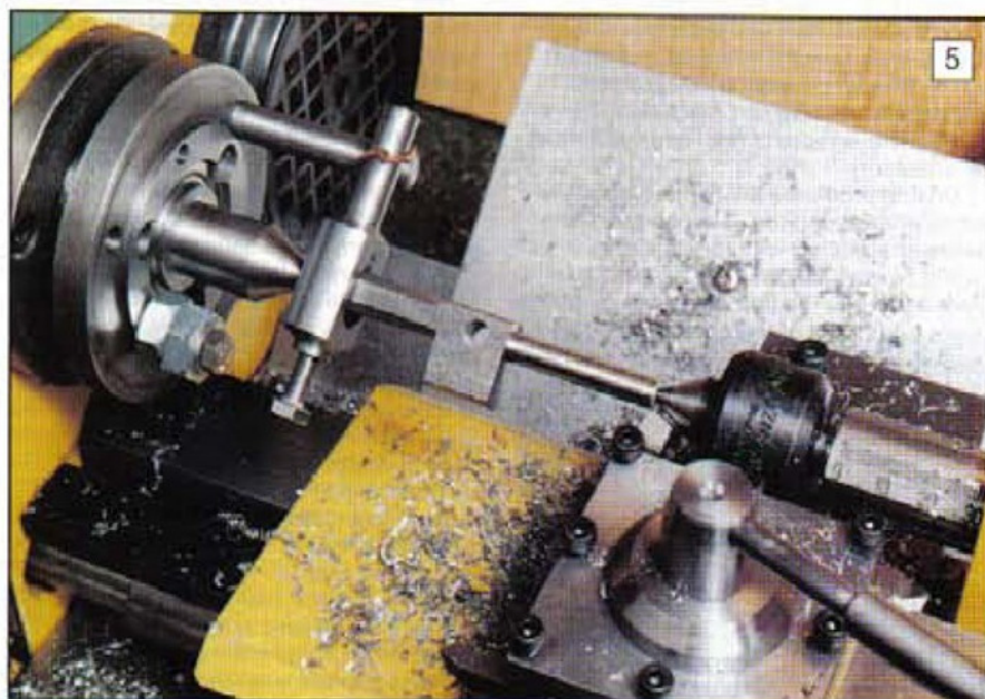
The initial stages of turning a small crankshaft. An excellent example of an item for turning between centres.
