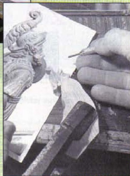
Carving the pattern for Warrior's figurehead, using a photograph of the full-size version as a guide.
