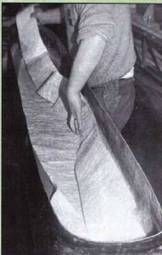
Re-inforcement of the hull in process.
