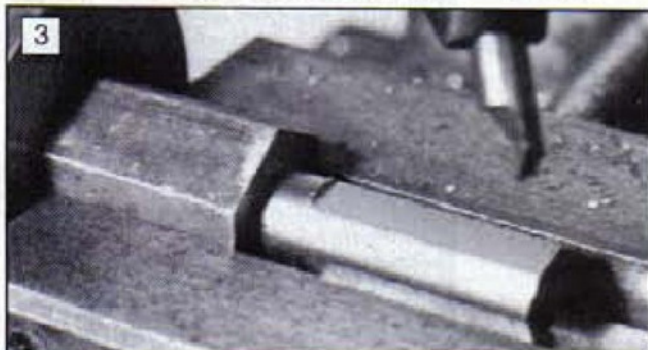
The three Drive Flats being Milled - Note method of Indexing
