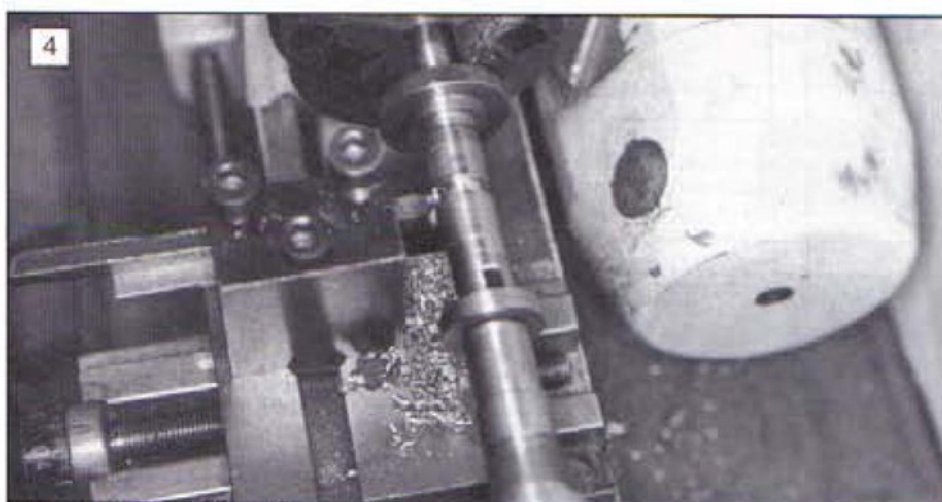
Undercutting the drive shaft.
