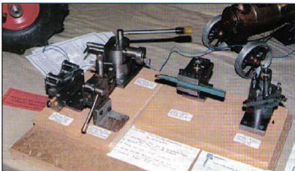
Tooling for the older lathe need not be a problem. All these tools, roller filing rest, scissor type knurling tool, Lammas three way toolholder, swing clear boring toolholder and engraving tools for protractor and circular scales were made for an elderly Drummond lathe. Builder is R. Spilman of Worthing DSME.
