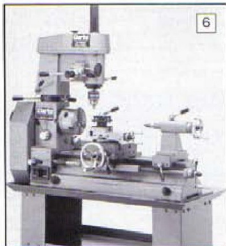
6: This example of a combined lathe/drilling and vertical milling machine is available from Machine Mart. Several other suppliers offer a similar machine, it is worth shopping around for a bargain. Advantages are a huge swing over the bed, and a lot of machine packed into a small area.
