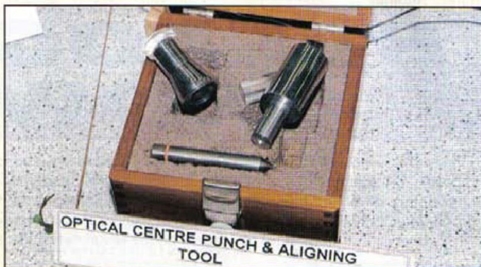
This design dates back to MEW No. 1. The optical centre punch and aligning tool, in a fitted box were made by a member of Chichester SME.
