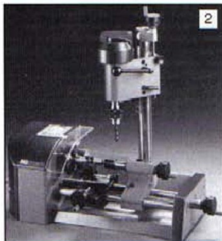
2: This Unimat machining centre, which combines the function of lathe, drilling machine and vertical milling facility in one small machine. Has electronic speed control to the motors as a built-in feature.
