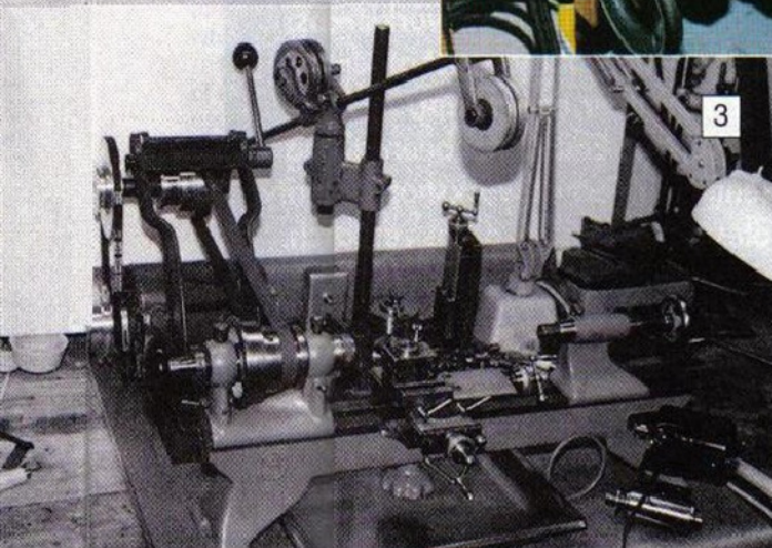
5: Spoilt for choice! A close-up of the G.H. Thomas designed small rotary table mounted on the Aceria F1 milling machine.
