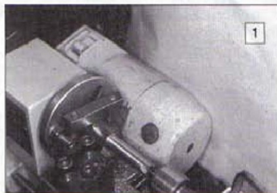
1: One end of the arbor being turned using an improvised carrier to drive the work.
