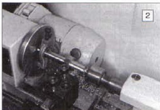
2: The other end of the arbor, with a conventional carrier.
