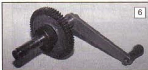
6: The completed handle, seen here with the gear used for dividing attached.
