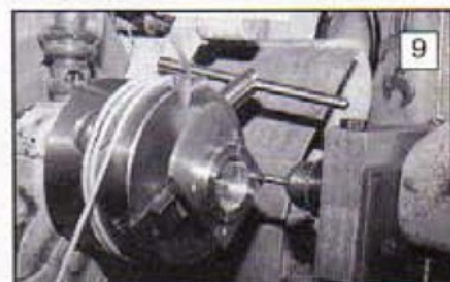
9: Drilling four holes in exact positions on a pitch circle diameter, using the bracket and electric pistol drill. The string around the chuck supports a heavy weight, thus effectively removing any backlash from the set-up.
