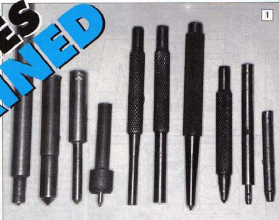
1: Selection of the author's punches, from left to right, spotting or transfer, riveting, special transfer (long reach), case-hardened for seed box holes, 2 pin, 2 centre, 2 hand bag.
