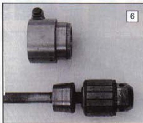
5: Angle of drill set by adjusting screws for cutting worm wheel tooth angle 6: Nose bearing and spindle for the Tauco drill.
