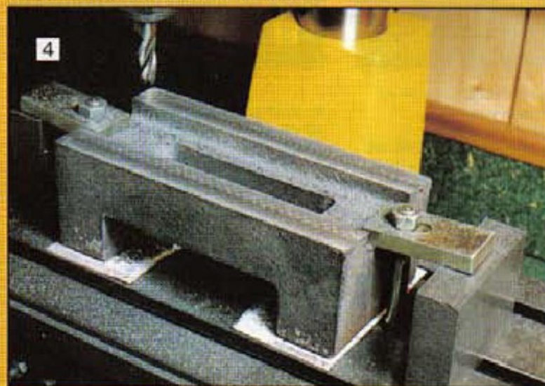
3: The jaw keep plate arrangement.
