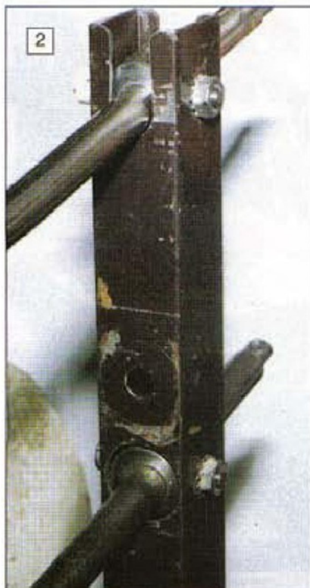
2: Showing how the arms fit on the frame. The pivot collars can be clearly seen.
