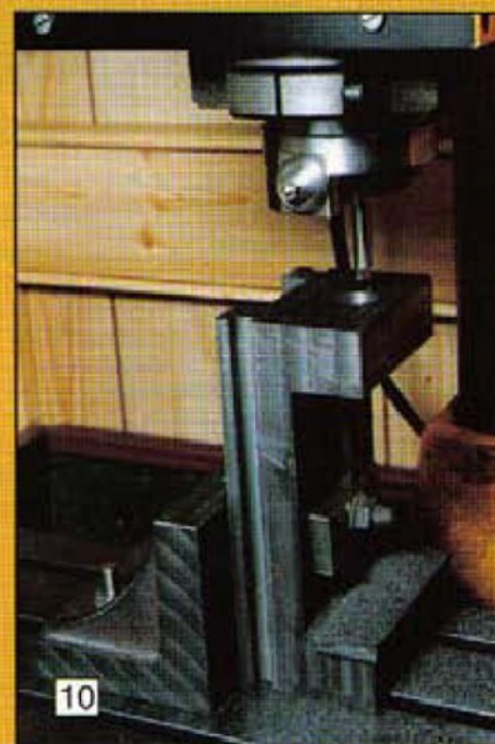
11: Finishing the jaw plates, including the mating faces.
