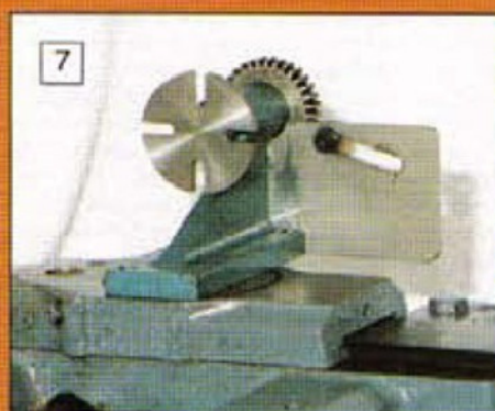
5: Assembled attachment with 36T change wheel in place.
