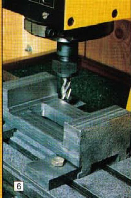
6: Machining the inside of the fixed jaw and the jaw sliding surfaces.
