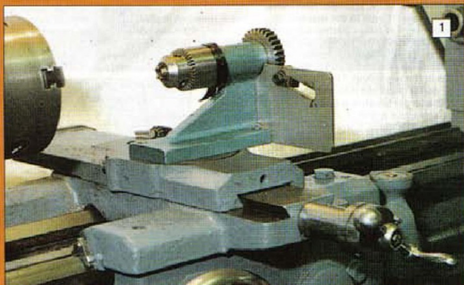
1: Completed attachment set up in the lathe parallel to centre line.
