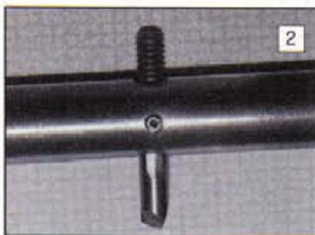
2: A boring bar, the tool bit is made from a section of a broken slot drill.
