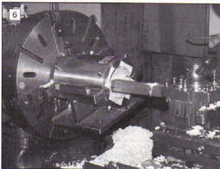
6: A complex stainless steel fabrication - a split bearing for the shaft of a mixer. This is lined with Teflon.
