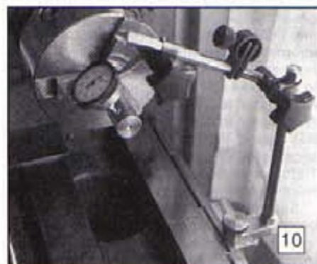
9: Angular scale and graduated collar. Note the swinging arm clamping screw installed in the right hand screw in the retainer bar. 10: Another use for the additional slideway - a permanent mounting for a DTI holder.
