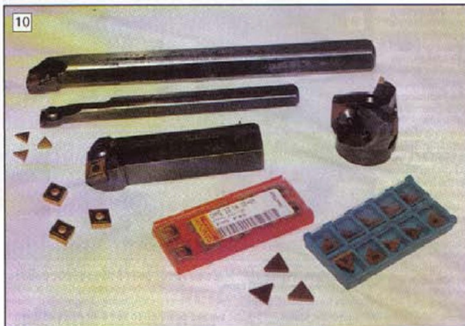
10: 'Throw away tip' lathe tools and 50 mm dia. milling cutter. Go for grade 235 for stainless (all the tips seen here would cost the best part of £100 today)
