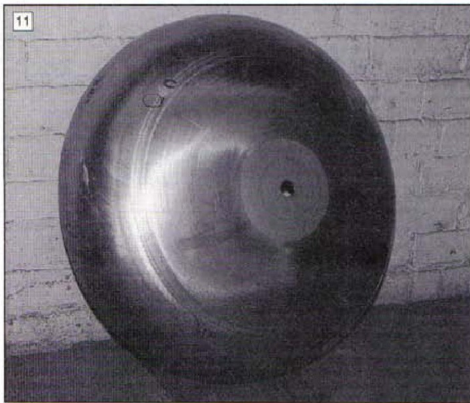
11: A dish which has been spun from 6mm stainless steel plate and is 80cm diameter. The 25mm hole in the centre is used for the spinning centre. It is eventually closed by means of a welded in plug.
