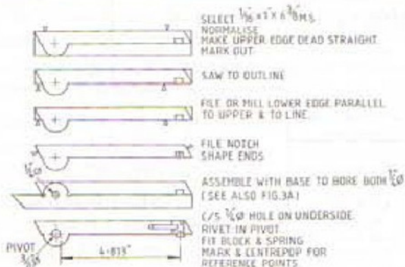
FIG. 4A SEQUENCE FOR MACHINING ARM
