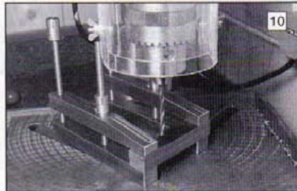
Showing one of the potential uses for this form of toolmakers clamp, that would not be possible with the traditional design of clamp.
