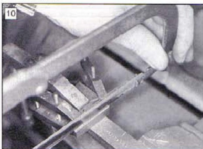
10: Sawing one of the quadrant steps using a fence again, note the bar clamped in the vice for clamping the work. The stamped numerals are where the number stamps were tested. This is the size used to identify positions for the quadrants.
