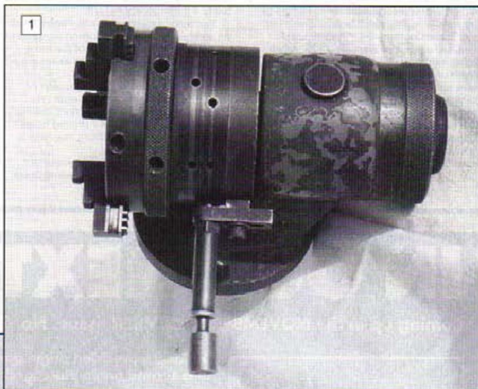
1: General view of indexing device. The calibrations can just be seen on the end cap at the right hand end.
