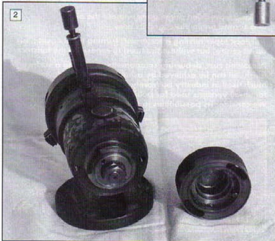
1: General view of indexing device. The calibrations can just be seen on the end cap at the right hand end.
