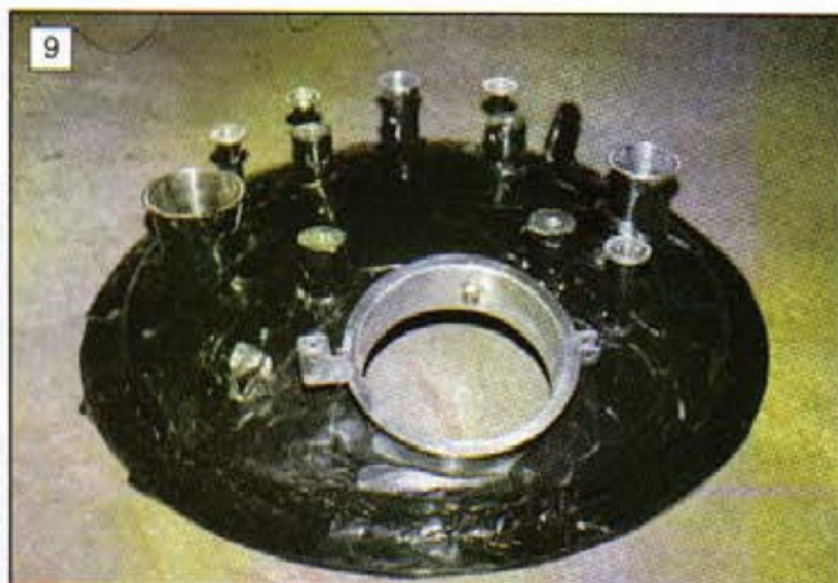
9: A stainless product should always be protected after polishing. This one is covered with PVC tape.
